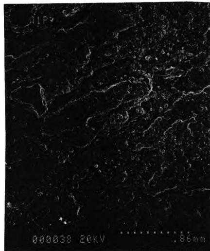
**Figure 5.19b: Fracture surface for specimen W1/W5 (cracks > 4 mm)**
