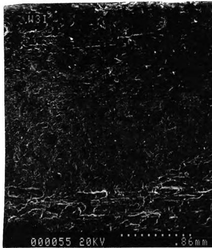
**Figure 4.15a: Shallow crack surface ( $a < 4$  mm), Specimen W6**
