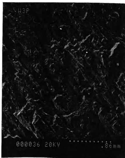
**Figure 4.15b: Deep crack surface ( $a > 4$  mm), Specimen W6**
