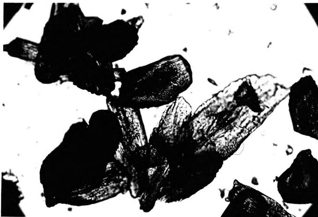
Figure 3.48 Optical micrograph of scale from non-MTW [ x100 ].
