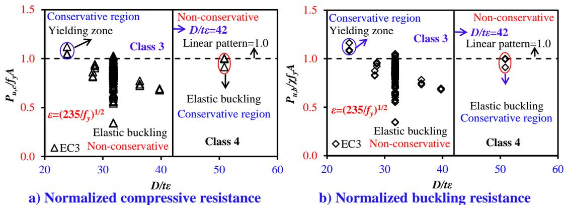
894 **Fig. 34** Normalized resistances of shear-keyed grouped tubes
