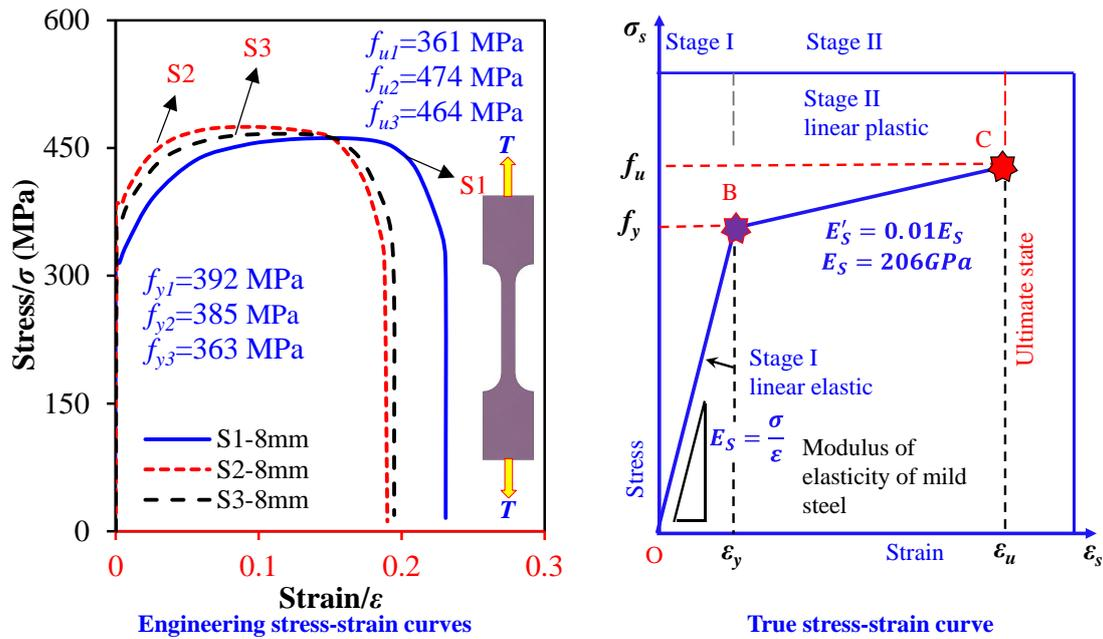
(c) Test stress-strain curves and FE material model
