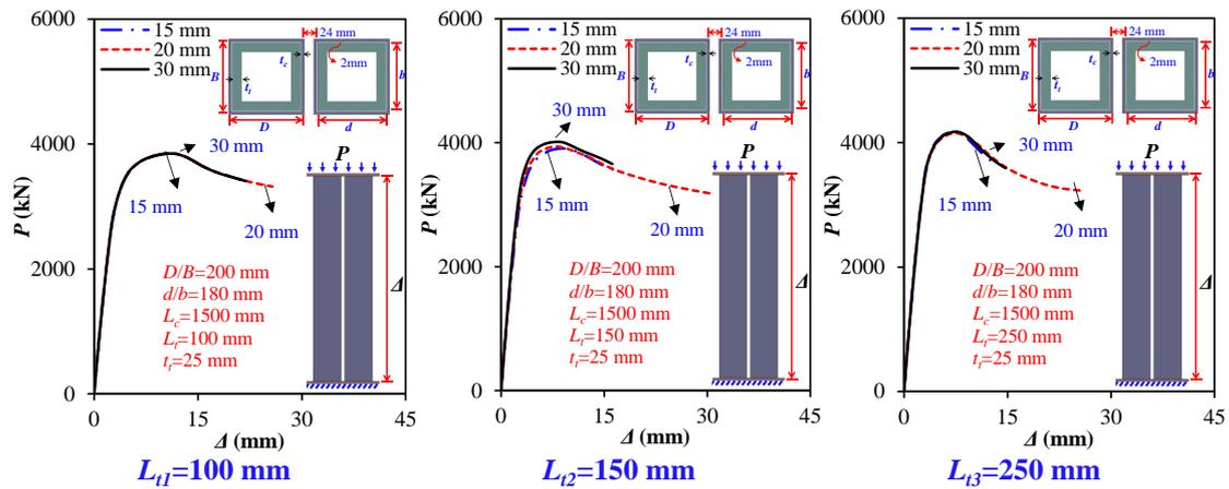
**Fig. 33** Influence of friction and connecting plate
