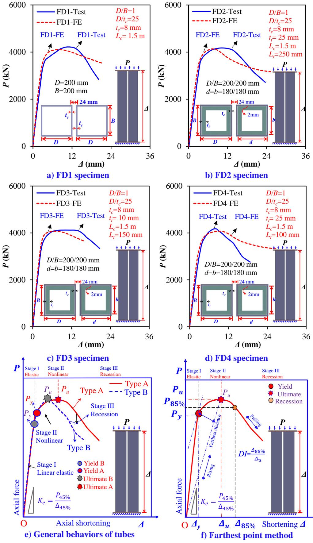
**Fig. 8** Axial shortening curves of shear-keyed grouped tubes
