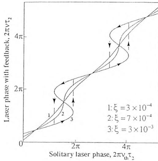
Fig. 2. Theoretical variation of frequency for a laser diode with feedback,  $\nu$ , with solitary laser frequency,  $\nu_0$ , for three values of feedback coupling coefficient,  $\xi$ , with external cavity length,  $L_{ext} = 200\text{mm}$ . Frequencies expressed in terms of external cavity phase.
