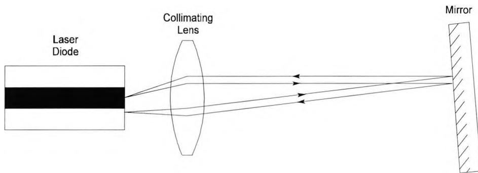
Fig. 6.5. Path taken by a single ray in an external cavity with a tilted reflector.
