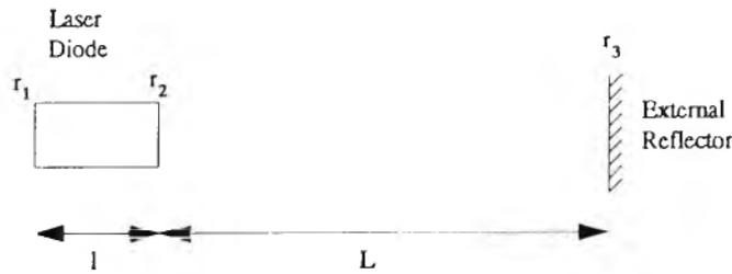
Fig. 1 Schematic representation of a laser diode with an external reflector.
