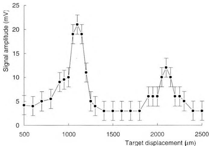
Fig. 4.1. Self-mixing interference fringe amplitude measured against longitudinal target displacement with a multimode laser diode.
