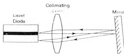
Fig. 4. Path taken by a single ray in an external cavity with a tilted reflector.
