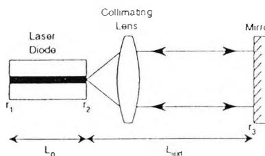
Fig. 1. Schematic representation of a laser diode self-mixing interference system.
