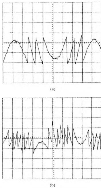
Fig. 6 Oscilloscope traces showing output intensity of a laser diode with feedback with the external cavity length modulated using a loudspeaker mounted mirror (a) Normal intensity modulation frequency. (b) Double intensity modulation frequency. (Horizontal scale: 2 ms/div, vertical scale 2 mV/div)
