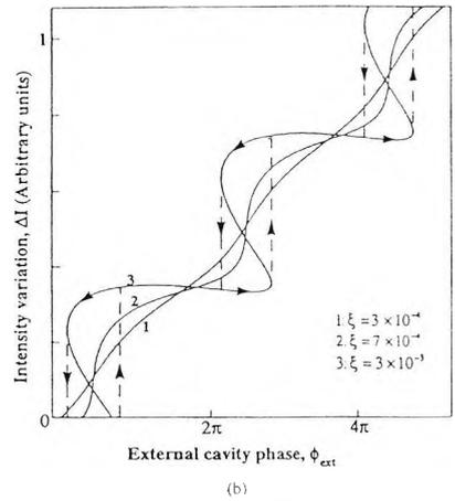
Fig. 3 Theoretical variation of output intensity  $\Delta I$  of a laser diode with feedback with external cavity phase  $\phi_{ext} = 2\pi\nu\tau_2$  due to (a) variation in external cavity length and (b) variation in drive current for three values of feedback coupling coefficient  $\xi$ .
