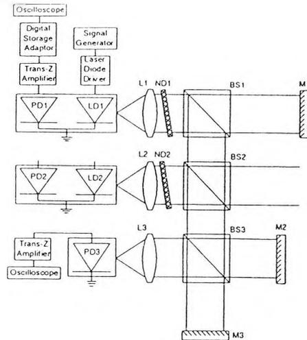
Fig. 4 Experimental arrangement used to study feedback; LD1-2: laser diodes, PD1-3: photodiodes; L1-3: lenses; BS1-3: cube beam splitters; M1-3: plane mirrors; ND1-2: neutral density filters.
