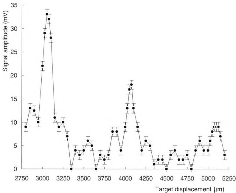
Fig. 4.2. Self-mixing interference visibility pattern for a multimode laser diode with strong feedback.
