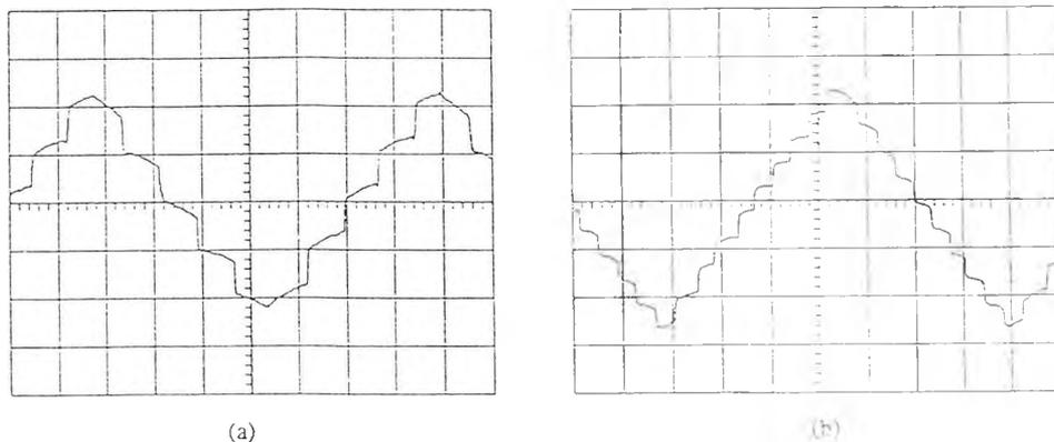
Fig. 6. Oscilloscope traces showing output intensity of a laser diode with feedback with the drive current modulated with a triangular waveform. (Horizontal scale: 2ms/div; vertical scale: 10mV/div.)
