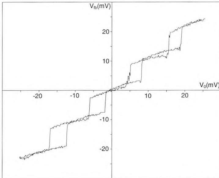
Fig. 3.7. Plot of monitor photodiode output with feedback,  $V_{fb}$ , against output without feedback,  $V_o$ , with triangular wave drive current modulation.
