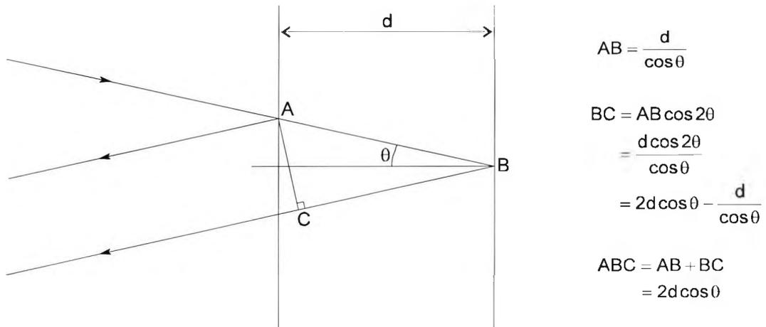
Fig. 1.1. Optical geometry of the Michelson interferometer.
