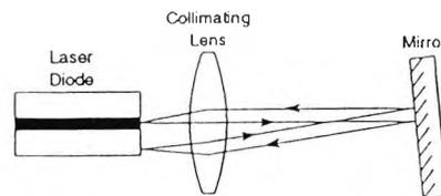
Fig. 8 Path taken by a single ray in an external cavity with a tilted reflector
