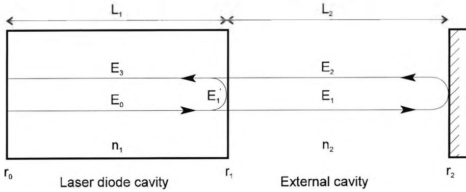
Fig 2.2. Schematic representation of a laser diode with an external reflector showing amplitude reflection coefficients,  $r_i$ , effective refractive indices,  $n_i$ , electric field amplitudes,  $E_i$ , and cavity lengths,  $L_i$ .
