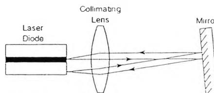
Fig. 9. Path taken by a single ray in an external cavity with a tilted reflector
