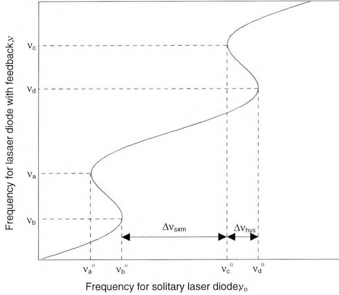
Fig. 2.7. Variation of compound cavity phase change with frequency difference showing single longitudinal mode frequency region,  $\Delta \nu_{sxm}$ , and hysteresis width,  $\Delta \nu_{hys}$ .
