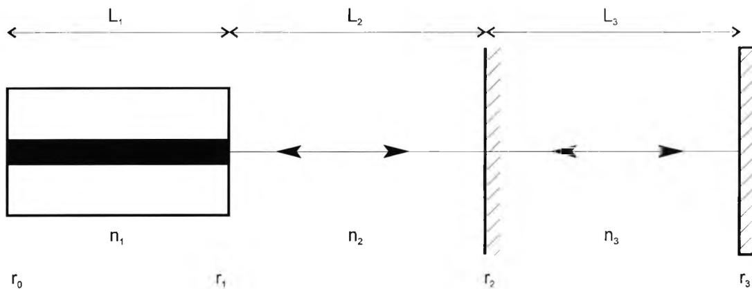
Fig. 5.3. Schematic representation of a laser diode with feedback from two external cavities.
