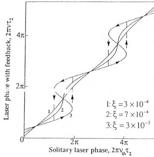
Fig. 1. Theoretical variation of frequency for a laser diode with feedback,  $\nu$ , with solitary laser frequency,  $\nu_0$ , for three values of feedback coupling coefficient,  $\xi$ , with external cavity length,  $L_{\text{ext}}=200\text{mm}$ . Frequencies expressed in terms of external cavity phase.
