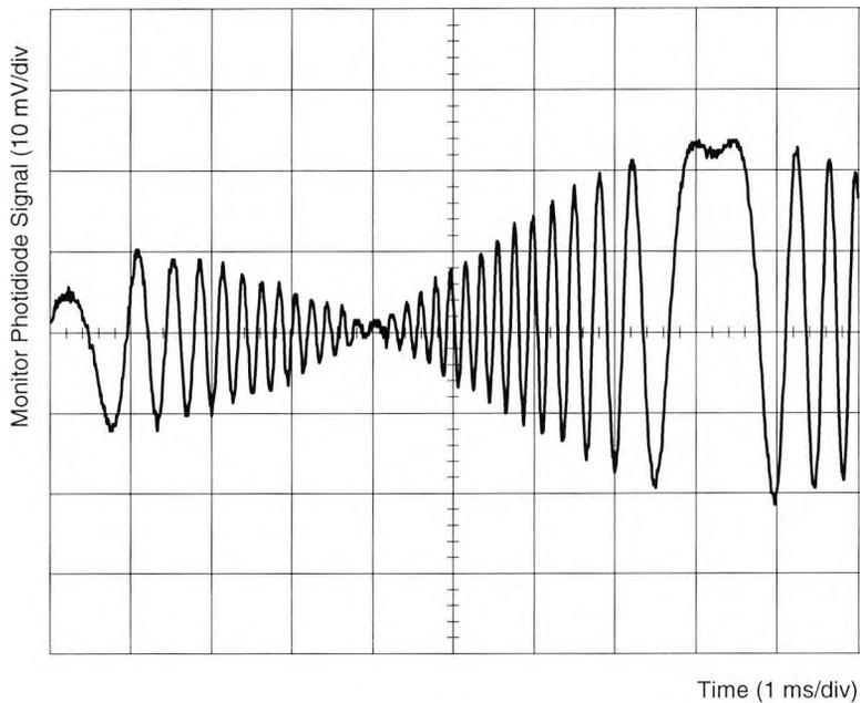
Fig. 3.3 Example of an oscilloscope trace obtained with the dual-wavelength Michelson interferometer.
