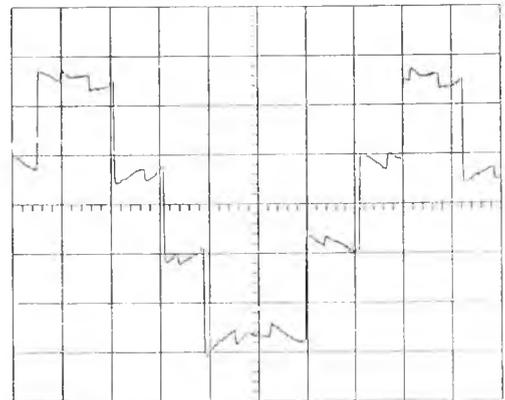
Fig. 4. Oscilloscope trace showing monitor photodiode output from laser with feedback from two external reflectors and with modulated drive current. (Horizontal scale: 2ms/div; vertical scale: 10mV/div.)
