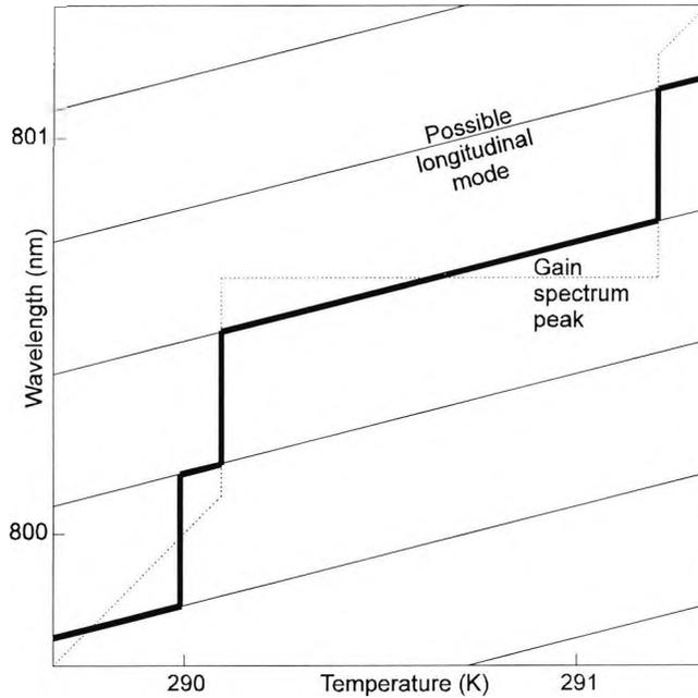
Fig. 5.2 Typical variation of wavelength with temperature for a laser diode with longitudinal mode stabilisation.
