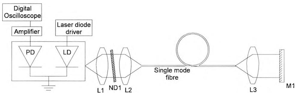
Fig. 4.5. Experimental arrangement used to demonstrate a self-mixing interference-based sensing system.
