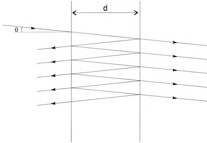
Fig. 1.2. Geometry of the Fabry-Perot interferometer.
