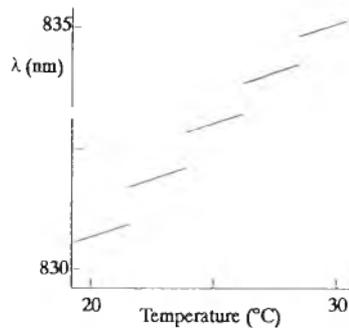
Fig. 2 Typical variation of laser diode wavelength,  $\lambda$ , with temperature.
