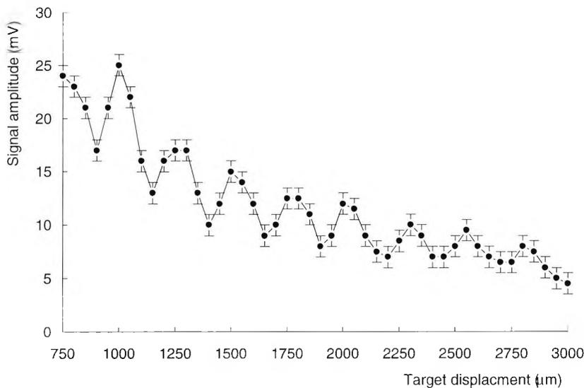
Fig. 4.3. Self-mixing interference visibility pattern for a single mode laser diode with feedback controlled by a neutral density filter.
