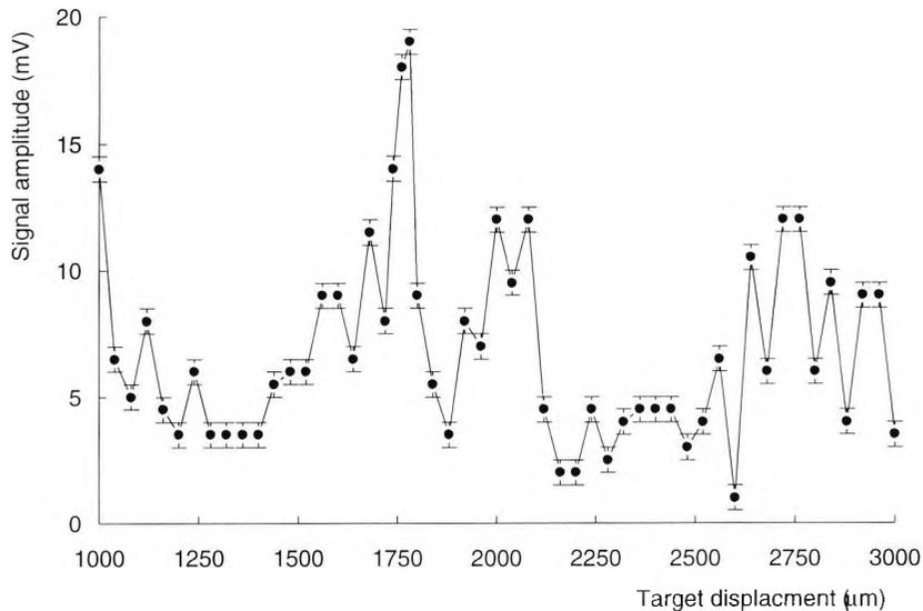
Fig. 4.4. Self-mixing interference visibility pattern recorded using a micro-prism embedded retro-reflecting paper target.
