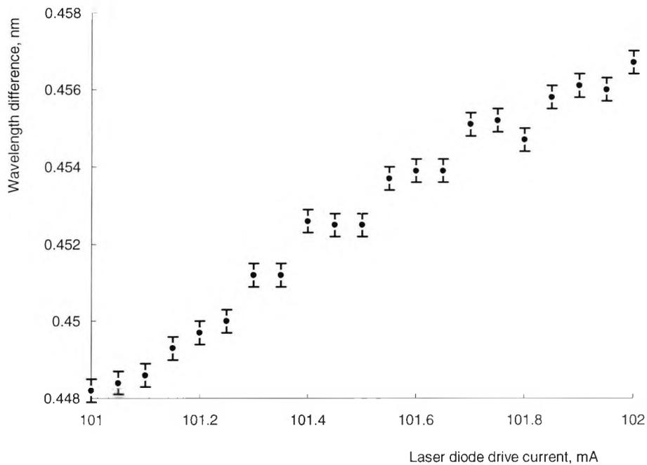
Fig. 5.5 Variation of wavelength for a laser diode with feedback measured using the dual-wavelength Michelson interferometer.
