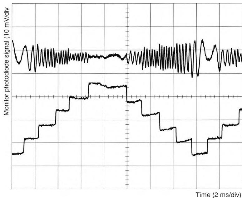
Fig. 6.3 Oscilloscope traces showing simultaneous output from laser diode with double frequency intensity modulation and output from a dual wavelength interferometer.
