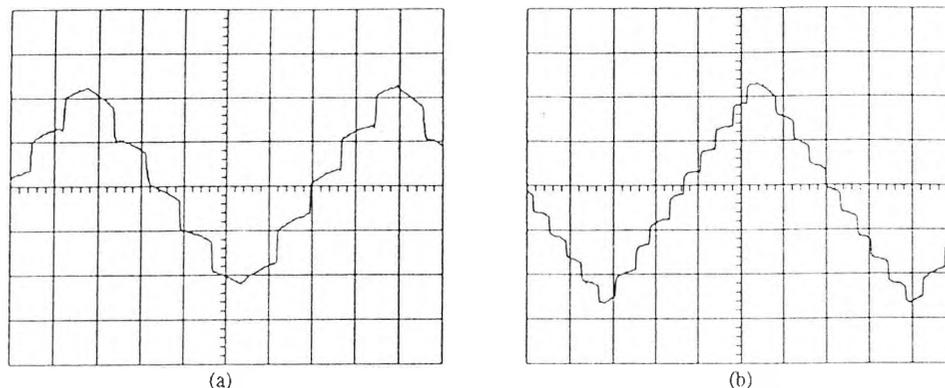
Fig. 3. Oscilloscope traces showing output intensity of a laser diode with feedback with the drive current modulated with a triangular waveform. (Horizontal scale: 2ms/div; Vertical scale: 10mV/div.)
