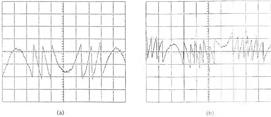
Fig. 7. Oscilloscope traces showing output intensity of a laser diode with feedback with the external cavity length modulated using a loudspeaker mounted mirror. (Horizontal scale: 2ms/div; vertical scale: 10mV/div.)
