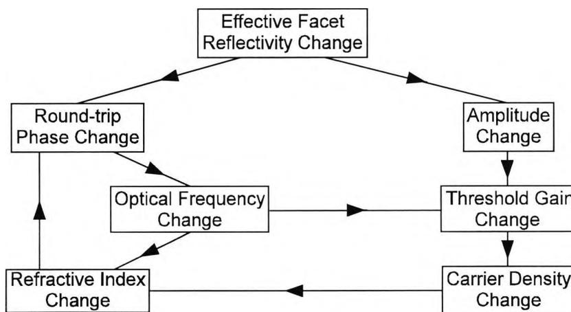
Fig. 2.1 Block diagram showing the relationships between the physical parameters affected by external optical feedback.
