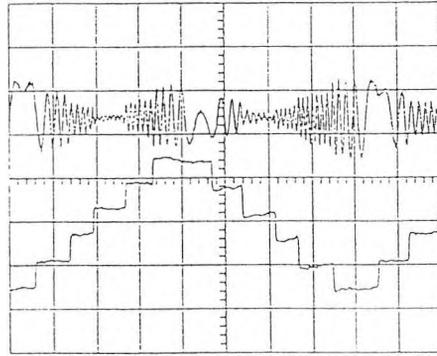
Fig. 8. Oscilloscope traces showing intensity output of a laser diode with feedback with drive current modulation (lower trace) and simultaneous dual-wavelength Michelson interferometer output (upper trace). (Horizontal scale: 2ms/div; Vertical trace: 10mv/div).
