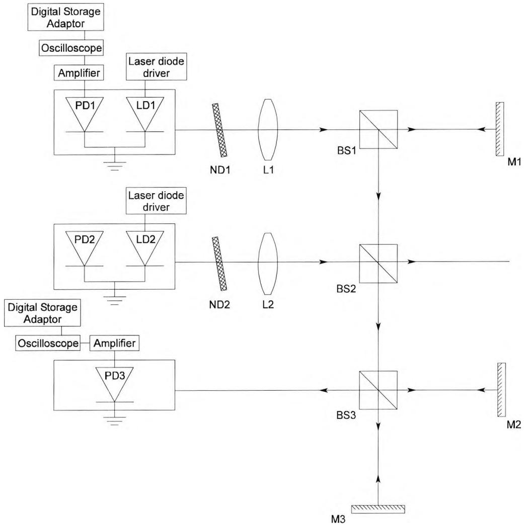
Fig. 3.1. Typical experimental set-up; LD<sub>i</sub>: laser diodes; PD<sub>i</sub>: monitor photodiodes; L<sub>i</sub>: collimating lenses; ND<sub>i</sub>: neutral density filters; BS<sub>i</sub>: beamsplitters; M<sub>i</sub>: mirrors.
