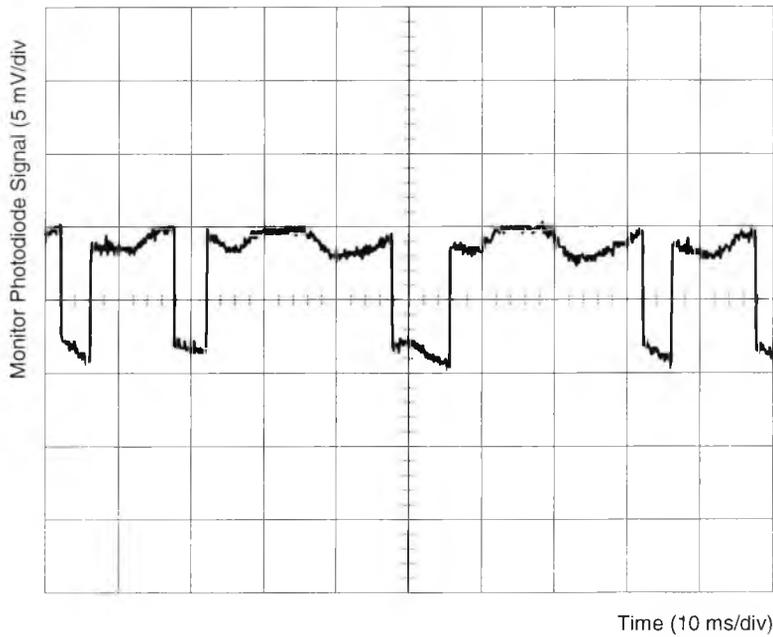
Fig. 3.8 Oscilloscope trace showing laser diode optical power output as mode-hopping occurs between external cavity longitudinal modes under stationary conditions.
