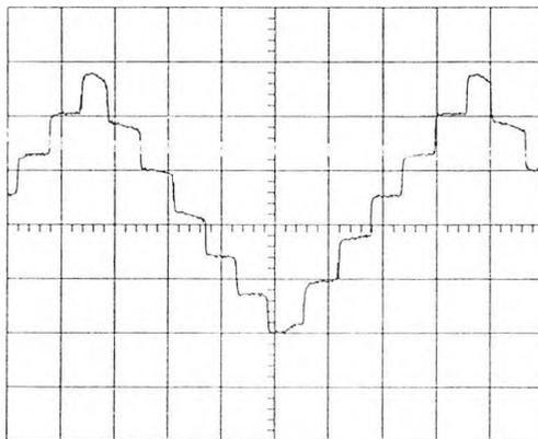
Fig. 3. Oscilloscope trace showing monitor photodiode output from laser with feedback from a single external reflector and with modulated drive current. (Horizontal scale: 2ms/div; vertical scale: 10mV/div.)
