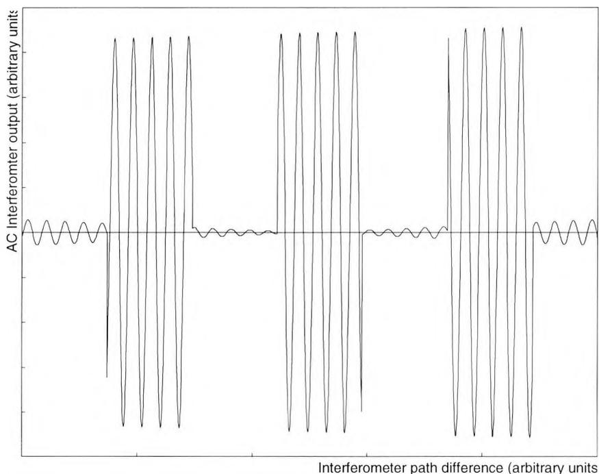
Fig. 6.4. Calculated visibility pattern for a dual wavelength interferometer when one laser diode undergoes hopping between laser diode cavity longitudinal modes.
