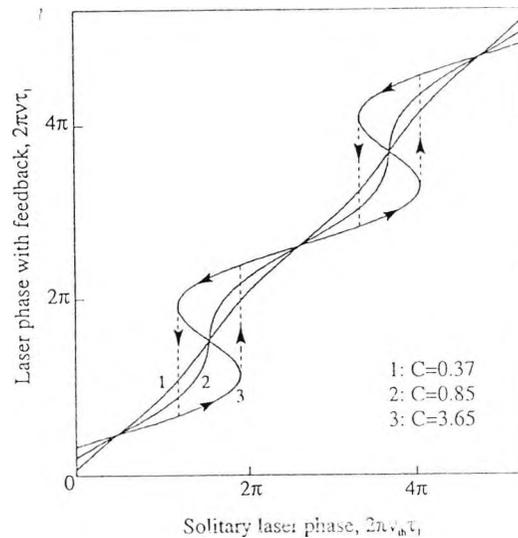
Fig. 1. Variation of laser frequency with feedback from a single external reflector with solitary laser frequency, expressed in terms of external cavity round trip phase, for various feedback strengths.
