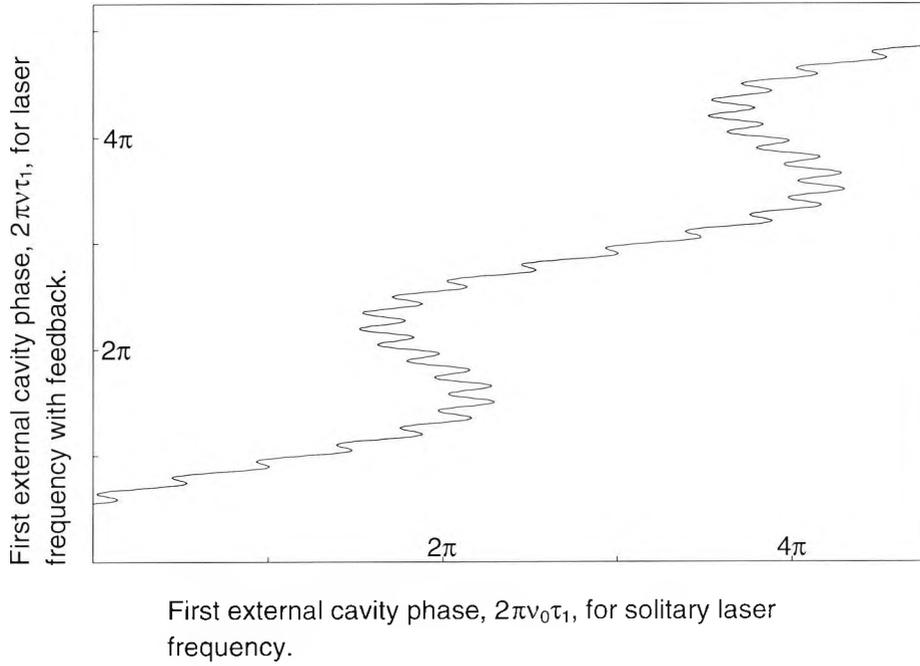
Fig. 5.4. Variation of laser frequency with feedback from two external reflectors with solitary laser frequency, expressed in terms of round trip phase in the first external cavity, for  $L_1=25\text{mm}$ ,  $L_2=300\text{mm}$ ,  $R_2=2.5 \times 10^{-5}$ ,  $R_3=10^{-6}$ .
