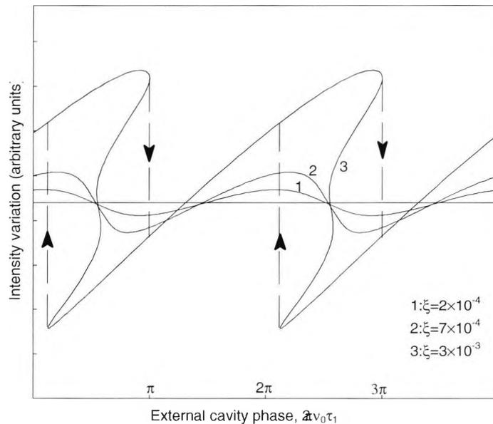
Fig. 2.6. Intensity variation with external cavity phase when linewidth and coherence length are phase dependent.
