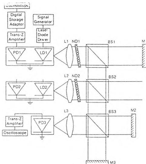
Fig. 5. Experimental arrangement used to study feedback. LD1-2: laser diodes; PD1-3: photodiodes; L1-3: lenses; BS1-3: cube beamsplitters; M1-3: plane mirrors; ND1-2: neutral density filters.
