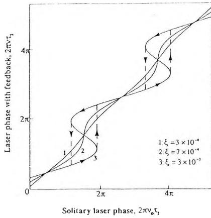
Fig. 2 Theoretical variation of frequency for a laser diode with feedback  $\nu$  with solitary laser frequency  $\nu_{th}$  for three values of feedback coupling coefficient  $\xi$  with external cavity length  $L_{ext} = 200$  mm. Frequencies expressed in terms of external cavity phase.
