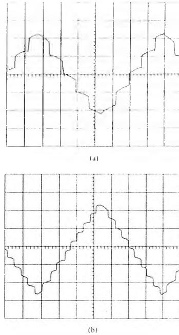
Fig. 5. Oscilloscope traces showing output intensity of a laser diode with feedback with the drive current modulated with a triangular waveform (a) Normal intensity modulation frequency. (b) Double intensity modulation frequency. (Horizontal scale: 2 ms/div; vertical scale: 10 mV/div.)
