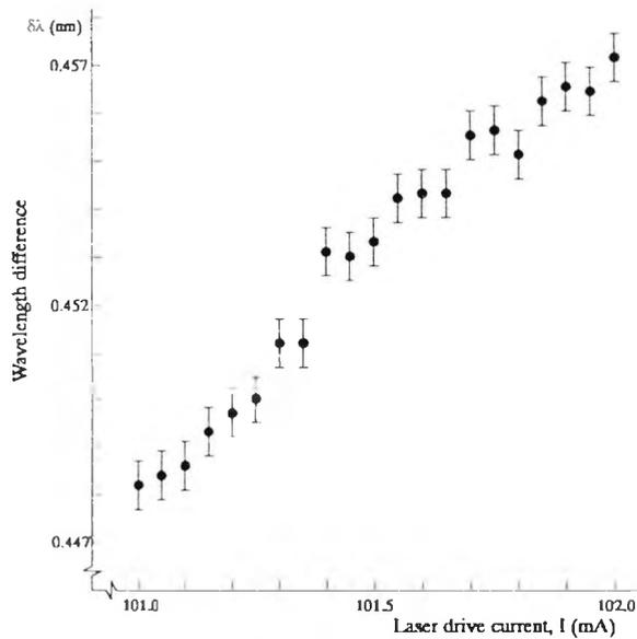
Fig. 4 Measured variation of wavelength with drive current for a laser diode with strong optical feedback.
