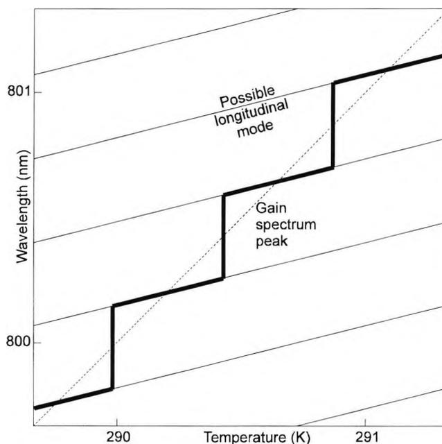
Fig. 5.1 Typical variation of laser diode wavelength with temperature.
