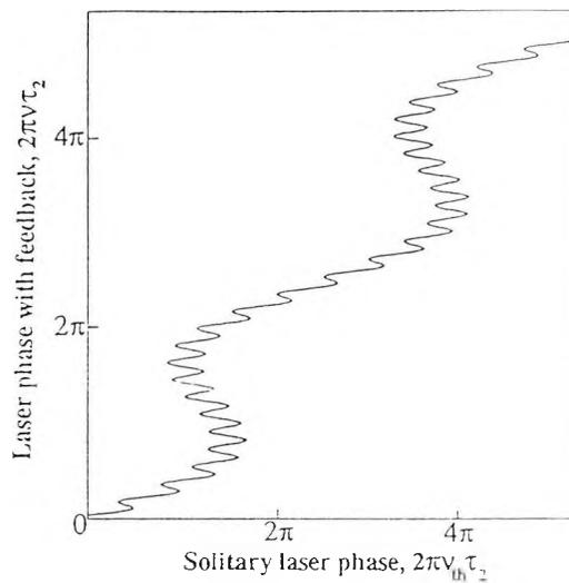
Fig. 4. Theoretical variation of frequency,  $\nu$ , for a laser diode with two external reflectors with variation in solitary laser frequency,  $\nu_{th}$ . Frequencies expressed in terms of first external cavity phase.
