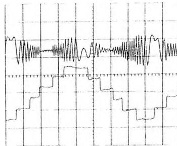
Fig. 7 Oscilloscope traces showing intensity output of a laser diode with feedback with drive current modulation (lower trace) and simultaneous dual wavelength Michelson interferometer output (upper trace) (Horizontal scale 2 ms/div, vertical trace 10 mV/div)
