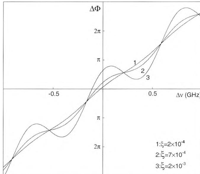
Fig. 2.3. Variation of compound cavity phase change,  $\Delta\Phi$  with frequency change,  $\Delta\nu$ .  $n_1L_1=1\text{mm}$ ,  $L_2=20\text{mm}$ ,  $\alpha=5$ .
