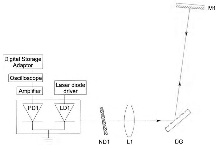
Fig. 5.7. Experimental arrangement with feedback from two external reflectors. LD1: laser diode; PD1: monitor photodiode; ND1: neutral density filter; DG: L1: collimating lens; diffraction grating; M1: mirror.
