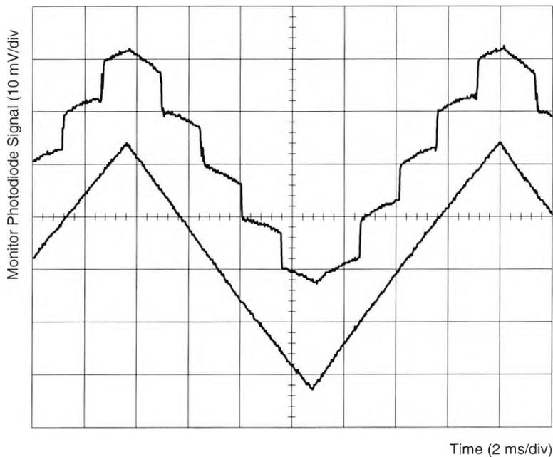
Fig. 3.6 Oscilloscope trace showing monitor photodiode output for a laser diode with feedback (upper trace) and without (lower trace) with triangular wave drive current modulation.
