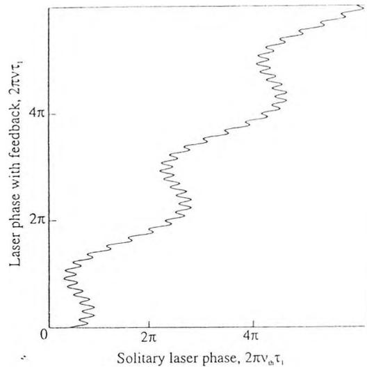
Fig. 2. Variation of laser frequency with feedback from two external reflectors with solitary laser frequency, expressed in terms of round trip phase in the first external cavity, for  $L_1=25\text{mm}$ ,  $L_2=300\text{mm}$ ,  $R_2=2\times 10^{-5}$ ,  $R_3=10^{-6}$
