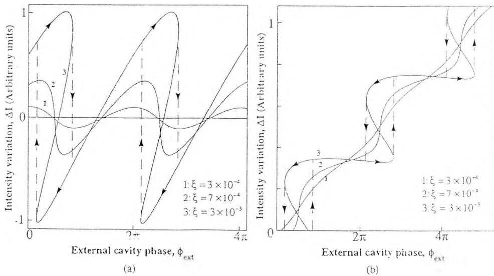
Fig. 3. Theoretical variation in output intensity,  $\Delta I$  of a laser diode with feedback with external cavity phase,  $\phi_{ext} = 2\pi\nu\tau_2$  due to (a) variation in external cavity length, and (b) variation in drive current, for three values of coupling coefficient,  $\xi$ .
