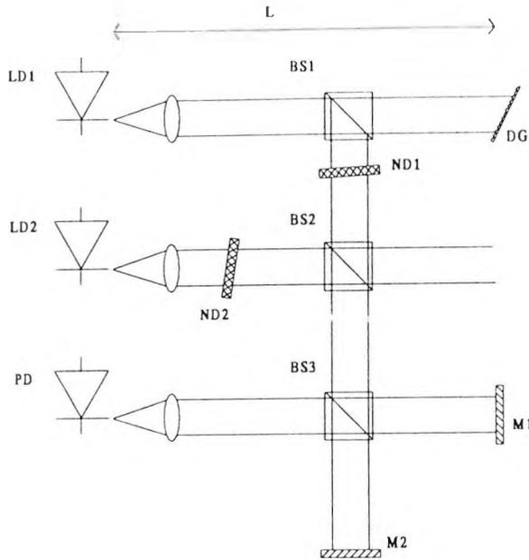
Fig. 3 Experimental arrangement; LD1, LD2: Laser diodes; DG: Diffraction grating; PD: Photodiode; BS1, BS2, BS3: Beam-splitters; ND1, ND2: Neutral density filters; M1, M2: Mirrors.
