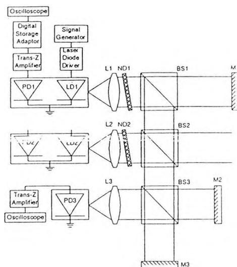
Fig. 2. Experimental arrangement used to study feedback. LD1-2: laser diodes. PD1-3: photodiodes; L1-3: lenses; BS1-3: cube beamsplitters. M1-3: plane mirrors; ND1-2: neutral density filters.
