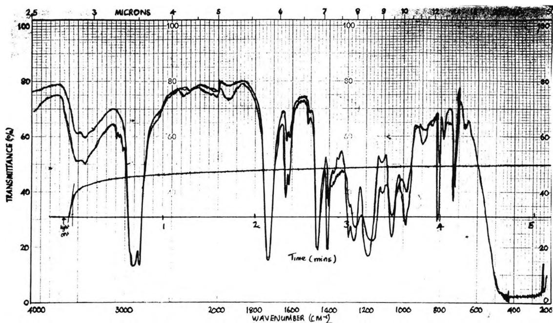
Spectrum 5: RTIR spectrum, showing the polymerization of 2-ethyl-2(hydroxymethyl)-1,3 propanediol triacrylate in the presence of 2,3-bis(4-methoxyphenyl) quinoxaline and N-methyldiethanolamine, under anaerobic conditions.
