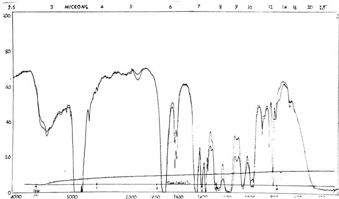
Spectrum 4: RTIR spectrum, showing the polymerization of 2-ethyl-2(hydroxymethyl)-1,3-propanediol triacrylate in the presence of 2,3-bis(4-hydroxyphenyl)quinoxaline and N-methyldiethanolamine, under anaerobic conditions
