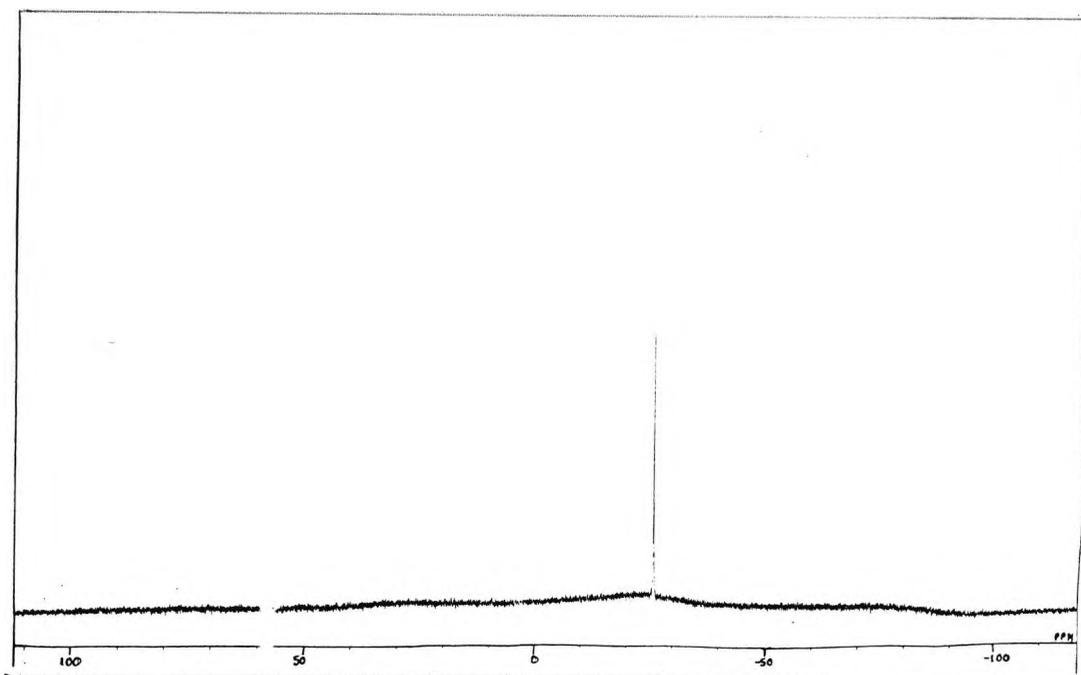
Spectrum 2: <sup>11</sup>B spectrum of methylene-blue-n-butyltriphenylborate
