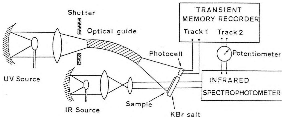
Fig. 2.1 Experimental device for real-time monitoring of uv curing reactions.
