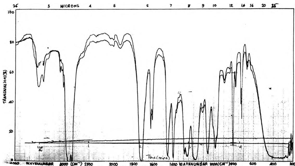
Spectrum 4:- RTIR spectrum, showing the polymerization of 2-ethyl-2(hydroxymethyl)-1,3-propanediol triacrylate in the presence of  $n^6$ -dichlorobenzene- $n^5$ -cyclopentadienyliron(II)- $n$ -butyltriphenylborate, under aerobic conditions.
