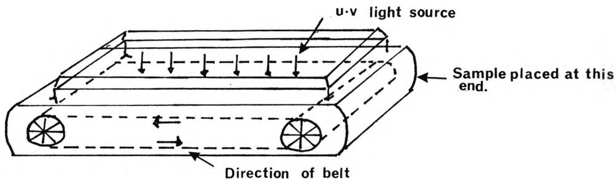
Fig. 2.3 A Moving Belt System
