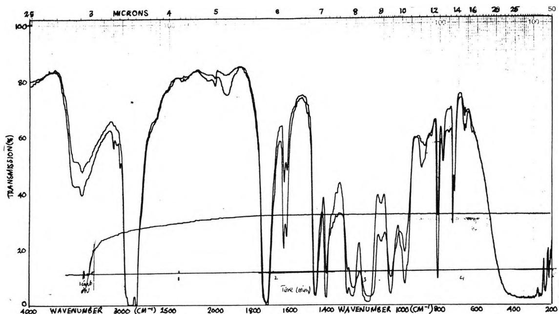
Spectrum 1: RTIR spectrum, showing the polymerization of 2-ethyl-2 (hydroxymethyl)-1,3-propanediol triacrylate in the presence of an amine and pyrenediazonium tetrafluoroborate, under anaerobic conditions.
