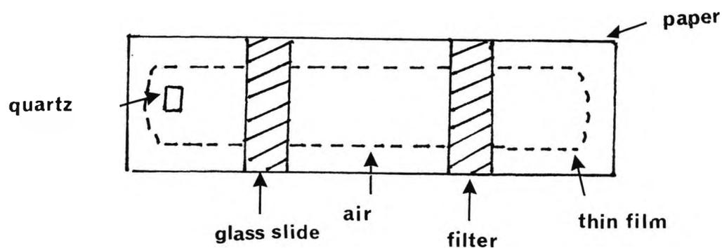
Fig. 2.4 A diagram showing a prepared thin film before exposure to u.v. radiation.
