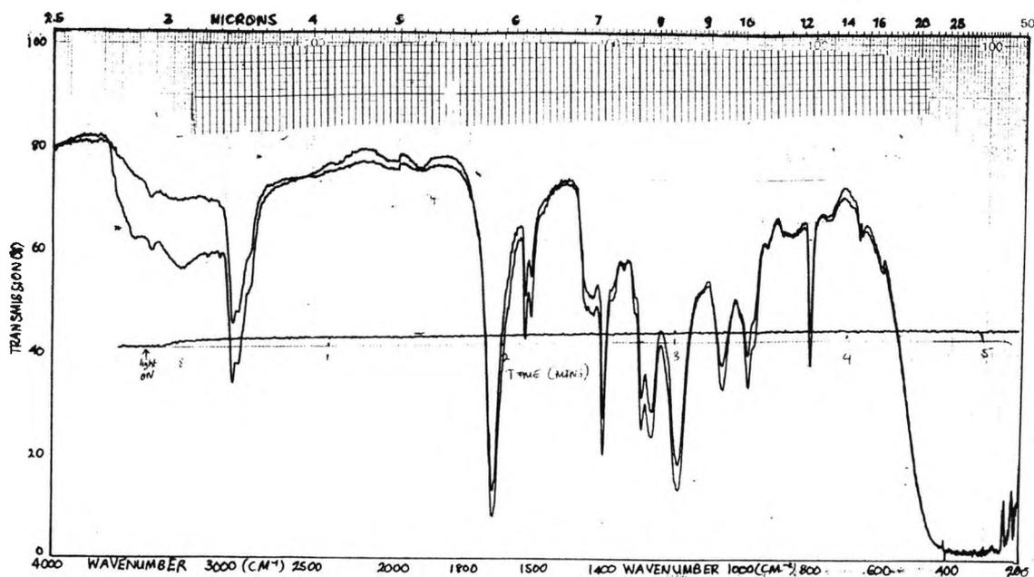
Spectrum 6:- RTIR spectrum showing the polymerization of 2,2-thiodiethyl diacrylate in the presence of Irgacure 907, under aerobic conditions.
