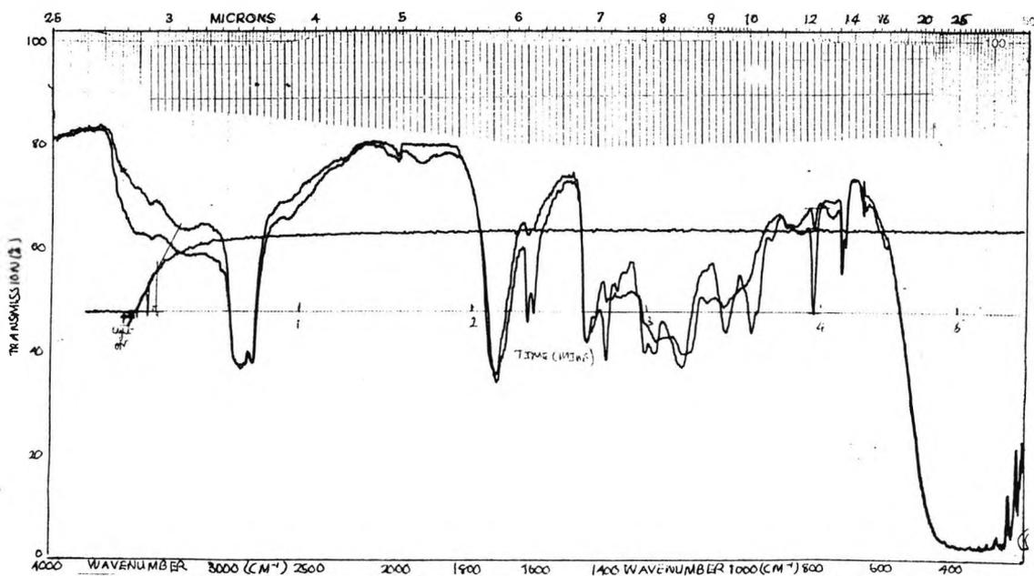
Spectrum 5:- RTIR spectrum showing the polymerization of 2,2-thiodiethyl diacrylate in the presence of Irgacure 907, under anaerobic conditions.
