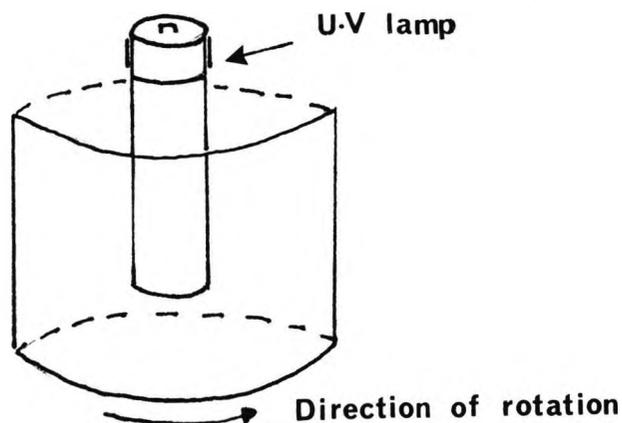
Fig. 2.2 Apparatus used in bulk polymerization
