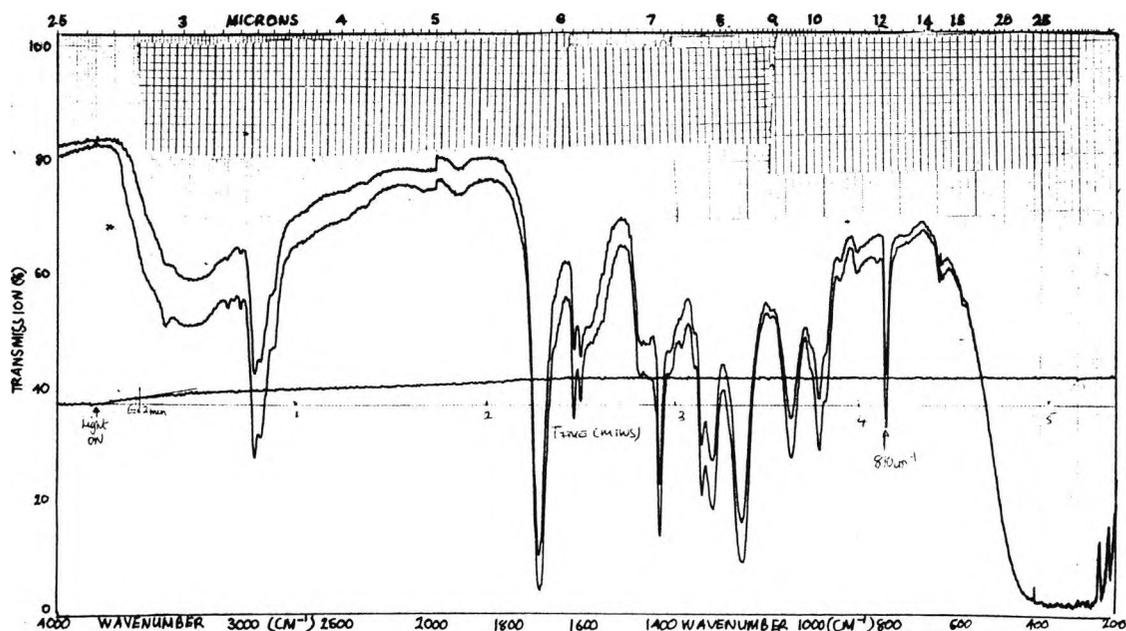
Spectrum 4:- RTIR spectrum, showing the polymerization of 3,6-dithia - 1,8 octane diacrylate in the presence of Irgacure 907 and N-methyldiethanolamine, under aerobic conditions.
