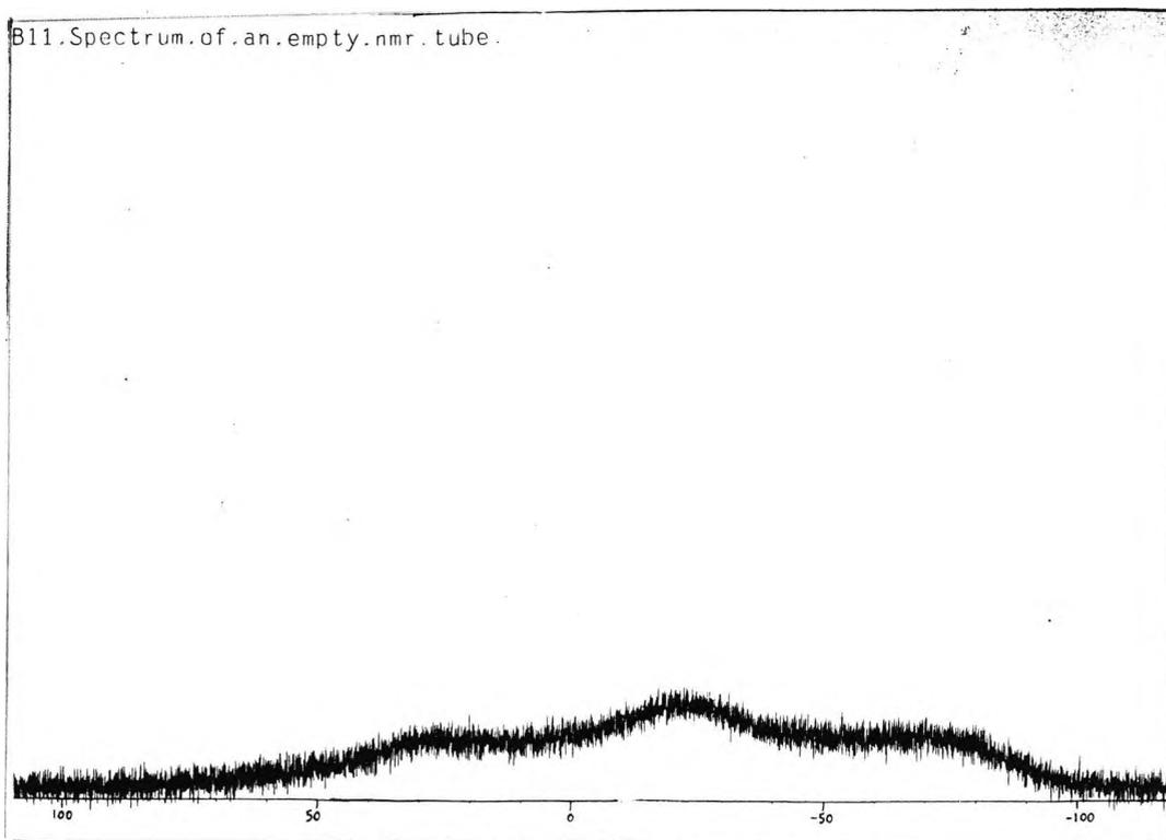
Spectrum 3:  $^{11}\text{B}$  spectrum of an empty NMR tube
