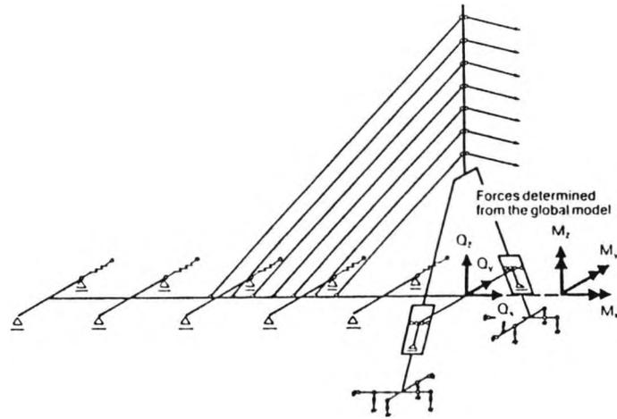
(a) DUSSELDORF-FELHE BRIDGE: PARTIAL MODEL INTENDED FOR THE DESIGN OF PYLON.
