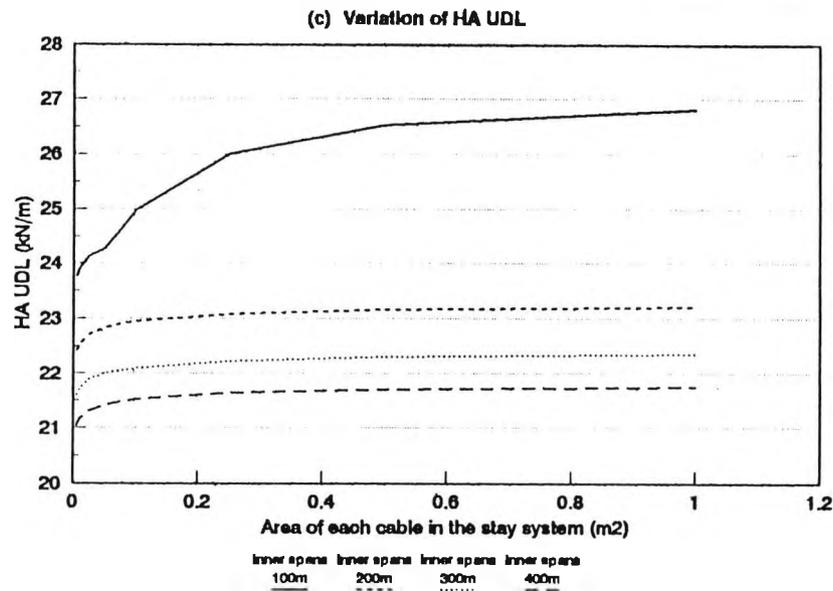
FIGURE 5.20. VARIATION OF HA LOADING PARAMETERS FOR FOUR CABLE-STAYED BRIDGES WITH DIFFERENT SPANS ARRANGEMENT.
