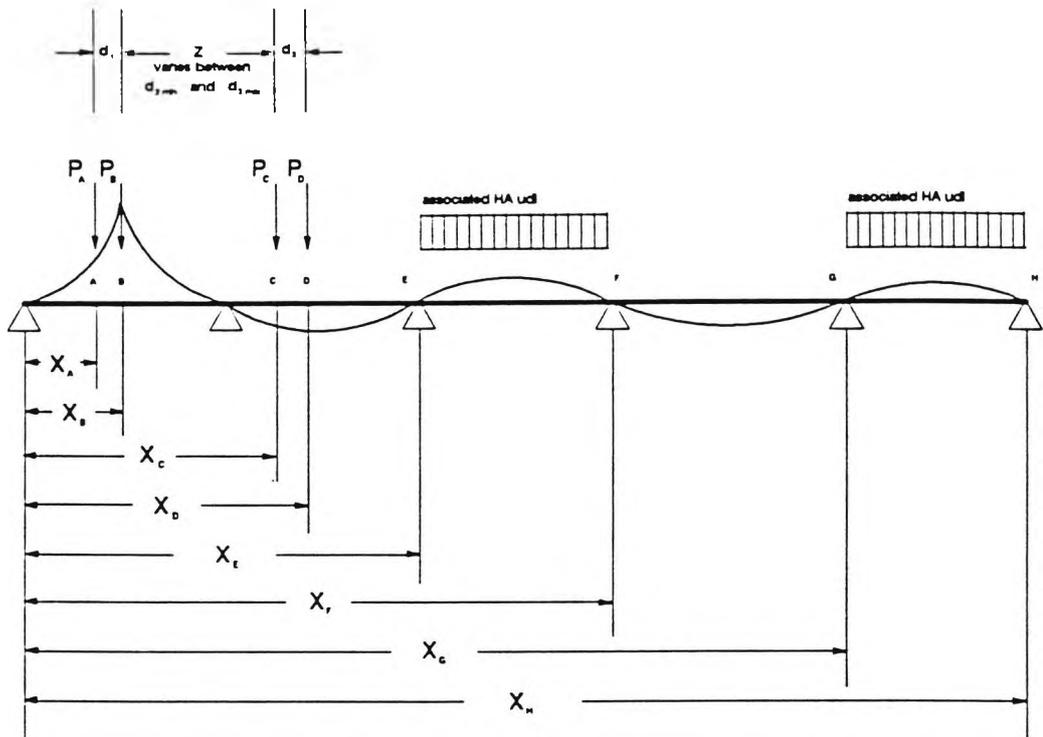
FIGURE 5.10. INFLUENCE LINE LOADED BY HB AND ASSOCIATED HA LOADING.
