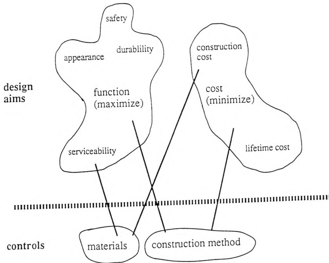
**FIGURE 2.1. A REPRESENTATION OF BRIDGE DESIGN SPACE.**
