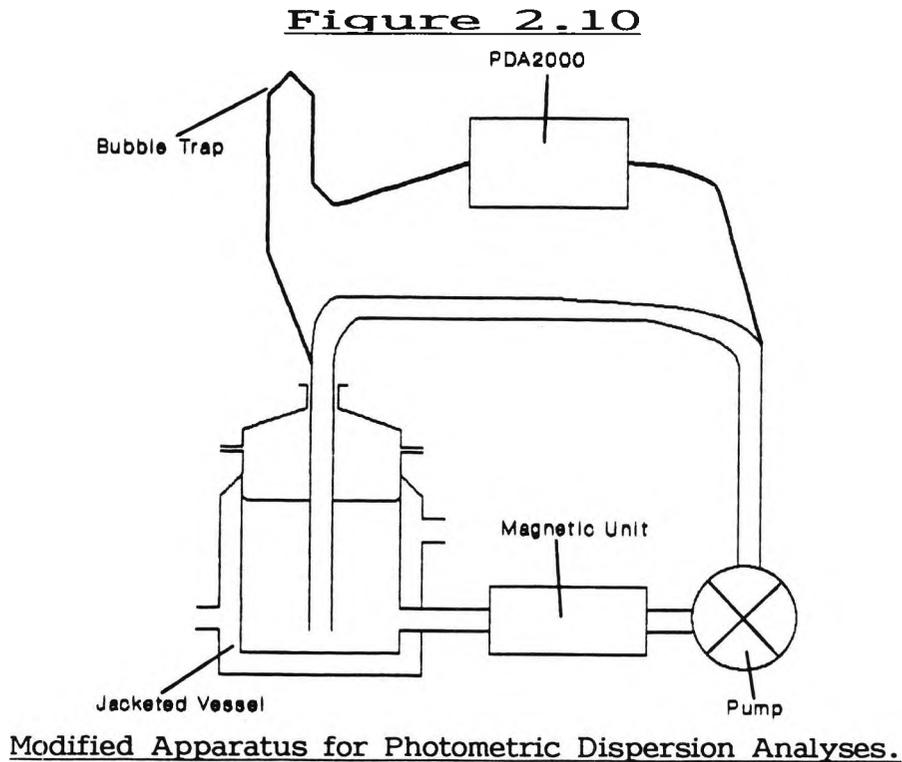
Many tests were carried out using this apparatus. For these experiments the oxalate solution was added to the vessel after five minutes and the circulation of the solution was continued. The results of these analyses were in very good agreement with the particle size results previously presented, i.e. the effect of the magnetic treatment was to give smaller particles. Figures 2.11 and 2.12 show typical results of control and magnetic test runs.
