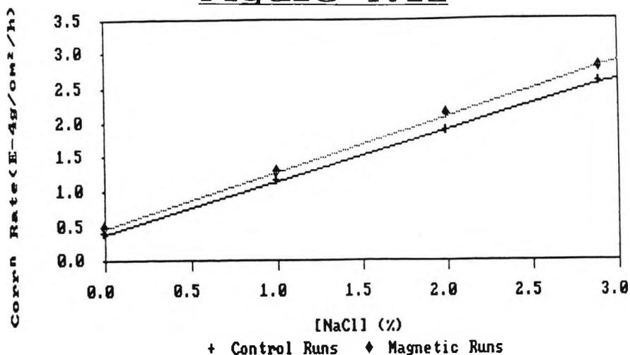
Corrosion Rates at Different [NaCl] Concentrations
