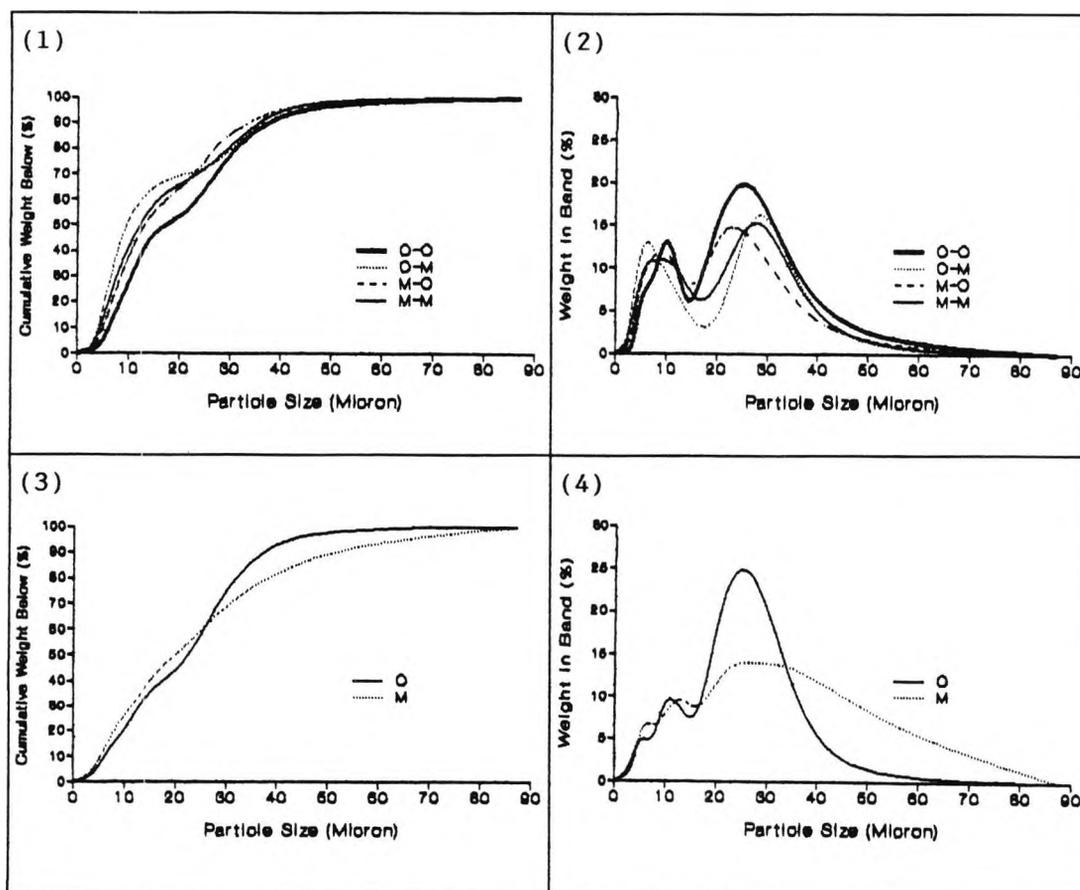
Particle Size Distribution Graphs - Barium in Aqueous Sol<sup>n</sup> & Sulphate in 2.9% NaCl<sub>(aq)</sub> with Ca<sup>2+</sup>, Sr<sup>2+</sup>, HCO<sub>3</sub><sup>-</sup> (X-Y\*).
