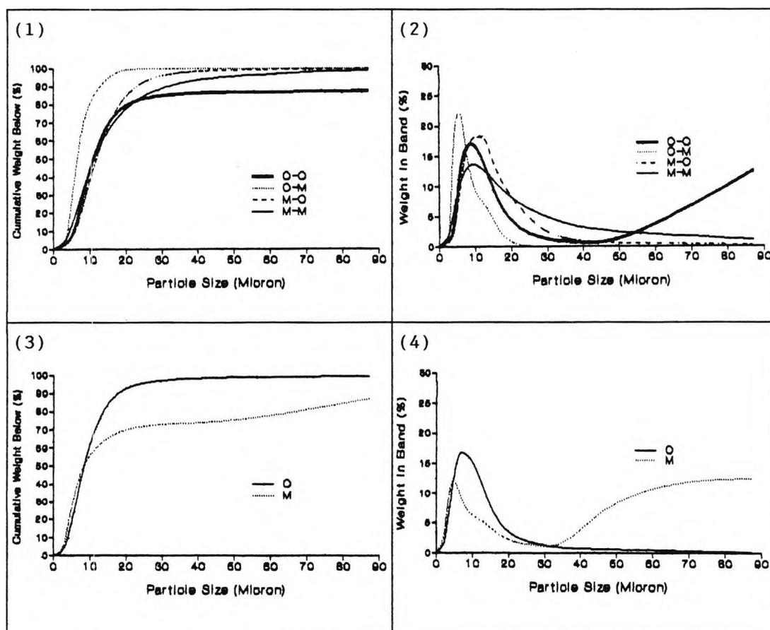
Particle Size Distribution Graphs - Barium in Saturated  $\text{BaSO}_4(\text{aq})$  and Sulphate in 2.9%  $\text{NaCl}(\text{aq})$  ( $X^S$ - $Y^*$ ).
