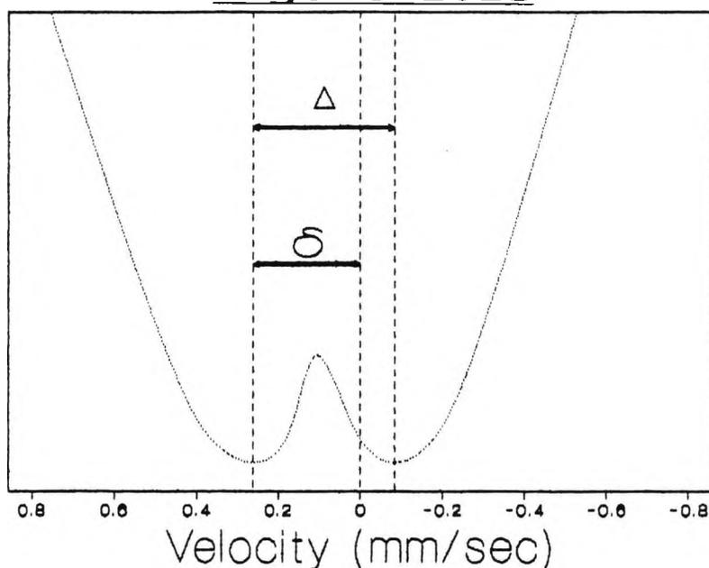
Measurement of  $\delta$  and  $\Delta$  for a Mössbauer Spectrum.
