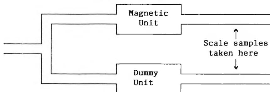
Schematic Diagram of Industrial Test Site.
