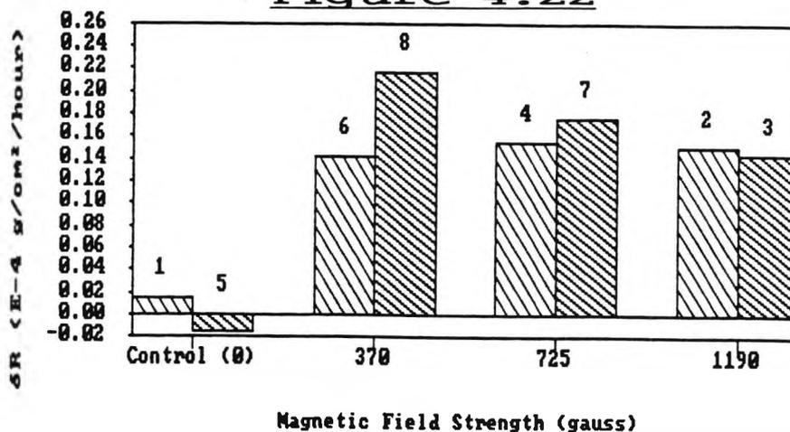
Graph of Corrosion Rate Results for Experiment 25.
