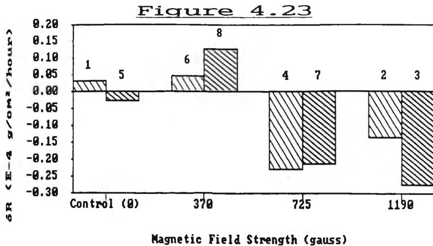
The results of Experiments 17 to 25 show that, above a certain flow rate and field strength, the effect of the treatment is to increase the corrosion rate. Below this minimum flow rate, lower field strengths were found to cause an increase in the corrosion rate, while higher field strengths caused a reduction.
