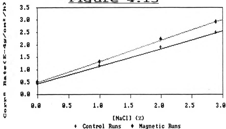
Corrosion Rates at Different [NaCl] Concentrations
