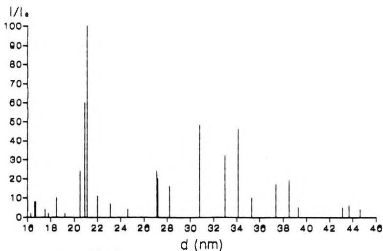
X-ray Diffractogram for O-O Run Sample.
