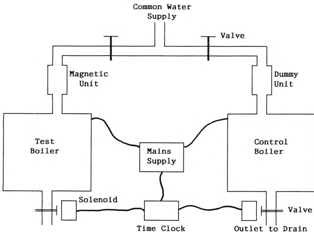
Arrangement of Boilers for Scale Prevention Experiments.
