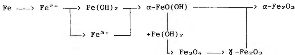
Hiller's Scheme for the Mechanism of Corrosion.
