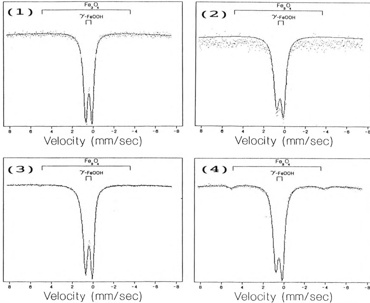
Room Temperature Mössbauer Spectra of Corrosion Products from Experiment 16
