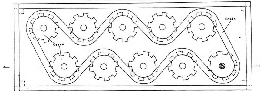
Plan View of the Stirring System Used with the Multiple Test Rig.
