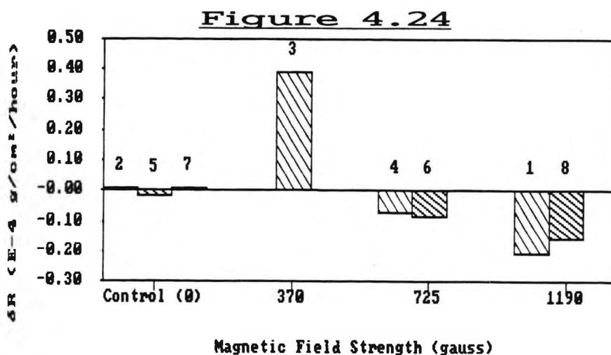
Graph of Corrosion Rate Results for Experiment 27.
