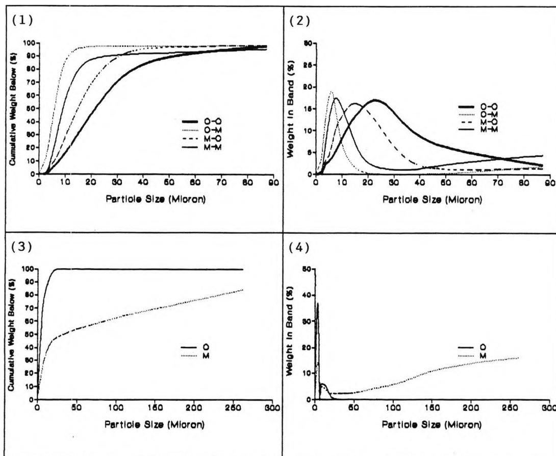
Particle Size Distribution Graphs - Both Barium and Sulphate in 2.9% NaCl<sub>(aq)</sub> (X\*-Y\*).
