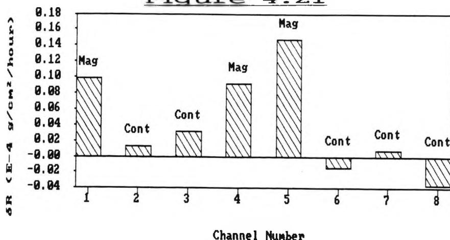
Graph of Corrosion Rate Results for Experiment 24.
