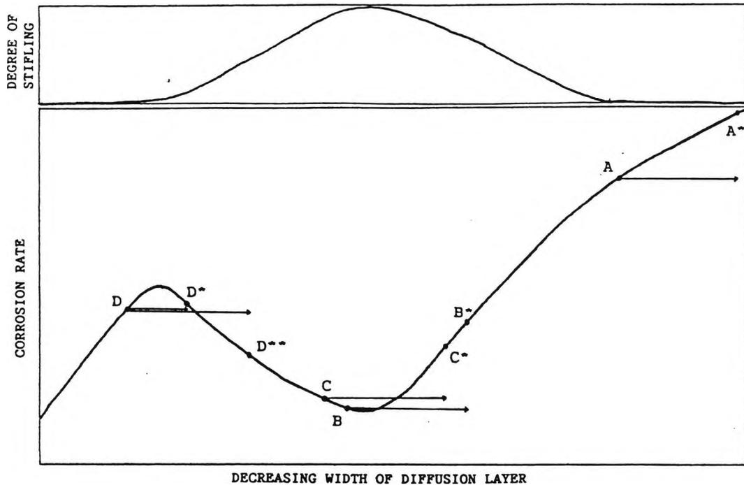
Effect of Decreasing Diffusion Layer Width on Stifling and Corrosion.
