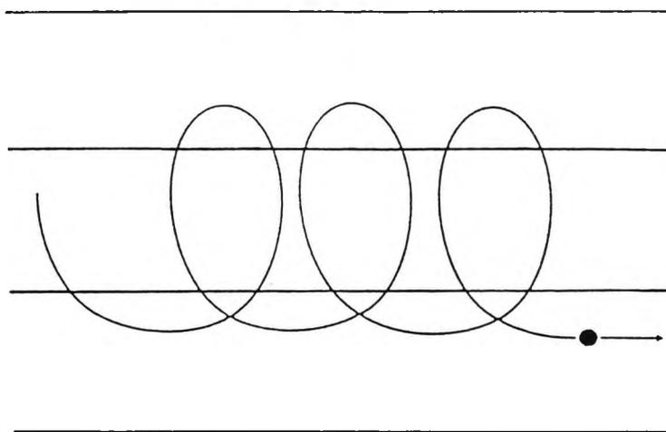
Helical Motion of a Charged Particle in a Uniform Magnetic Field.
