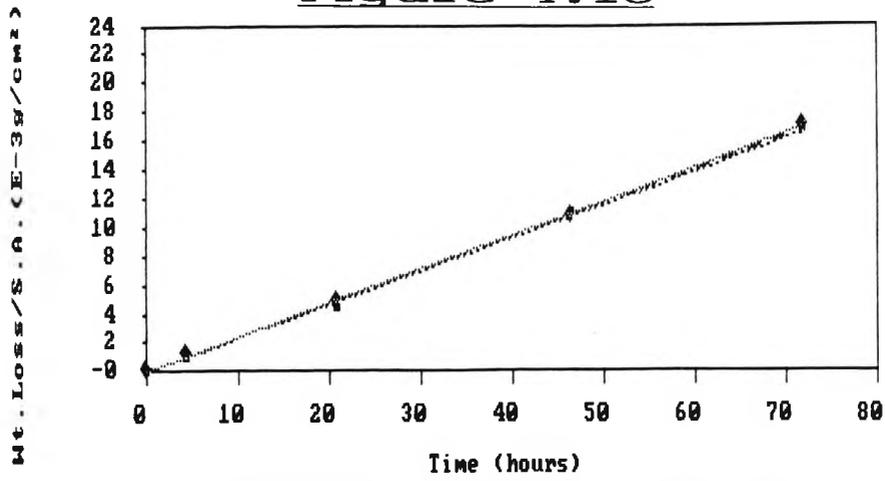
Control Corrosion Rate Results for Experiment 16.
