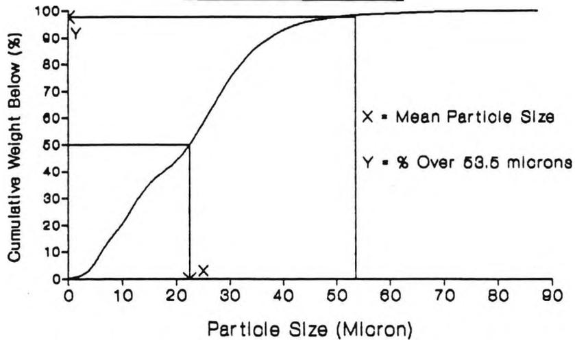
Particle Size Analysis as Cumulative Weight Below vs. Particle Size.
