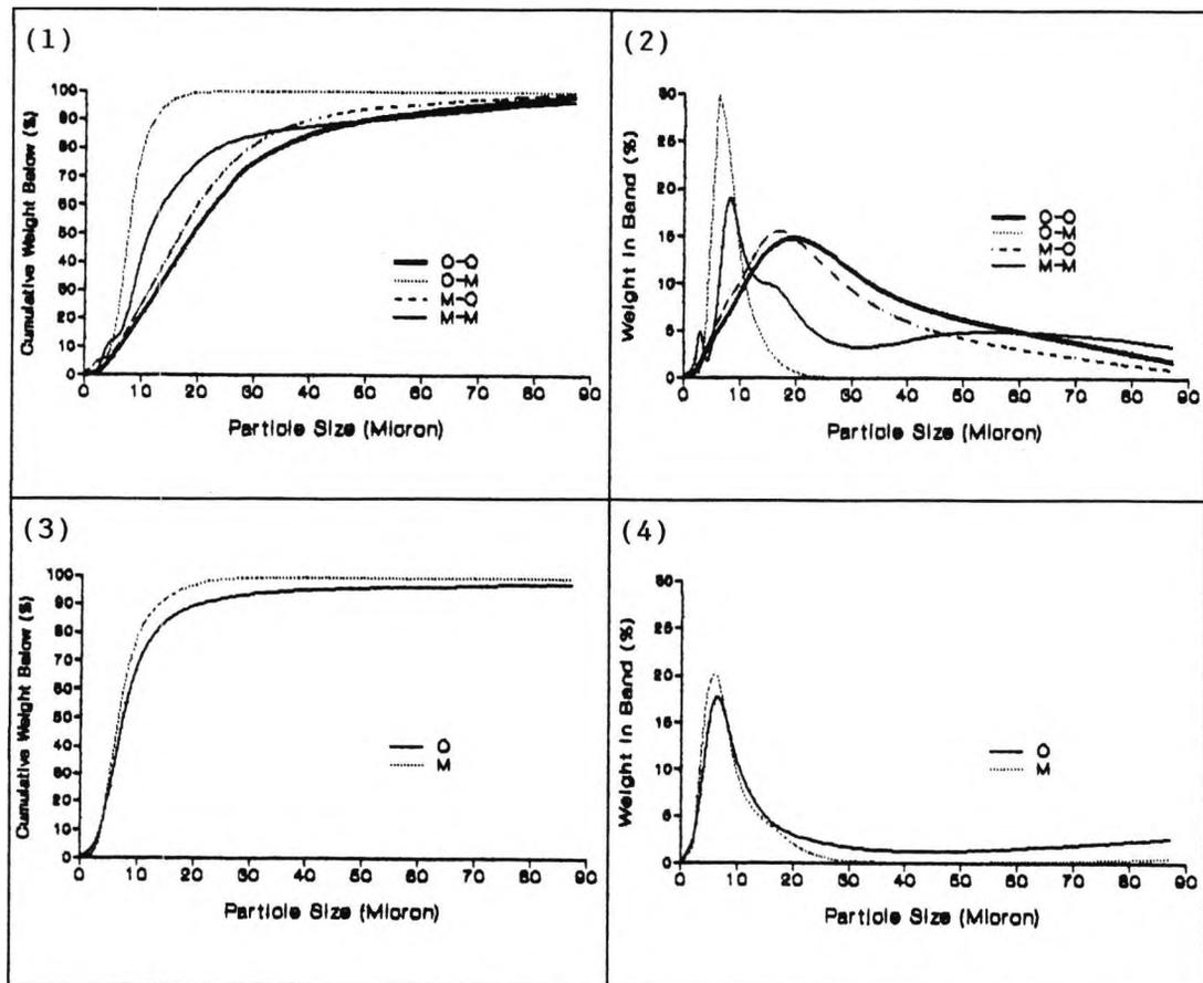
Particle Size Distribution Graphs - Barium in Aqueous Sol<sup>n</sup> and Sulphate in 2.9% NaCl<sub>(aq)</sub> (X-Y\*)
