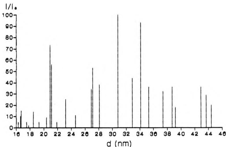
X-ray Diffractogram for M-M Run Sample.
