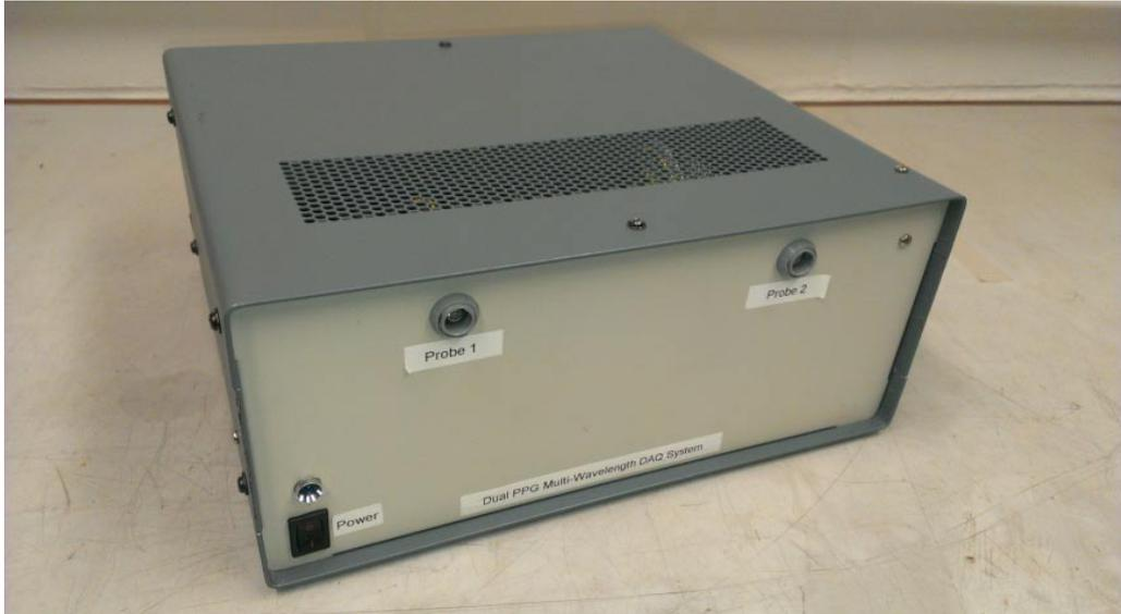
Figure 7.28: Completed dual PPG instrument front panel.
