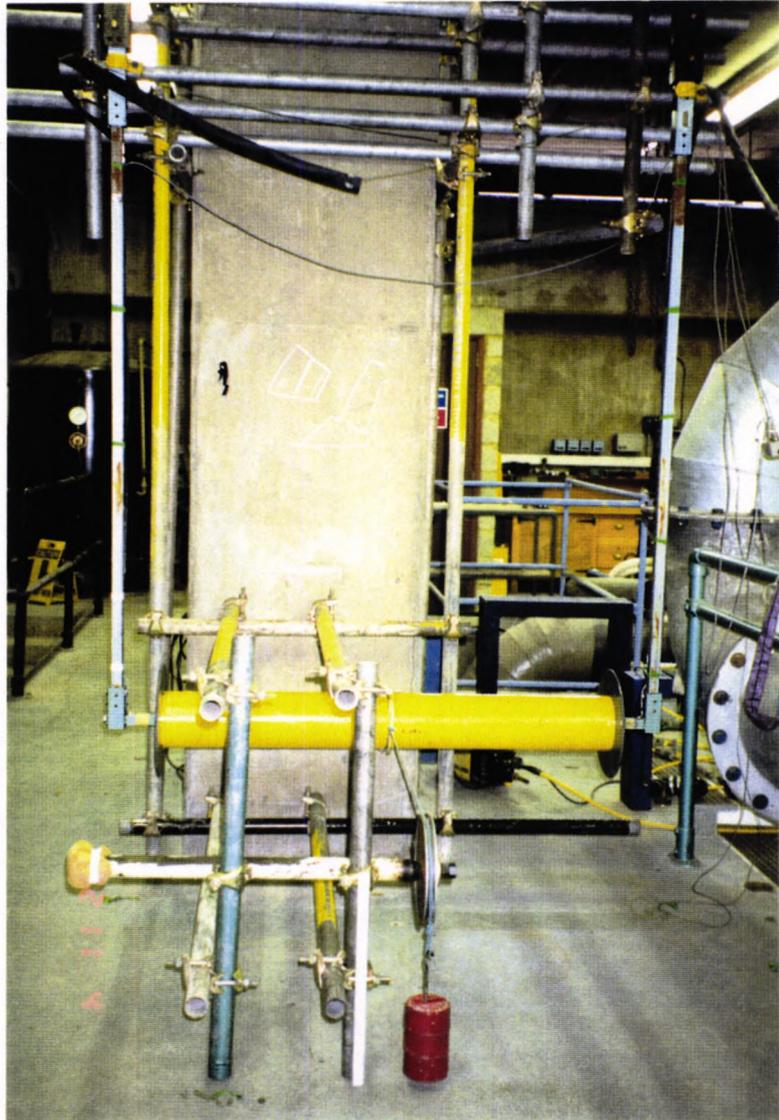
Fig: 3.5 (a) In-line Force Calibration Arrangement
