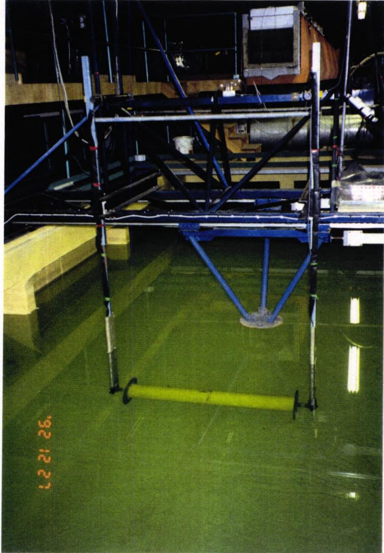
Fig: 3.3 (a) Test Cylinder in Oscillatory Flow
