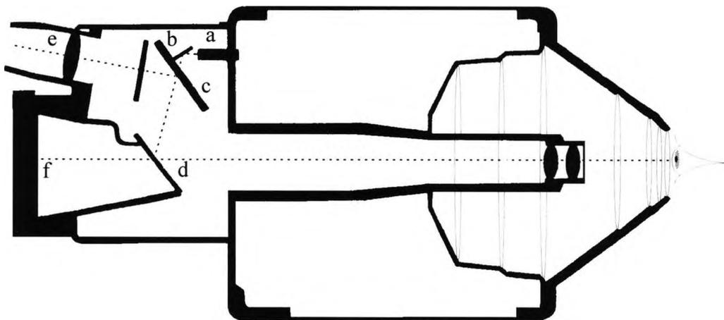
Figure 4.2 PEK instrument optics.
