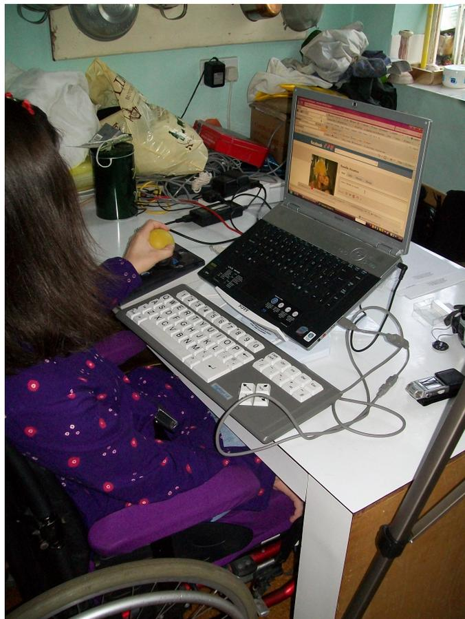
**Figure 26.** Participant using a joystick, large QWERTY keyboard, laptop adjuster, UI zoom software. The participant was also using screenreader software (video still).
