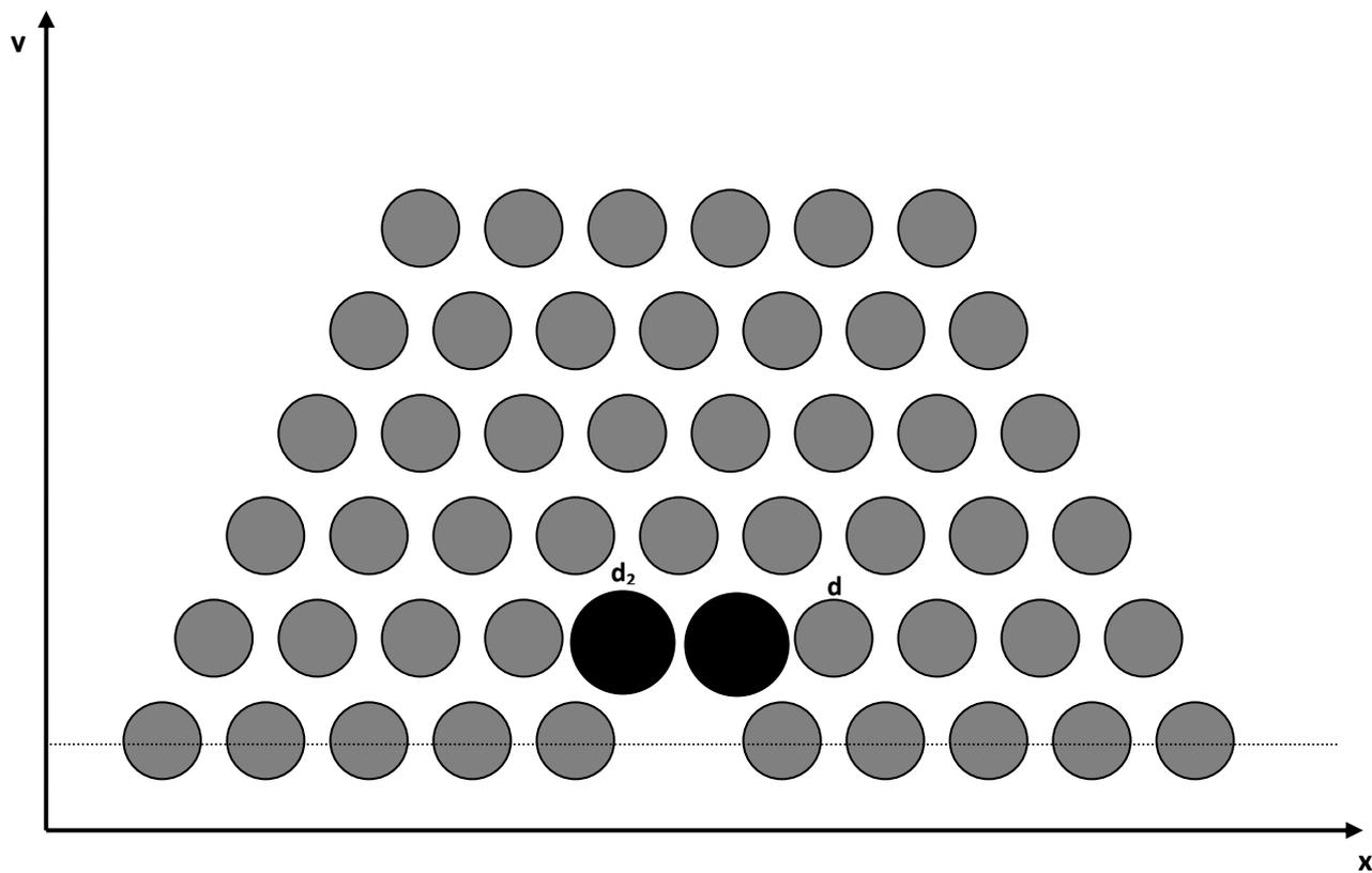
Fig. 5. 3: A graph depicting half of the cross-section of a PCF;  $d \neq d_2$
