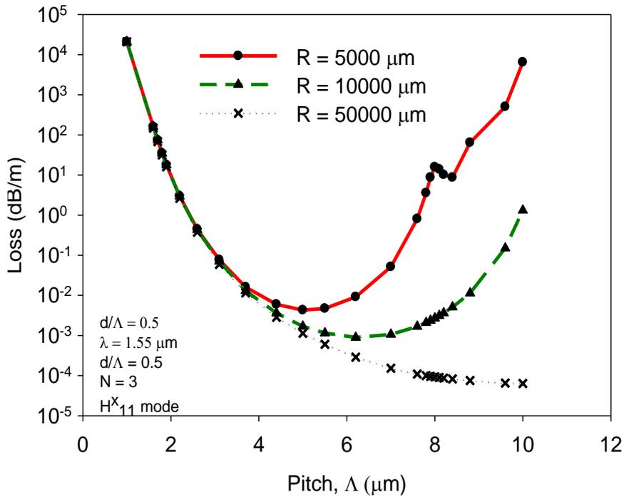
Fig. 4. 11: Variation loss with the pitch lengths for R = 5000μm, 10000μm and 50000μm
