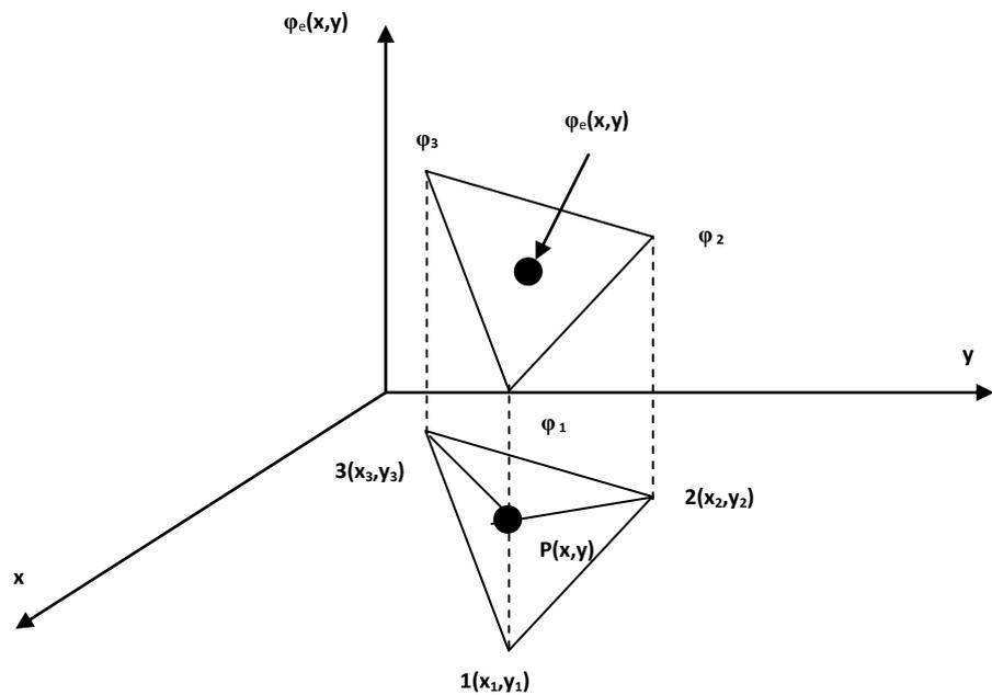
Fig. 3. 6: Representation of a first order triangular element.
