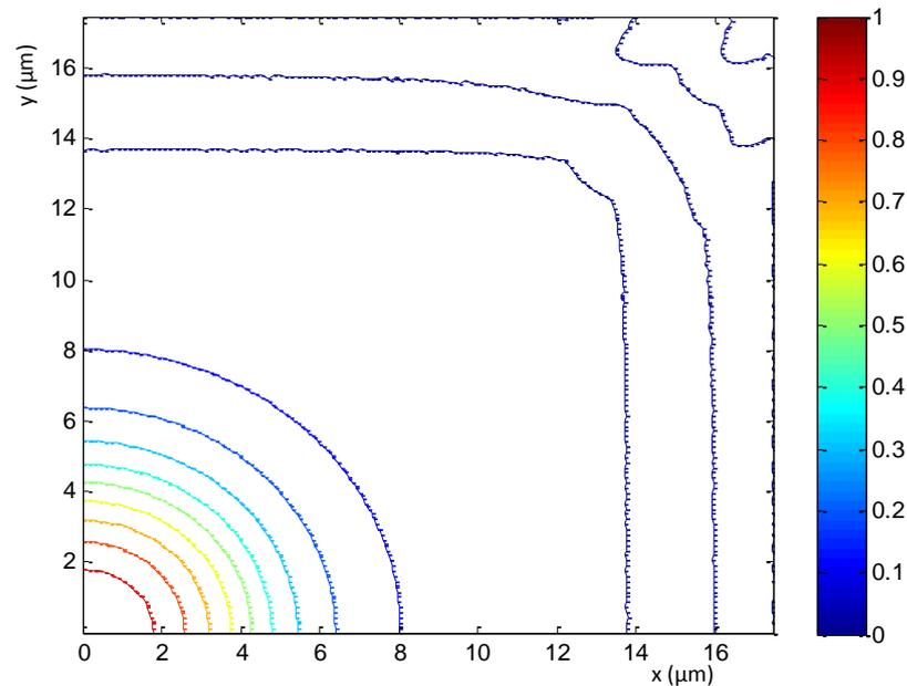
Fig. 6. 2: 2-D  $H_x$  field profile for a Single Mode Fibre exploiting 2-fold symmetry with only quarter of the structure simulated.
