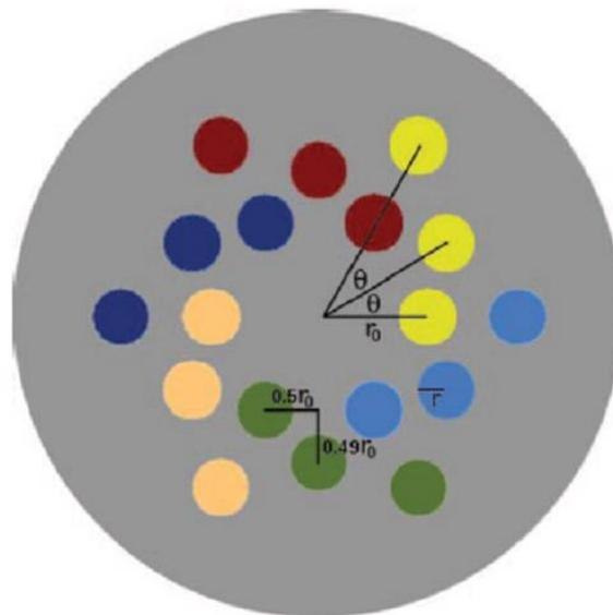
Fig. 7. 11: Schematic of the ES-PCF structure
