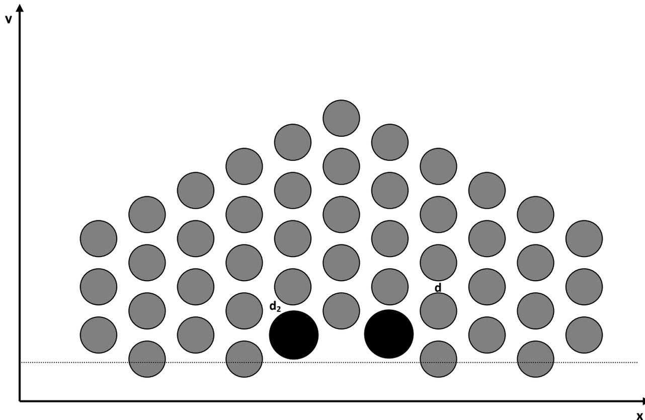
Fig. 5. 4: A graph depicting half of the cross-section of a PCF;  $d \neq d_2$ , same as shown in Fig. 5.3 but with a 90 degree rotation.
