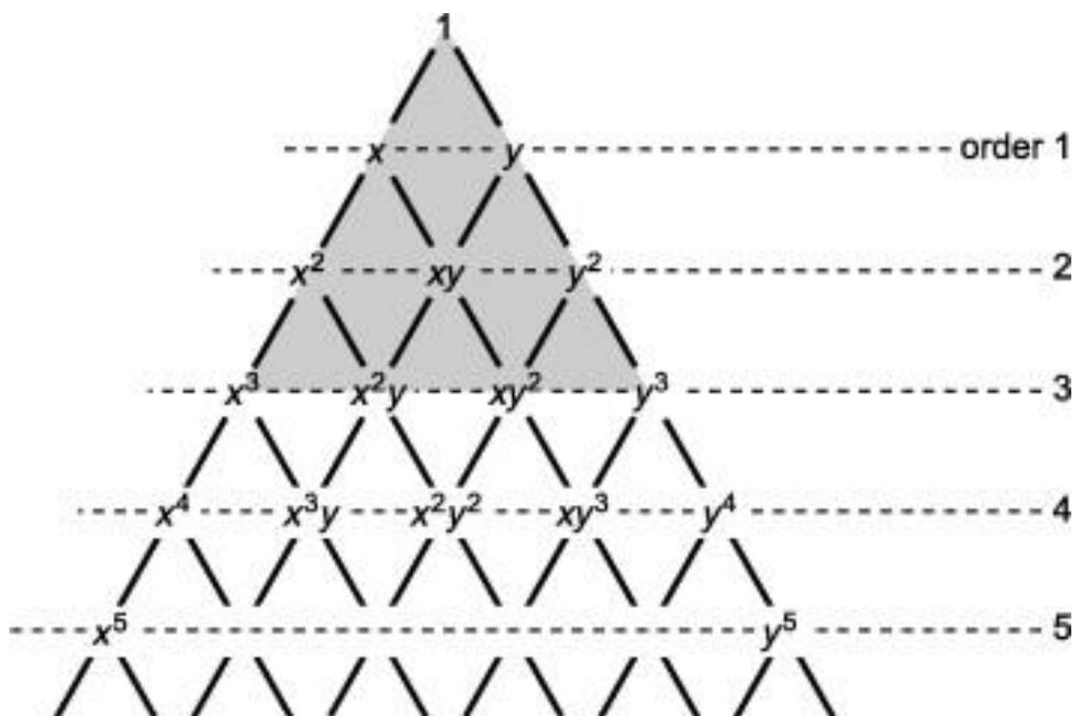
Fig. 3. 5: Pascal’s triangle for complete polynomials in two dimensions.
