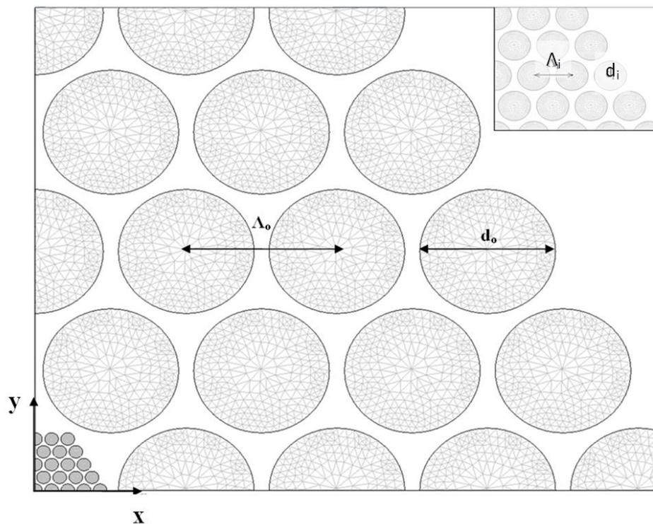
Fig. 7. 24: Representation of the porous core PCF cross-section with  $N_{\text{core}} = 4$ ,  $N_{\text{clad}} = 4$ .  $\Lambda_o =$  outer pitch and  $d_o =$  outer radius. Inset shows  $\Lambda_i =$  inner pitch and  $d_i =$  inner radius.
