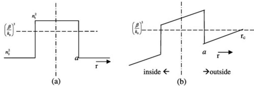
Fig. 2. 6: Refractive index profile of bent PCF. (a) straight fibre; (b) a bent fibre with the centre located at the side of 'inside'(Xiangru *et al.* 2010)
