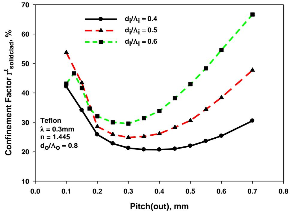
Fig. 7.33: Variation of the confinement factor in the core air-holes,  $\Gamma_{\text{solidclad}}^{\text{clad}}$ , with the outer pitch  $\Lambda_o$  for  $d_o/\Lambda_o = 0.8$  but with different  $d_i/\Lambda_i$  values.
