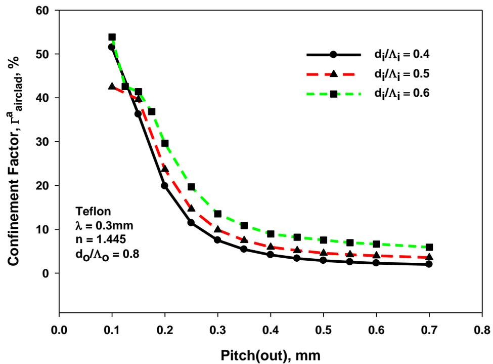
Fig. 7. 31: Variation of the confinement factor in the core air-holes,  $\Gamma_{\text{airclad}}^{\text{a}}$ , with the outer pitch  $\Lambda_o$  for  $d_o/\Lambda_o = 0.8$  but with different  $d_i/\Lambda_i$  values.
