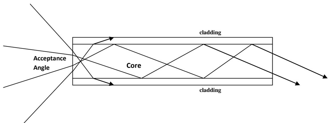
Fig. 1. 3: The propagation of light through a multi-mode optical fibre
