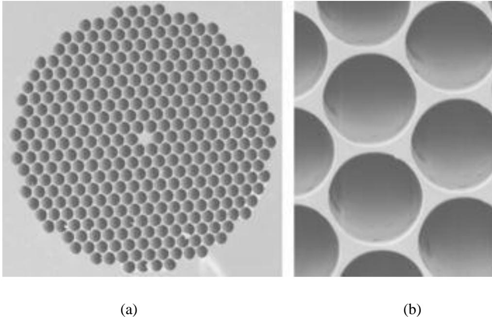
Fig. 2. 1: SEM micrographs of a photonic-crystal fibre produced at US Naval Research Laboratory. (a) The diameter of the solid core at the centre of the fibre is 5  $\mu\text{m}$ , while (b) the diameter of the holes is 4  $\mu\text{m}$  (Image of Photonic Crystal Fibre from NRL 2006).
