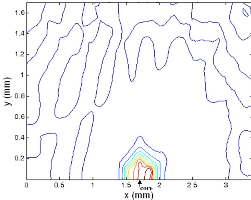
Fig. 7. 39:  $H_x$  field profile of the bent PCF for the fundamental  $H_{11}^x$  mode for bending radius, 1.5 cm.
