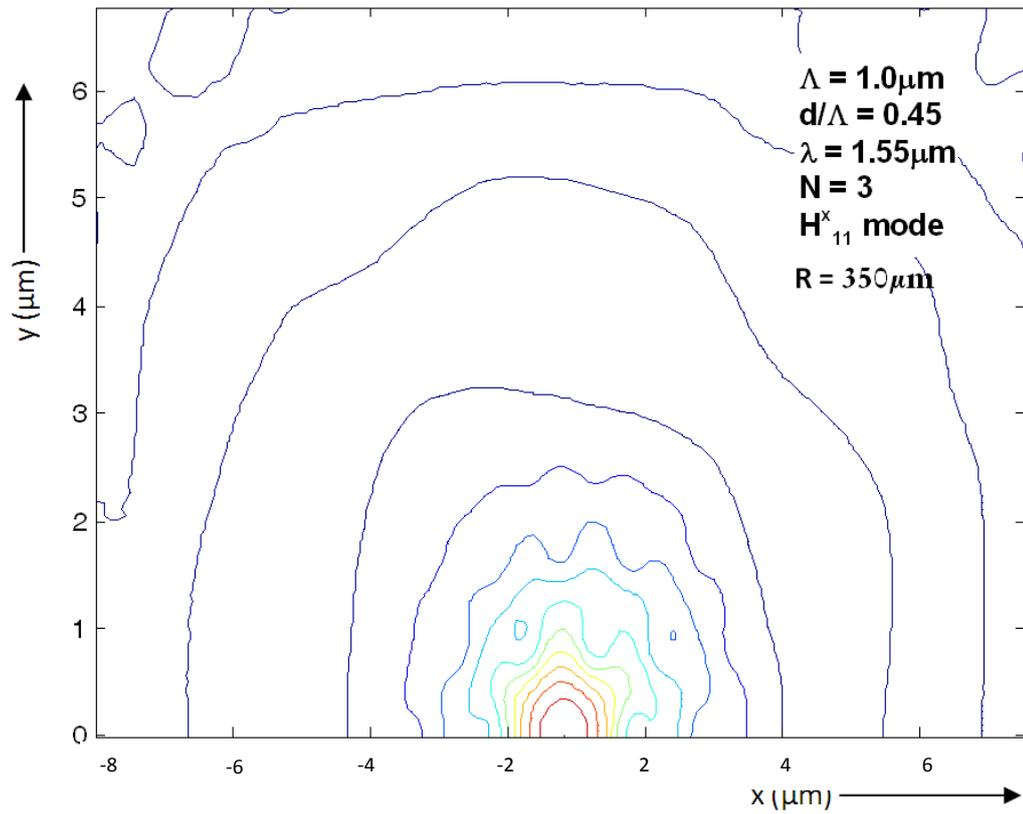
Fig. 4. 14:  $H_x$  field profile of the  $H_x^{11}$  mode  $R = 350\mu\text{m}$ ,  $\Lambda = 1.0\mu\text{m}$ ,  $d/\Lambda = 0.45$
