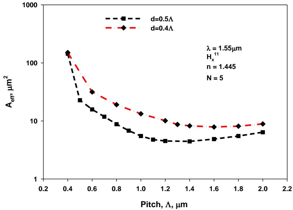
Fig. 6. 9: Variations of the  $A_{\text{eff}}$  with the pitch length for PCF having  $d/\Lambda = 0.4$  and  $0.5$  for  $N = 5$  with all air-holes equal.
