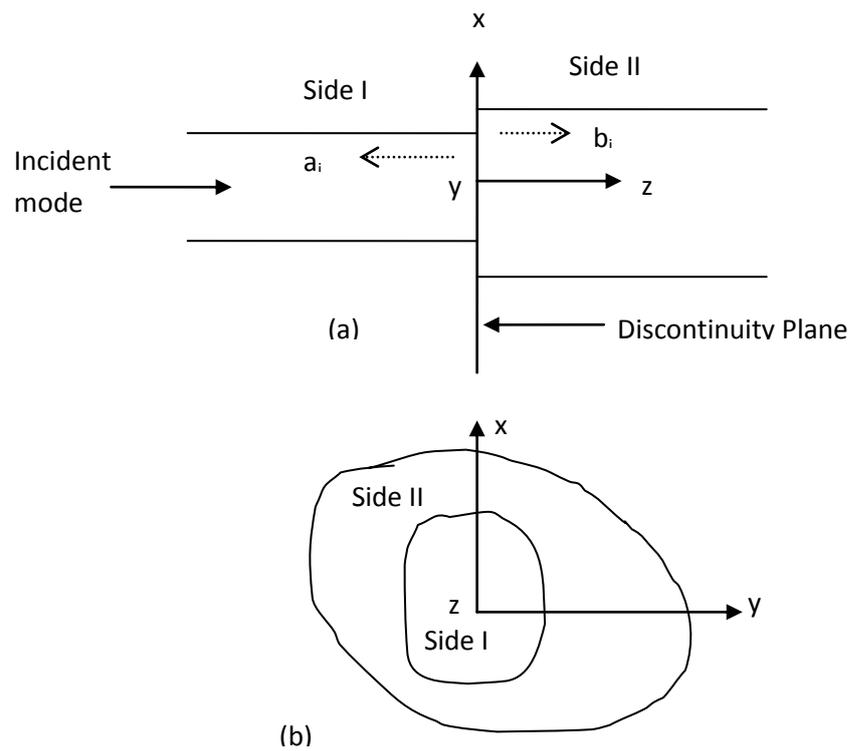
Fig. 3. 8: Discontinuity junction of two dielectric waveguide (a) vertical section of the discontinuity between side I and II (b) Transverse cross section of the discontinuity at the junction of two sides.
