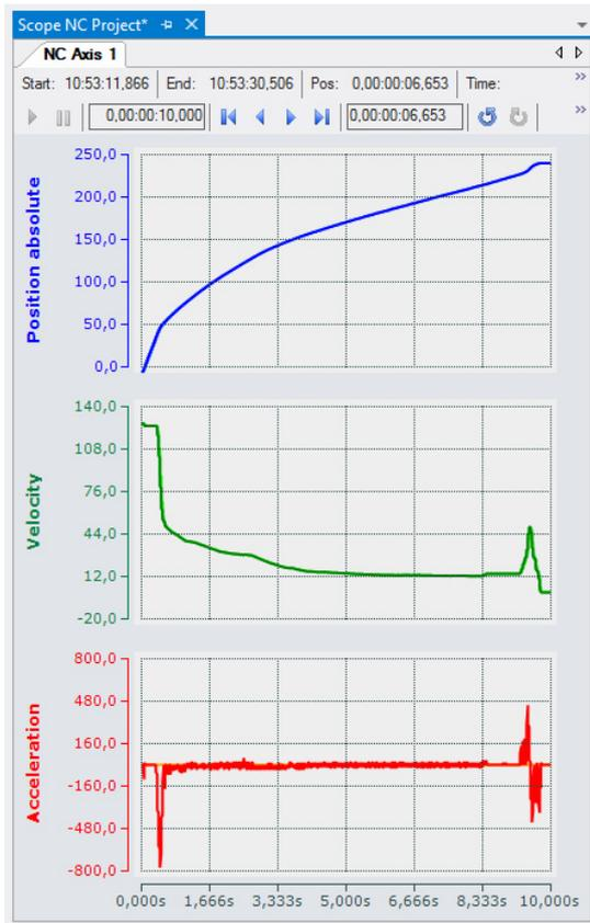
Fig. 6. Optimal control strategy (screenshot from the TwinCAT® control process environment; position x of the cutting head in [mm], velocity in [mm/s] and acceleration in [mm/s<sup>2</sup>])
