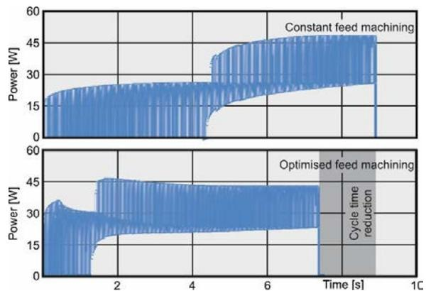
Fig. 7. Initial and optimized required power
