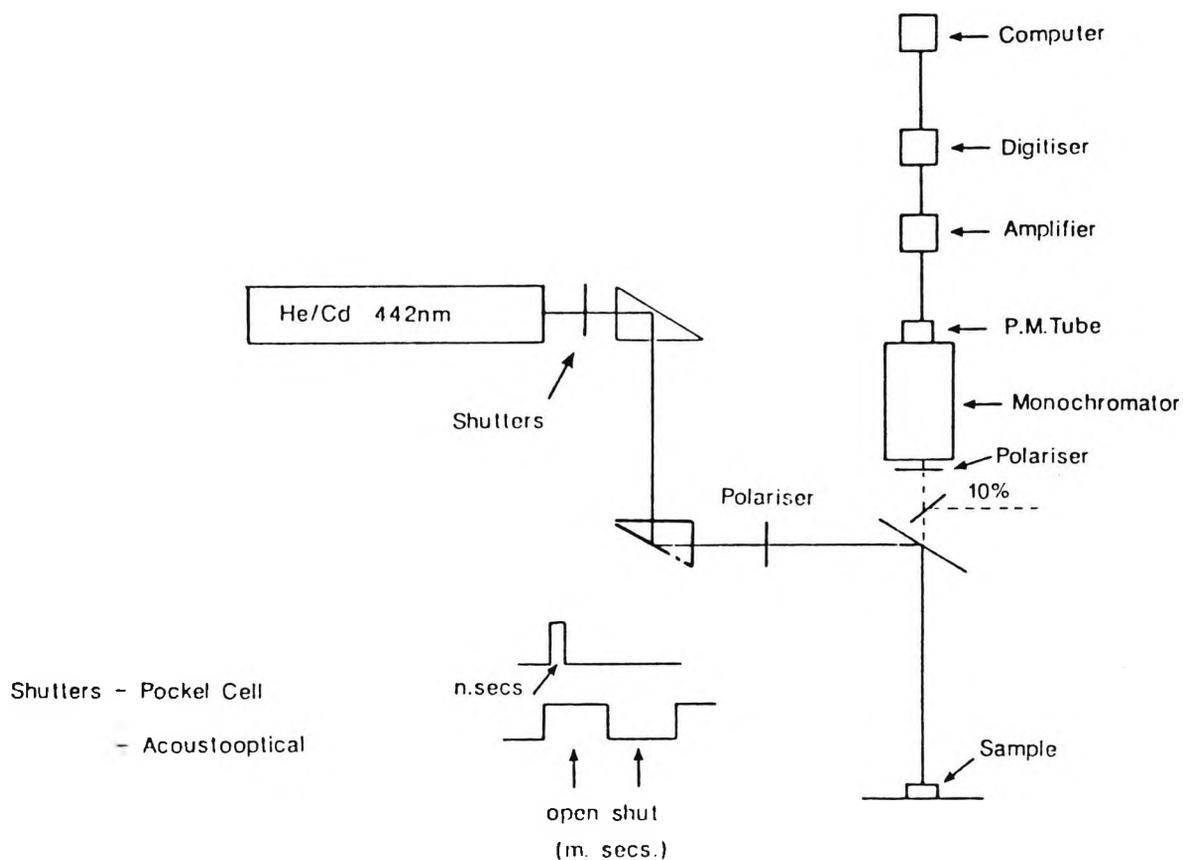
The microscope was a Carl Zeiss LAB 16 fluorescence microscope with a 40/0.75 Neofluar objective. The helium-cadmium laser, model 4240NB was made by Liconix, Sunnyvale, USA. The wavelength of the light was 442 nm and had a power output of 50 mW. The laser was gated by
