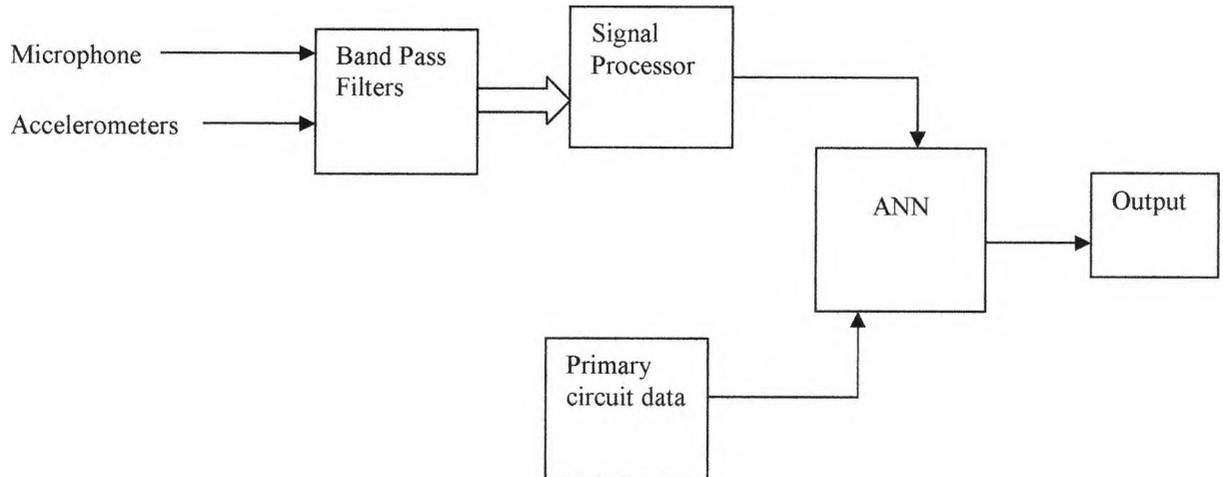
**Figure 6.24 Possible acoustic Neural Net Monitor**
