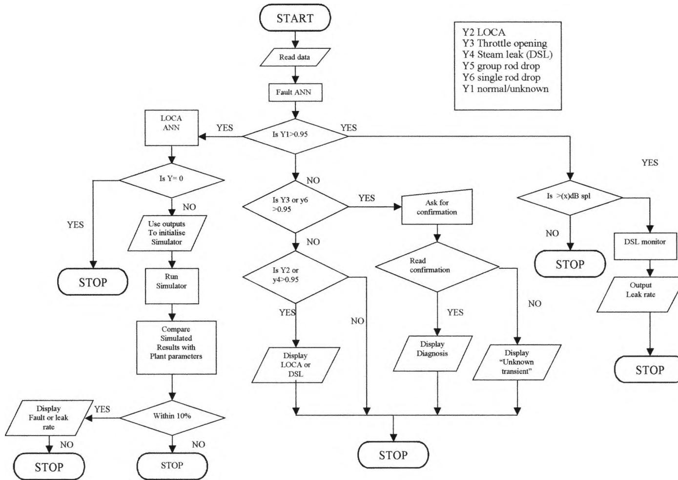
The overall performance of the OAS was very good. The prototype OAS was able to identify all major fault transients quickly and accurately (ANN output > 0.95) when tested on an independent data set. Plant operators are required to confirm the diagnosis for two of the transients (single and group rod drop). The inclusion of the plant operator interaction in the decision making process may be beneficial to the successful implementation of the OAS.
