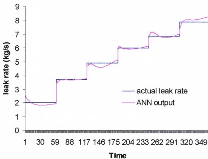
Figure 7.6 Estimation of large size leak rates
