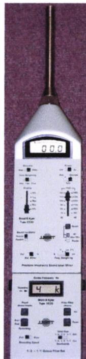
Figure 6.7 B&K 2260 with 1/3 octave filter
