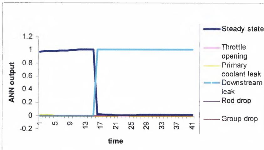
Figure 4.5 downstream leak at 60% full power
