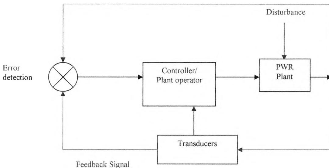
**Figure 3.5 Block Diagram of a control system**
