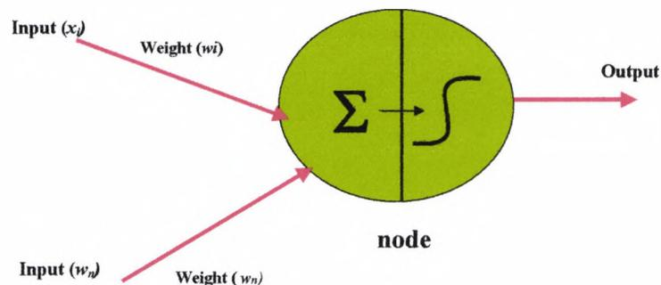
In supervised learning, the ANN the topology is usually held fixed, and the Connection weights are changed during training to minimise error between actual and desired output data.
