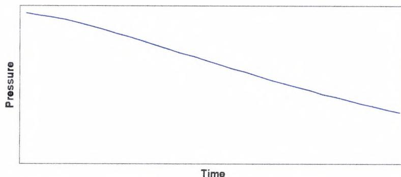
Figure 4.3 Pressuriser change for rod drop at 30 % power
