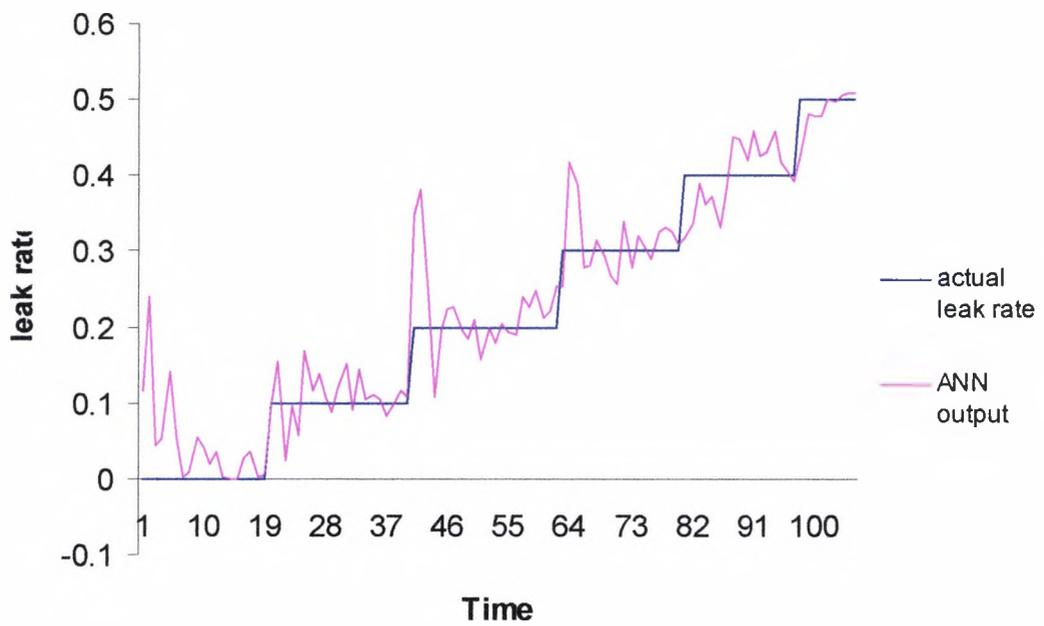
**Figure 5.13 ANN results for classification of leak rate (10 times step, 1% noise)**
