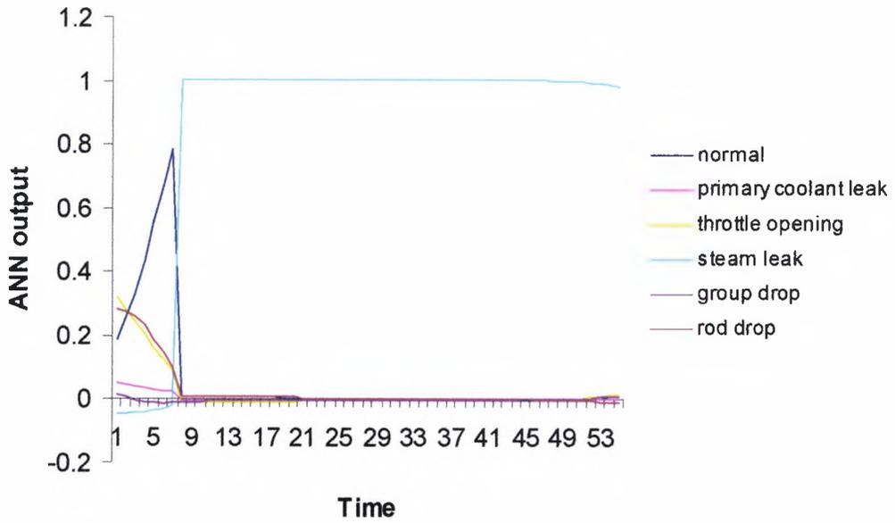
Figure 4.17 Steam Leak Transient
