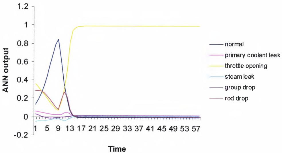
Figure 4.16 Throttle Opening Transient
