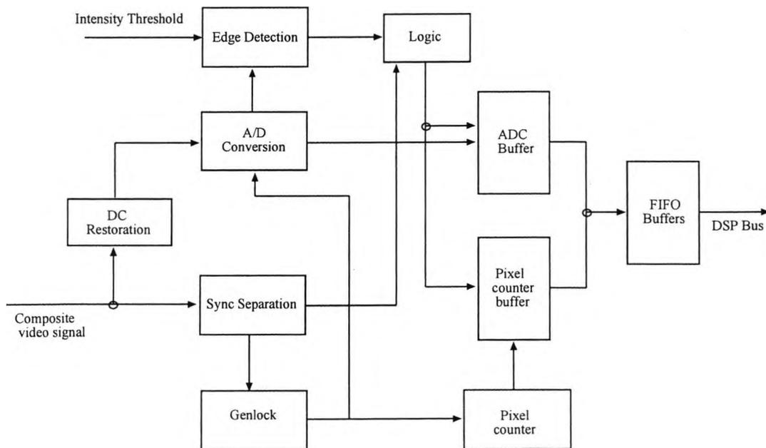
Figure 6.4 Block diagram of the video processing module
