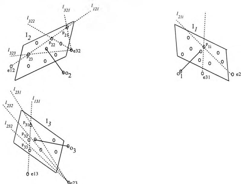
Figure 3.10 Intersection of epipolar lines on third view
