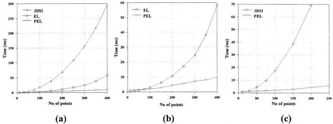
**Figure 4.14 Speed performance of algorithms at stereo pair level with performance improved *PEL* algorithm**
