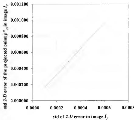
**Figure 5.13 Variation of  $\sigma_l$  for various values of  $\sigma$  for a single point**
