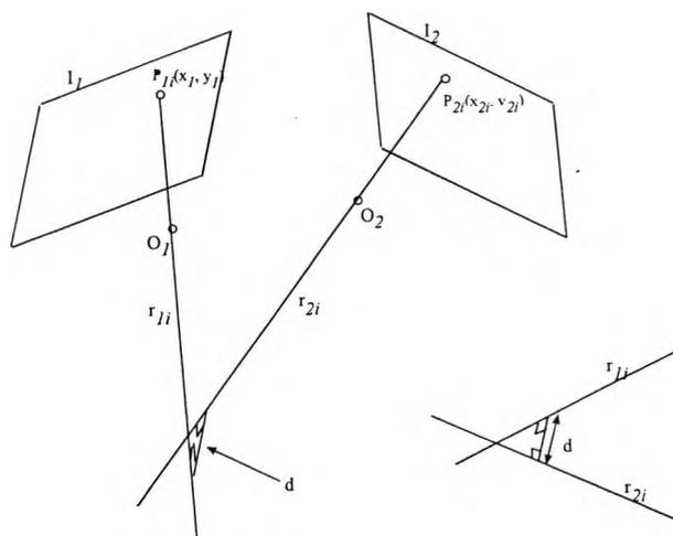
Figure 3.11 Minimum distance between a pair of rays
