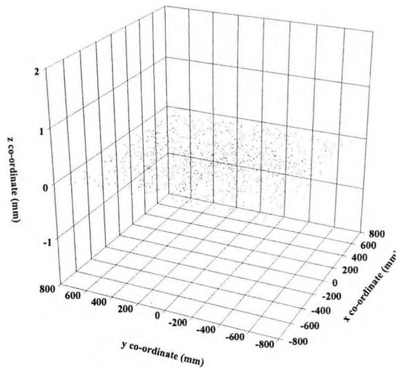
Figure 5.16 3-D reconstruction of planar target field
