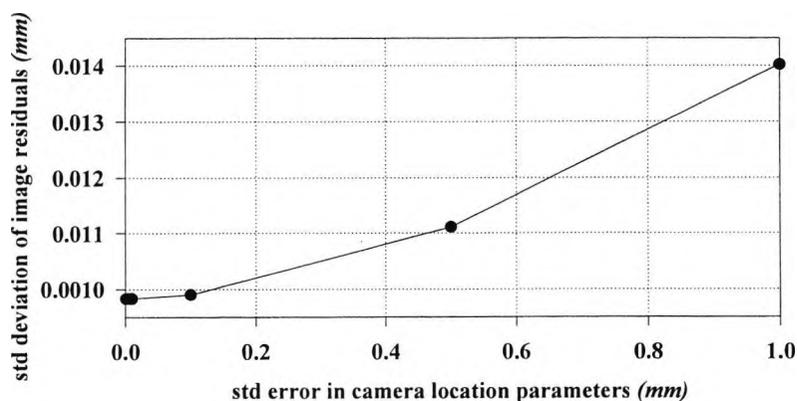
(a). std error in rotation parameters and 2-D image points = *0.01 degrees*,
