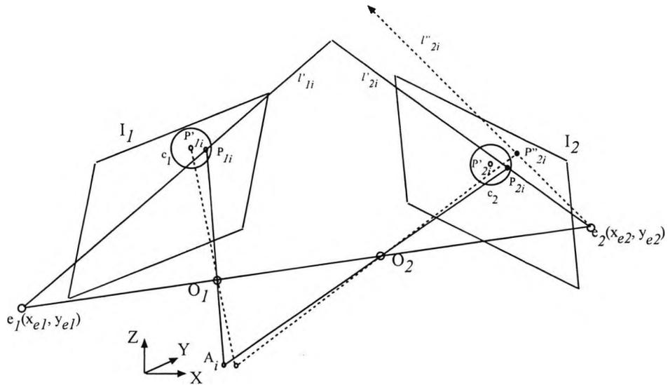
**Figure 5.11 Effect of 2-D residual on epipolar constraint**
