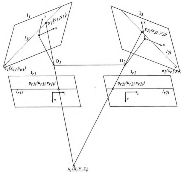
Figure 4.3 Convergent and corresponding rectified image pairs
