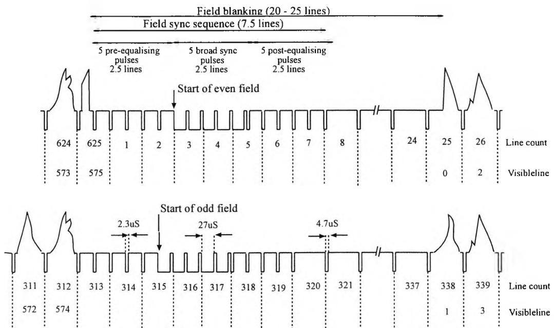
Figure 6.6 Odd and even field synchronisation (CCIR)
