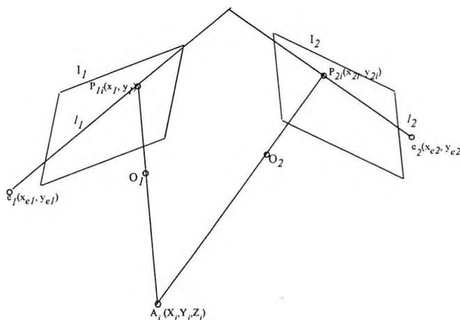
Figure 3.2 Epipolar geometry
