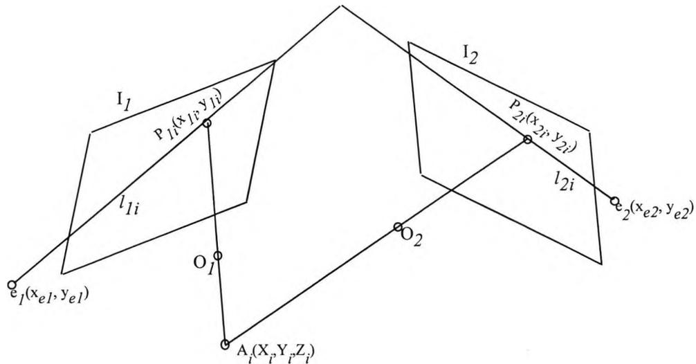
Figure 1.1 Epipolar geometry
