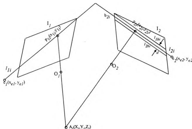
Figure 4.1 Application of epipolar constraint in image space
