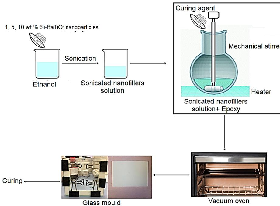
**Figure 4.** Schematic diagram of the preparation of Epoxy/Si-BaTiO<sub>3</sub> nanocomposites.
