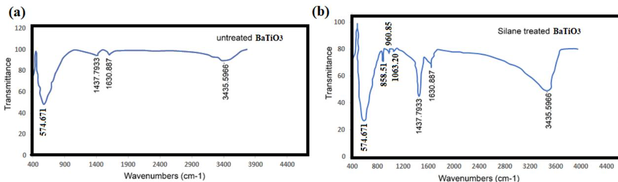
**Figure 3.** FTIR spectra of unmodified BaTiO<sub>3</sub> and modified BaTiO<sub>3</sub>, a) unmodified BaTiO<sub>3</sub>, b) modified BaTiO<sub>3</sub> (Si-BaTiO<sub>3</sub>).
