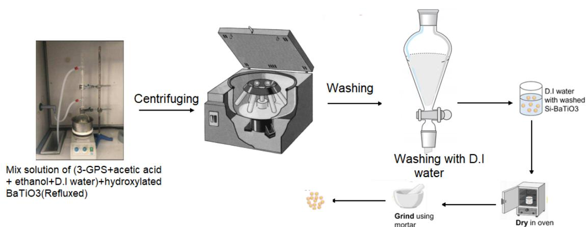
**Figure 2.** Schematic diagram of the functionalisation process of BaTiO<sub>3</sub> with 3-GPS. The epoxy nanocomposite fabrication process including Si-BaTiO<sub>3</sub> functionalisation is schematically illustrated.
