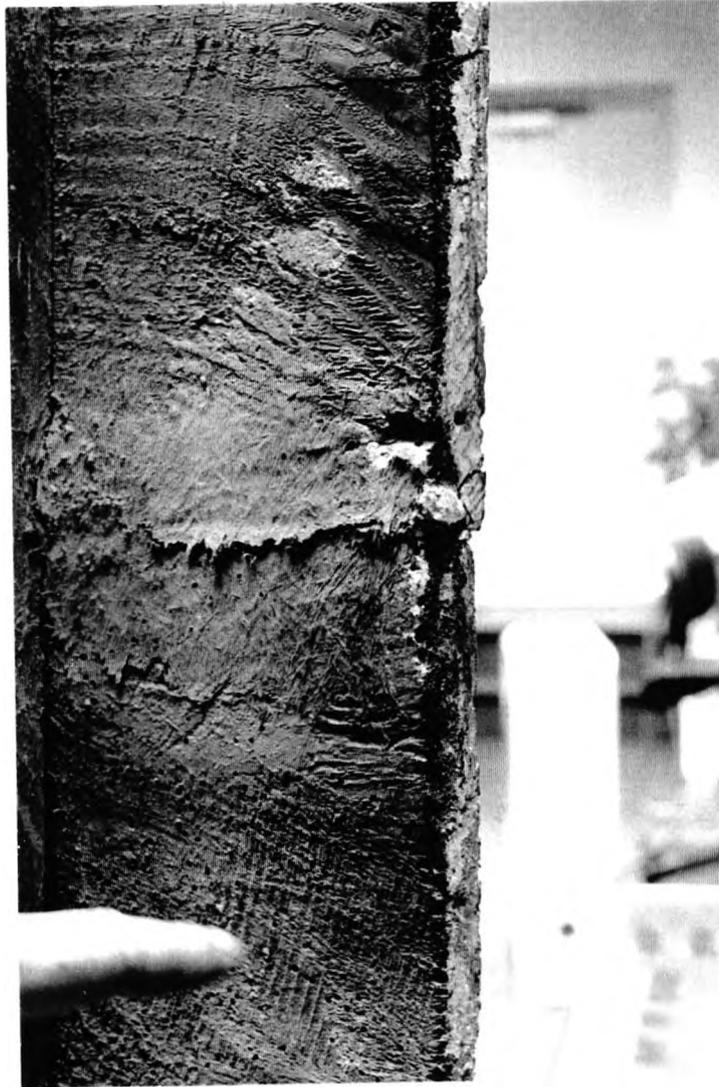
Figure 5. Original fixed battens on a 15th c. Spanish panel: Detail, transverse-grain edge at one side showing a split (top), a disjoin beneath an original fibre/gesso layer (middle), and a cupped warp in the lower plank, shown by the shadow along the batten at left.
