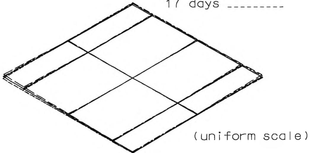
Figure 42. Isometric view from the top of an oak panel with sliding flexible battens showing changes in shape from dry to moist conditions. Note similar pattern over and between battens.
