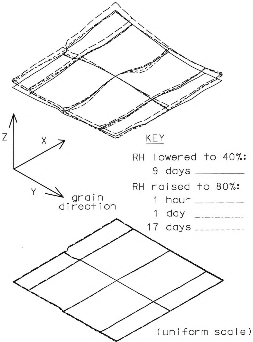
Figure 41. Isometric view from the top of an oak panel with sliding rigid battens showing changes in shape from dry to moist conditions. Note exaggerated warp in the free area between the battens.
