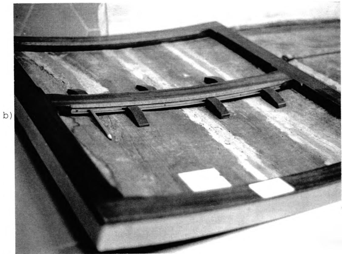
Figure 12. Rigid reinforcements which slide on roller-bearings: a) wooden battens with metal U-section runners on a thicker panel, b) a "chassis cadre" with cross member on a thinner panel in which the members lying across the panel grain are cut to approximate permanent warp.
