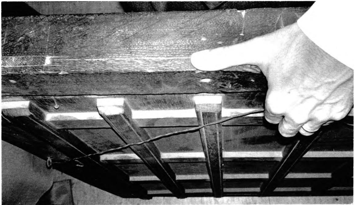
Figure 23. A cradle with flexible sliding members which have partly conformed to the panel's convex warp.
