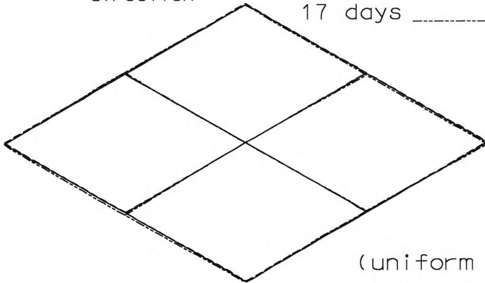
Figure 46. Changes in shape of a poplar panel laminated with medium density fibreboard (MDF) in going from dry to moist conditions.
