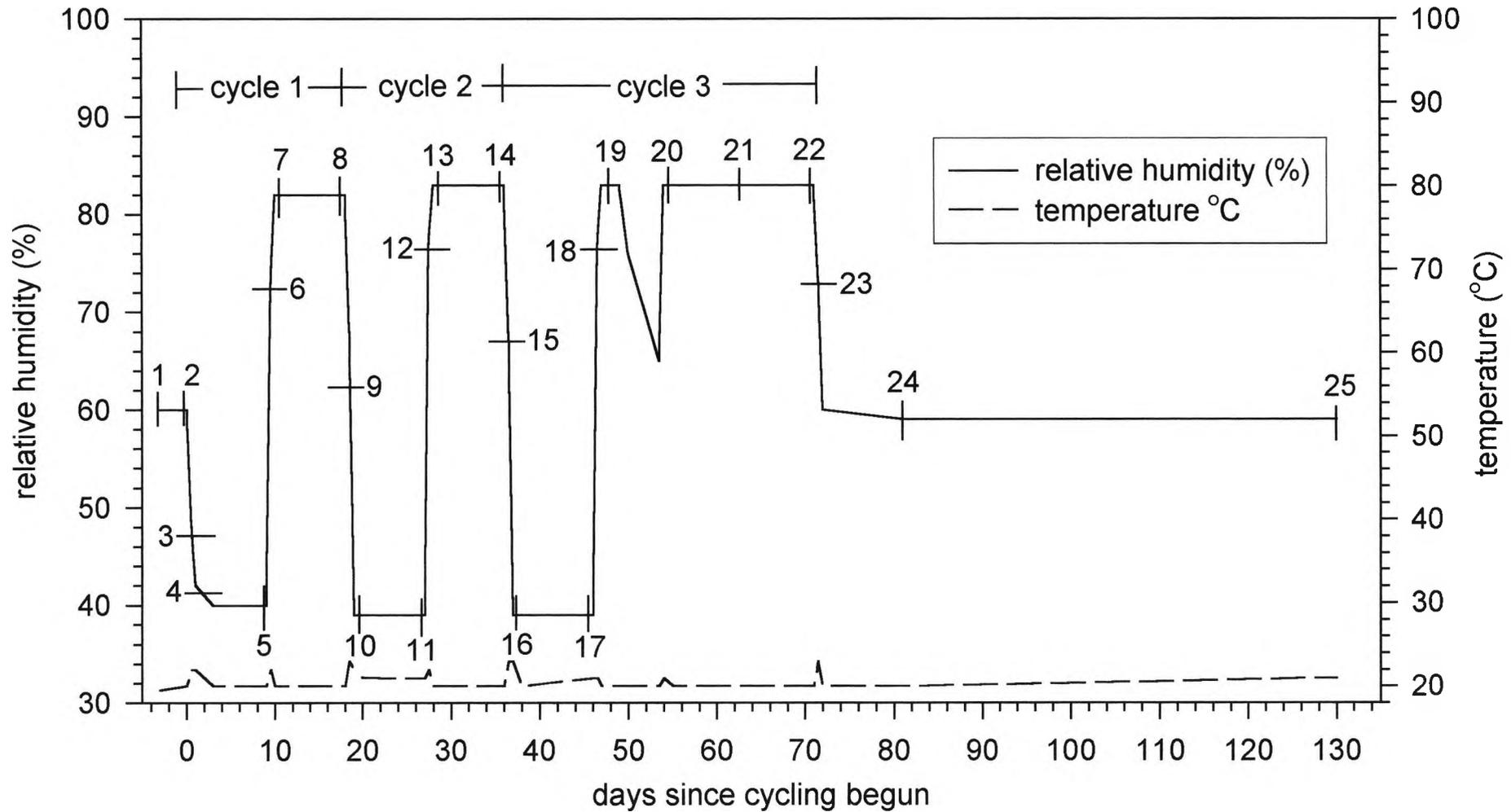
Figure 30. Relative humidity (RH) and temperature changes during the study: cycles numbered at the top, measurement epochs numbered along the humidity trace. RH fell temporarily in cycle 3 due to humidifier malfunction.
