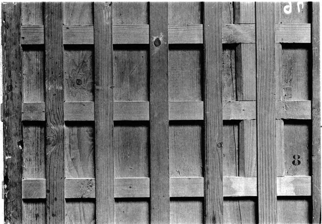
Figure 24. Splits in tangentially cut areas of a softwood panel with a relatively flexible cradle: a) one visible in panel lower half, just right of middle and b) (detail) another at upper left (Eustache Le Sueur, "La Naissance de l'Amour", 1820X1250X4mm, Louvre INV8050.) Photos Laboratoire de Recherche des Musées de France (1957).
