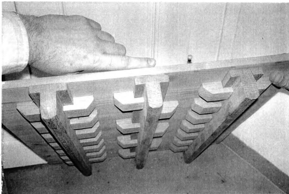
Figure 11. Panel/reinforcement mock-ups used to test sliding batten designs, from Münster, Germany: a) rectangular section aluminium battens, b) wooden T-section battens, similar to those used by Wehlte.
