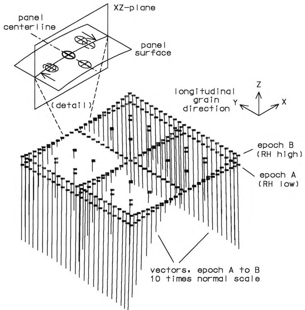
Figure 32. Panel front, isometric view from above showing shape (normal scale) and 10X vectors of 3-dimensional movement between two measurement epochs. Schematic detail shows irregularly-placed targets (circles) graphically constrained (dashed circles) to the vertical XZ-plane.
