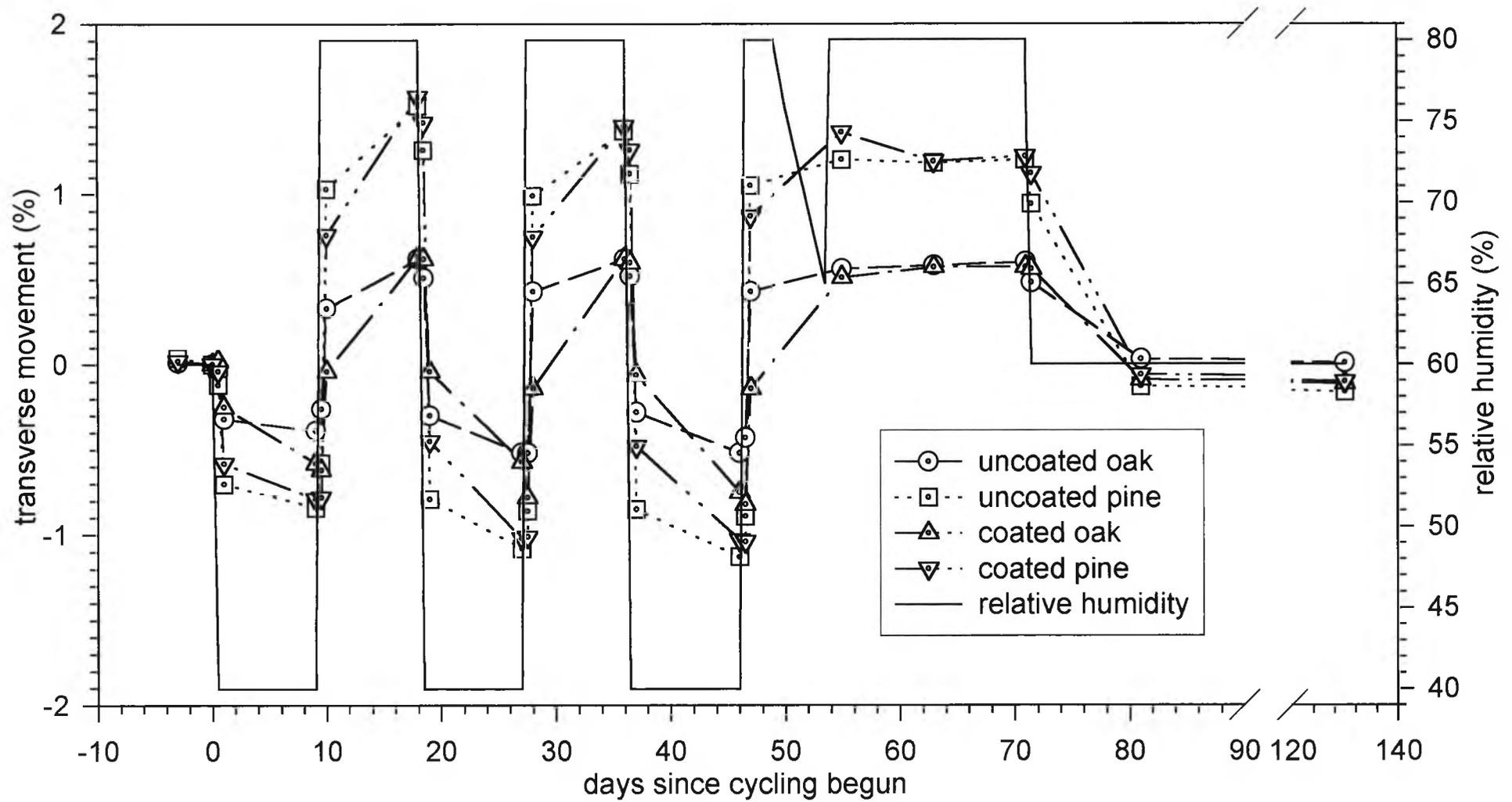
Figure 34. Transverse movement at panel centreline for uncoated and coated oak and pine over the entire study period.
