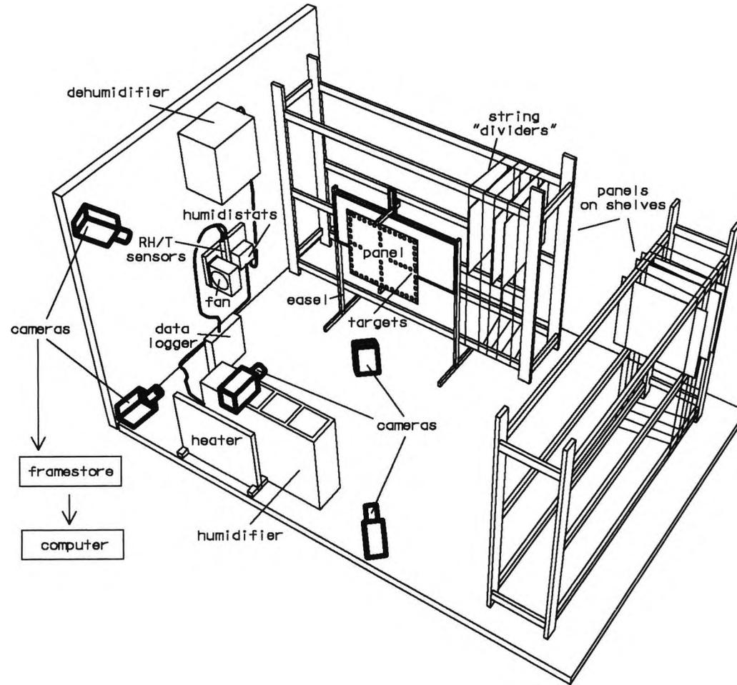
Figure 29. Elevated perspective view of the controlled environment room. A panel is on the easel to be recorded by the five wall-mounted digital cameras.
