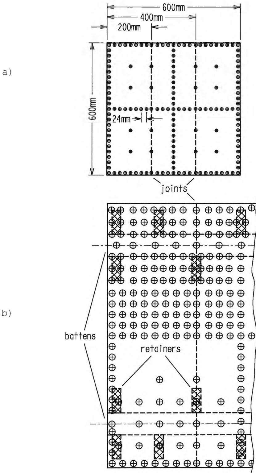
Figure 31. Panel front showing target patterns: a) assuming relatively uniform movement overall, and b) left half and upper quadrant, assuming local deformations near battens (centrelined) and their retainers (crosshatched).
