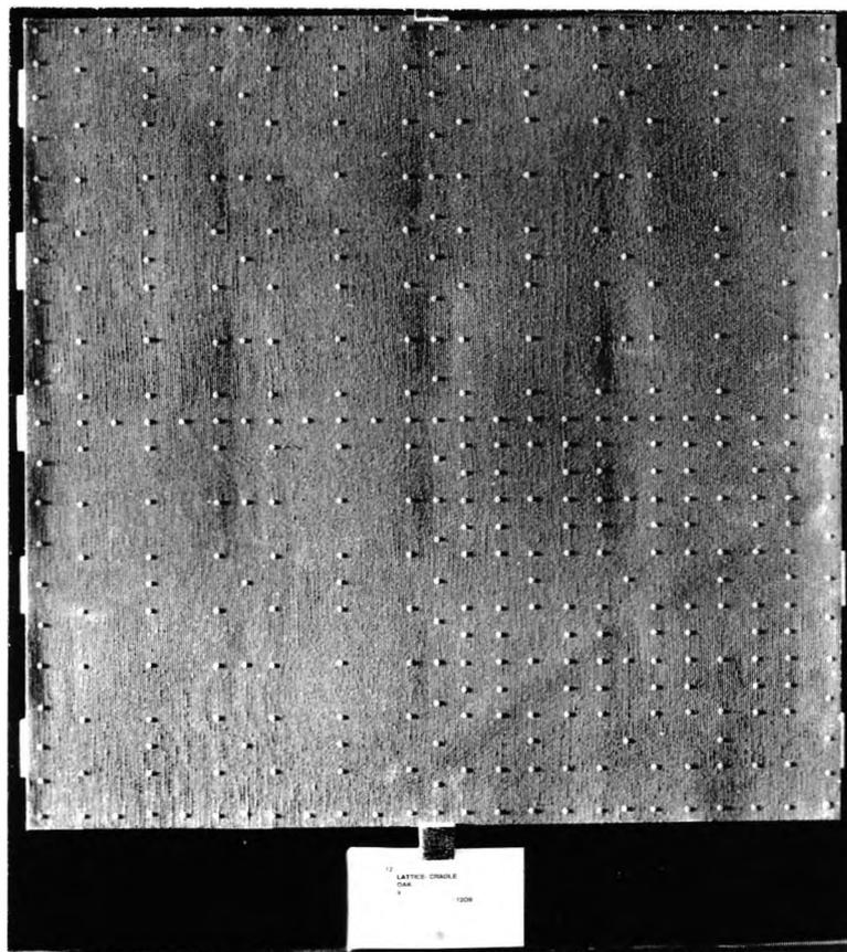
Figure 44. A cradled oak panel in raking light showing distortions around glued areas of fixed members immediately after cradle application.
