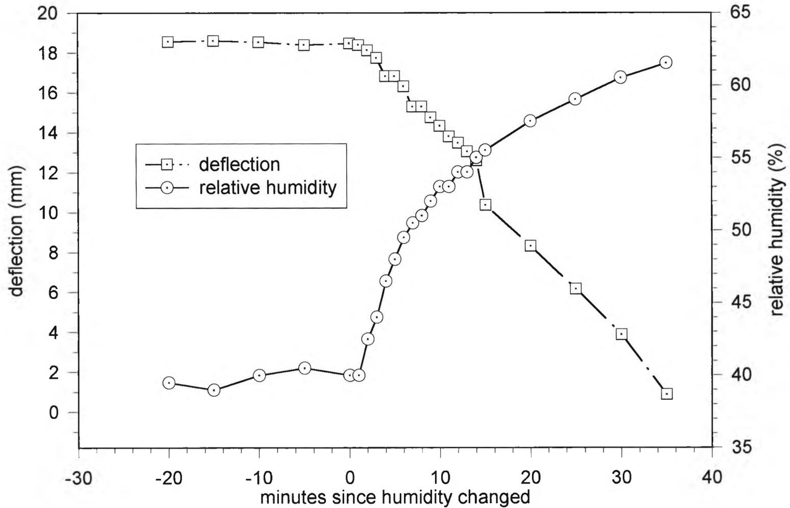
Figure 35. Warp response of coated oak during a change toward higher relative humidity.
