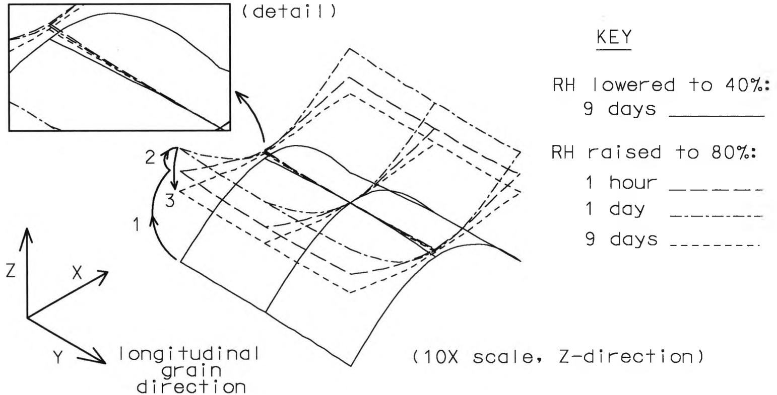
Figure 36. Sequence of warp movement in a coated poplar panel 10mm thick during a rise in relative humidity: isometric view of the front from above with warp (scale in Z direction) exaggerated ten times and changes ordered 1-3. Detail shows warp in the longitudinal grain-direction.
