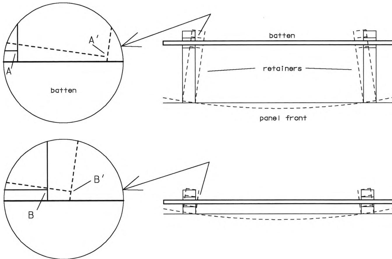
Figure 15. The effect of moving battens away from the panel back. The panel, face down, is shown before (solid lines) and after a convex warp (dashed lines). For battens retained further from the panel back (above), the contact surface moves a greater distance down and across (from A to A', detail at left) than it would for battens retained closer to the panel back (below and in detail, from B to B'). Thus battens retained further from the back will impede panel movement more easily.
