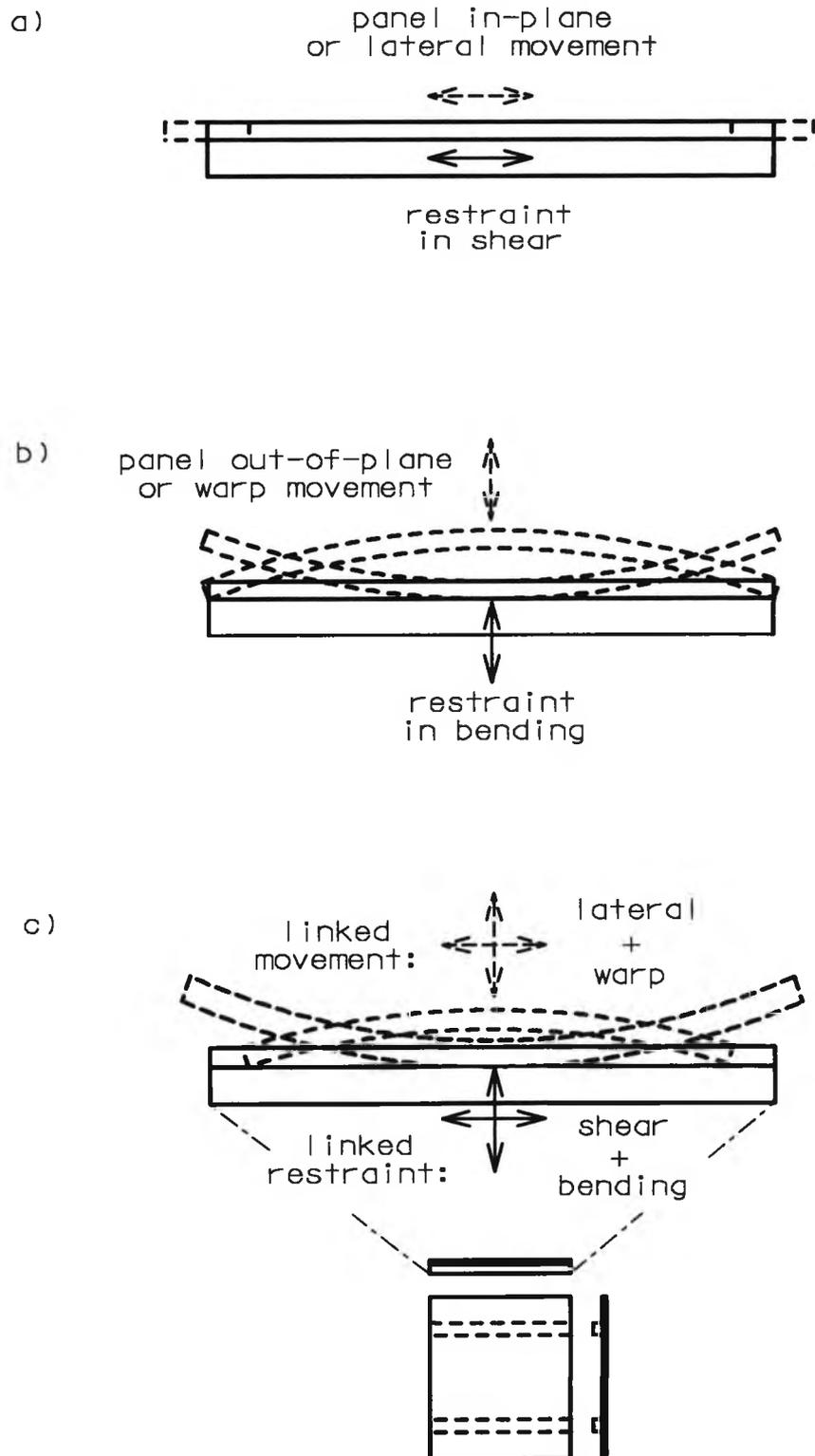
Figure 2. Movement and restraint in reinforced panels: a) in-plane, b) out-of-plane, c) combined.
