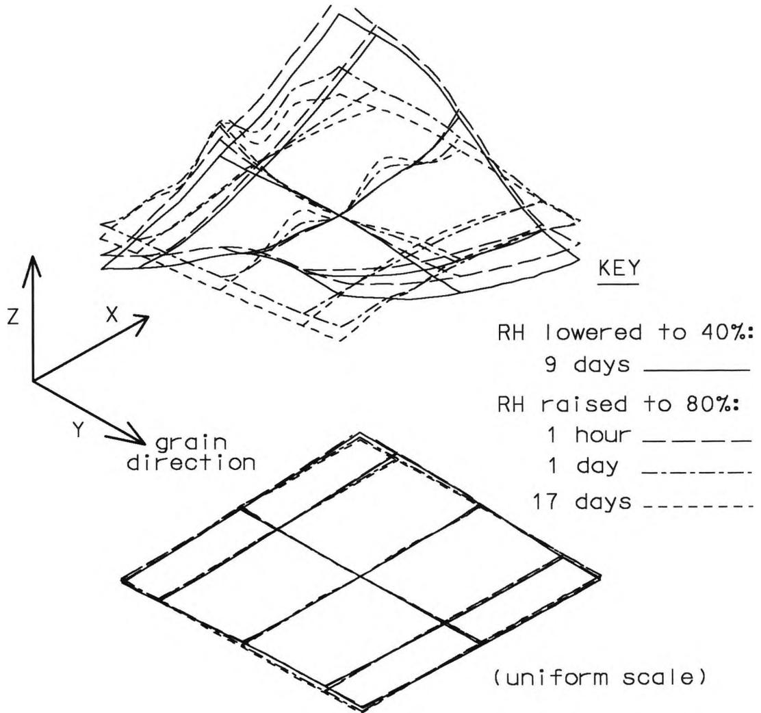
Figure 40. Isometric view from the top of an oak panel with fixed rigid battens showing changes in shape from dry to moist conditions. Note the twist, most evident in dry conditions.
