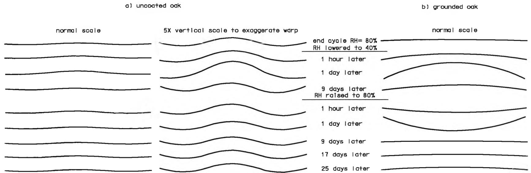
Figure 33. Transverse centreline profiles showing changes during a dry and then a moist period: a) oak, uncoated, b) oak, coated. The upper side is the coated side.
