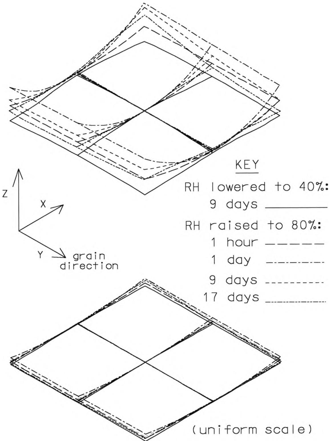
Figure 51. Changes in shape for an oak panel laminated with oak parquets, grain parallel to that of the panel, in going from dry to moist conditions.
