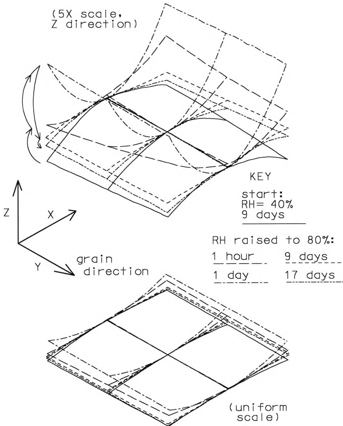
Figure 37. Coated oak, 3.30mm-thick, showing warp changes over the extended high-RH period.
