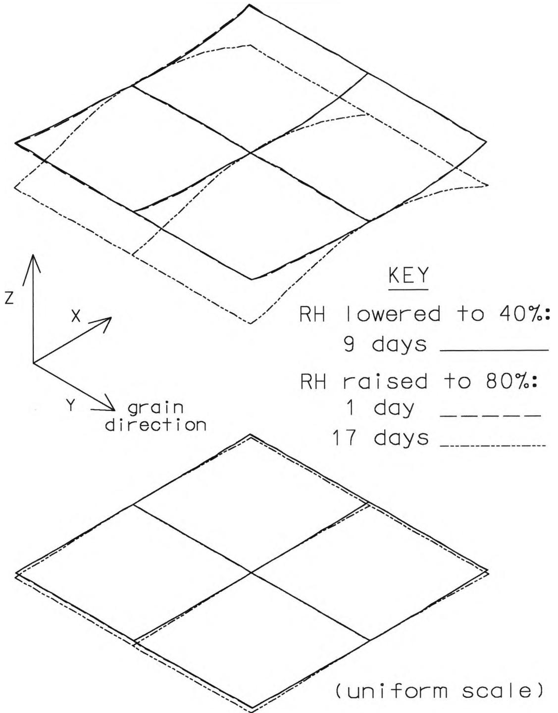
Figure 49. Changes in shape for an oak panel laminated with balsa blocks and wax-resin in going from dry to moist conditions.
