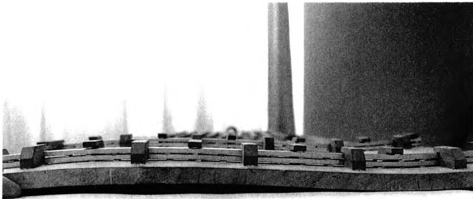
Figure 18. A model showing sliding flexible metal battens: a) viewed from the batten ends and b) from a transverse-grain edge showing the two layers of batten bent to conform to the panel curvature.
