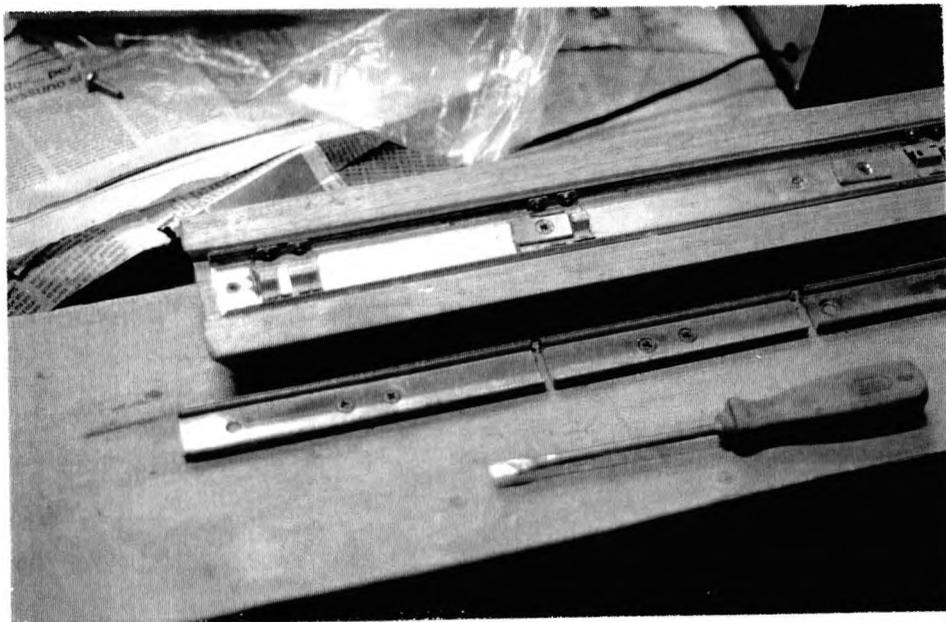
Figure 17. A rigid batten sliding on ball-bearing runners: the batten with outer track and ball-bearing cages is shown at the top, with below, sections of inner track which would be screwed to the panel back.
