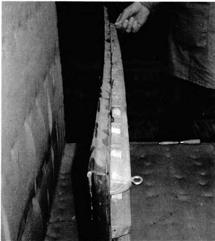
Figure 22. Panel deformation due to a cradle: out-of-plane bend parallel to the panel longitudinal-grain direction, viewed from above a longitudinal-grain edge.
