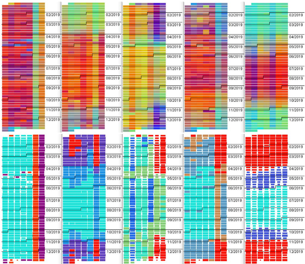
**Figure 8:** The time steps are represented by coloured bricks arranged in rows corresponding to the weeks and columns to days of the week. In the upper row of time arrangers, the bricks are coloured according to the positions of the time steps in the projections (Figure 7). In the lower row, the brick colours represent the cluster affiliations of the time steps.
