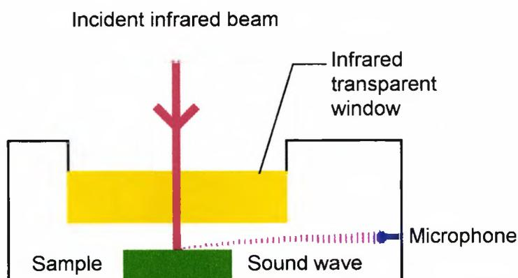
Figure 8.4.2. Schematic diagram of an infra-red photoacoustic cell
