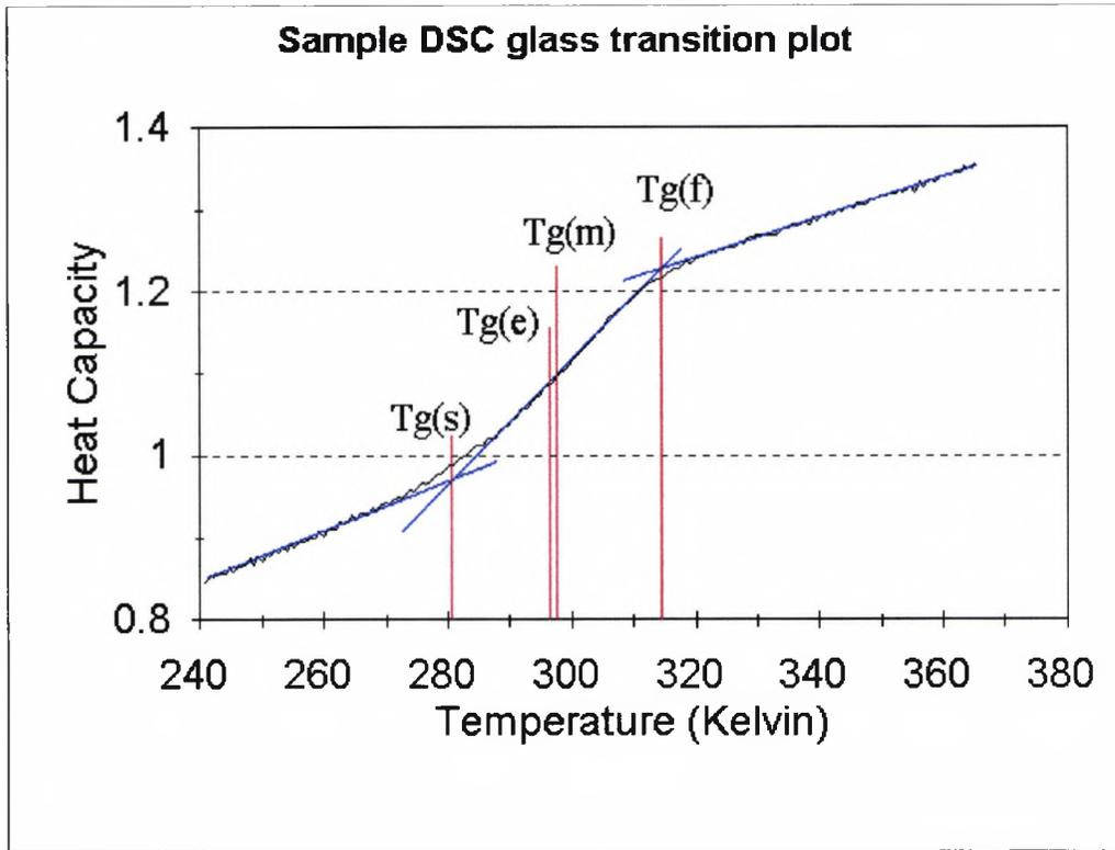
Figure 8.2. Glass transition plot of an unexposed traditional pigmented alkyd. The black trace is from the original data, blue lines are the intersection lines, and the red lines show the  $T_g$  s.
