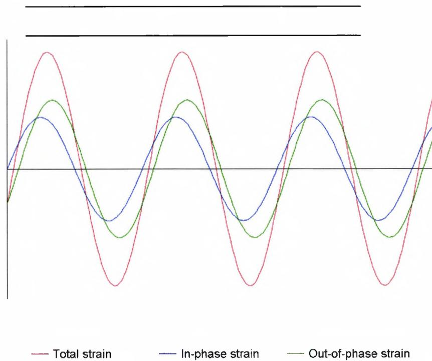
Figure 8.3.2. The strain can be deconvoluted into an in-phase strain and an out-of-phase strain (to the applied stress). The sum of the in-phase and out-of-phase strains is numerically equal to the total strain.
