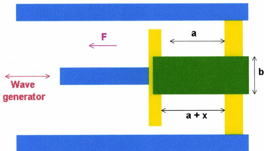
Figure 8.3.5. Schematic diagram of a DMTA tensile head. Measurements  $a$  and  $b$  are the dimensions of the polymer (shown in green) before pre-tension force  $F$  is applied, stretching the film by  $x$ . The amount of material in and beyond the clamps (shown in yellow) was assumed to have little effect on the value of the strain measured.
