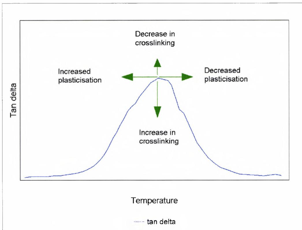
Figure 8.3.4. Plot illustrating how the shift in the maximum value of  $\tan \delta$  can yield information about the state of the polymer
