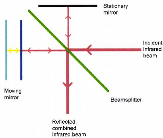
Figure 8.4.1.2. Schematic diagram of the optical arrangement. The moving mirror will cause individual wavelengths to interfere with themselves when the beam is recombined.
