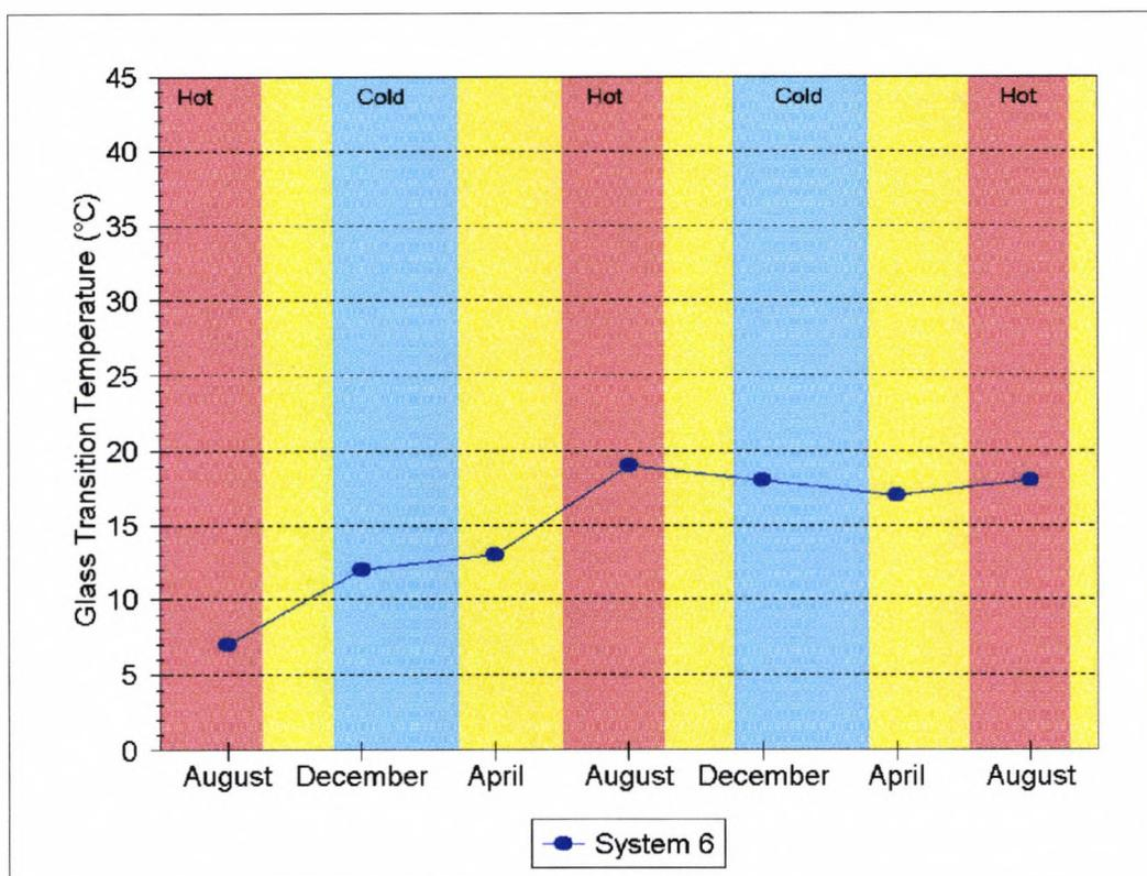
Figure 9.3.3. Variation of  $T_g$  of an alkyd-acrylic hybrid with month of measurement.
