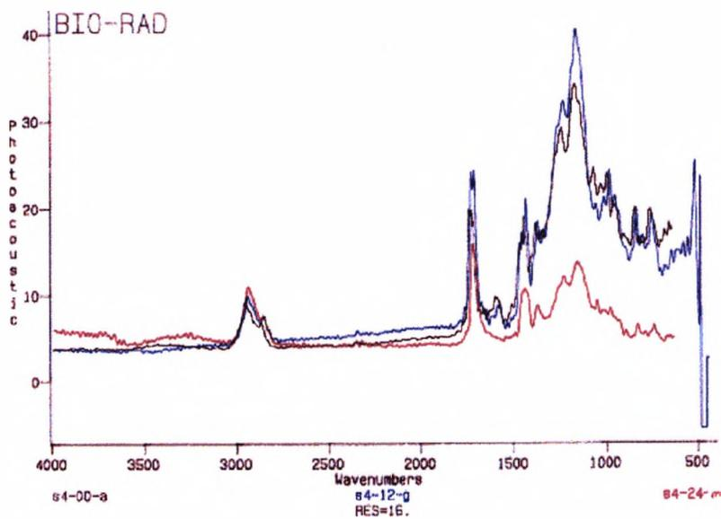
Figure 9.4.3.1. The effect of natural exposure on the infra-red spectra of System 4. The black, blue and red spectra are of the coating unexposed, and after 12, and 24 months respectively.
