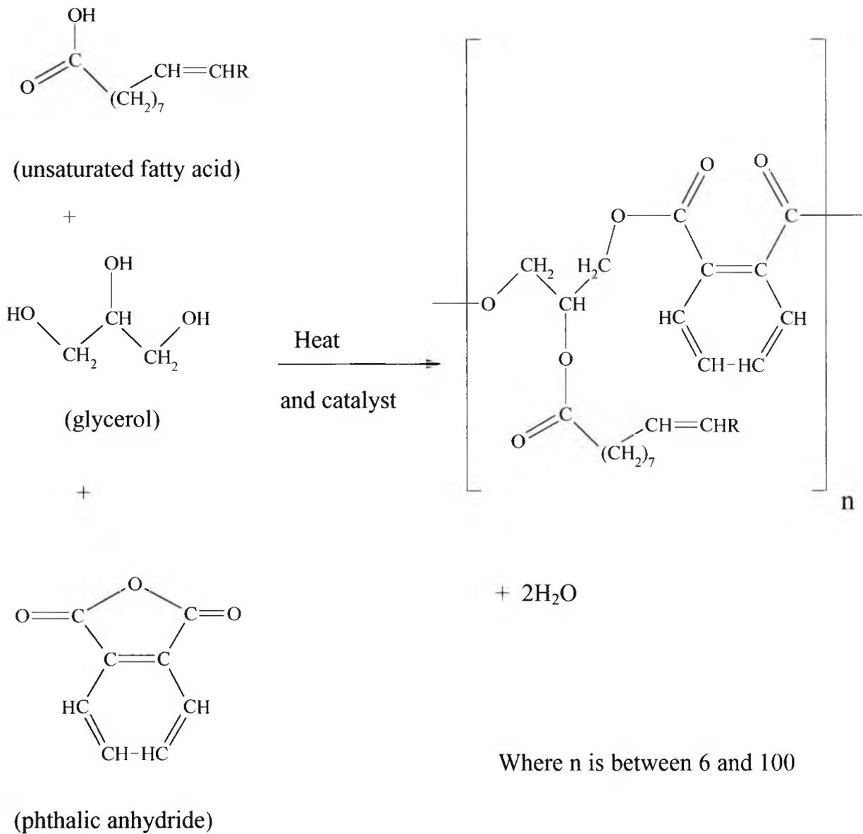
The second method is to react only the oil or fatty acid with the polyol first, to leave one or more hydroxyl groups, and then, in a second stage, reacting that ester with the polybasic acid.
