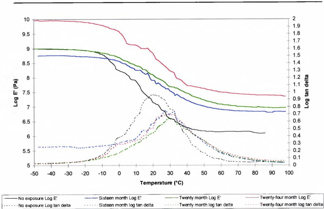
Figure 9.3.1.2.b. The effect of up to twenty-four months natural weathering on System 1
