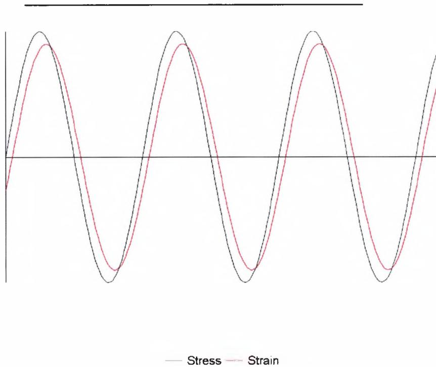
Figure 8.3.1. An applied sinusoidal stress results in a corresponding strain.
