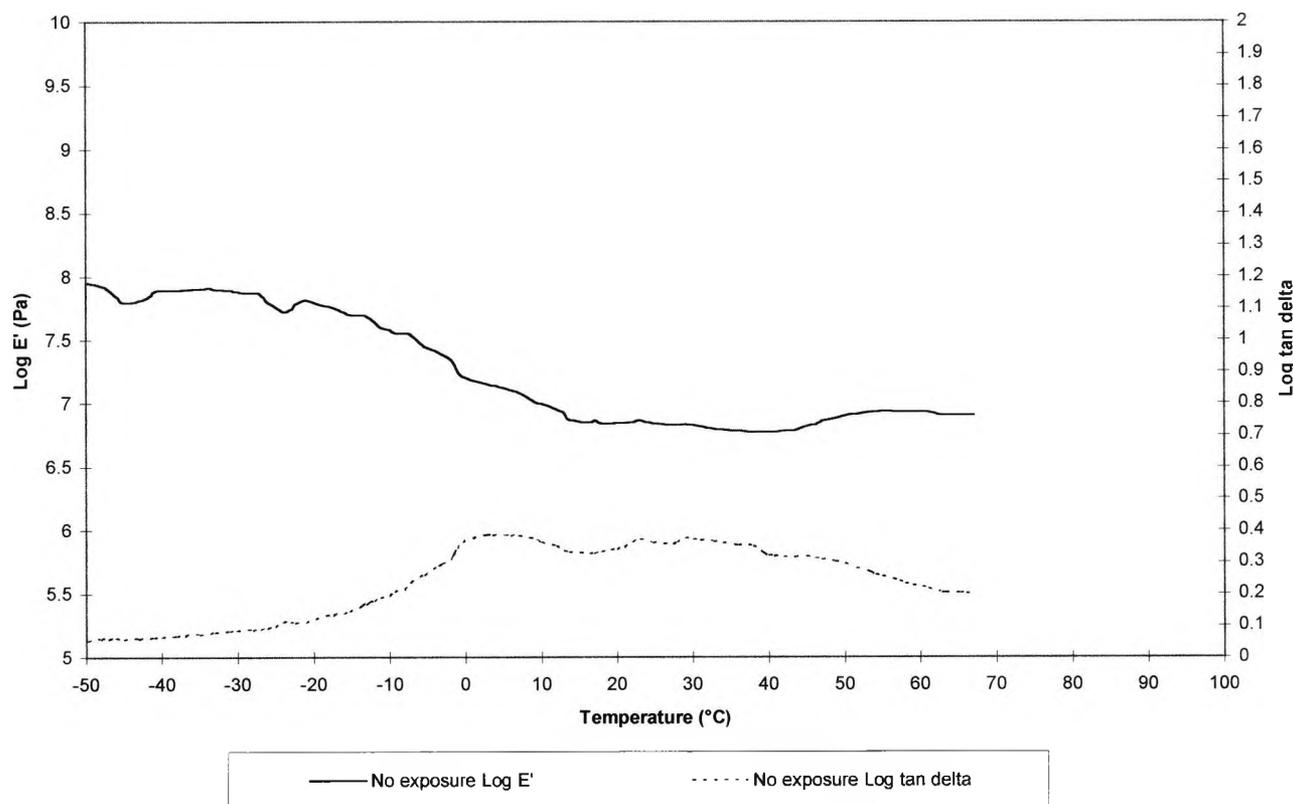
Figure 9.2.3. DMTA plot of the unexposed coating based on the alkyd-acrylic hybrid resin.
