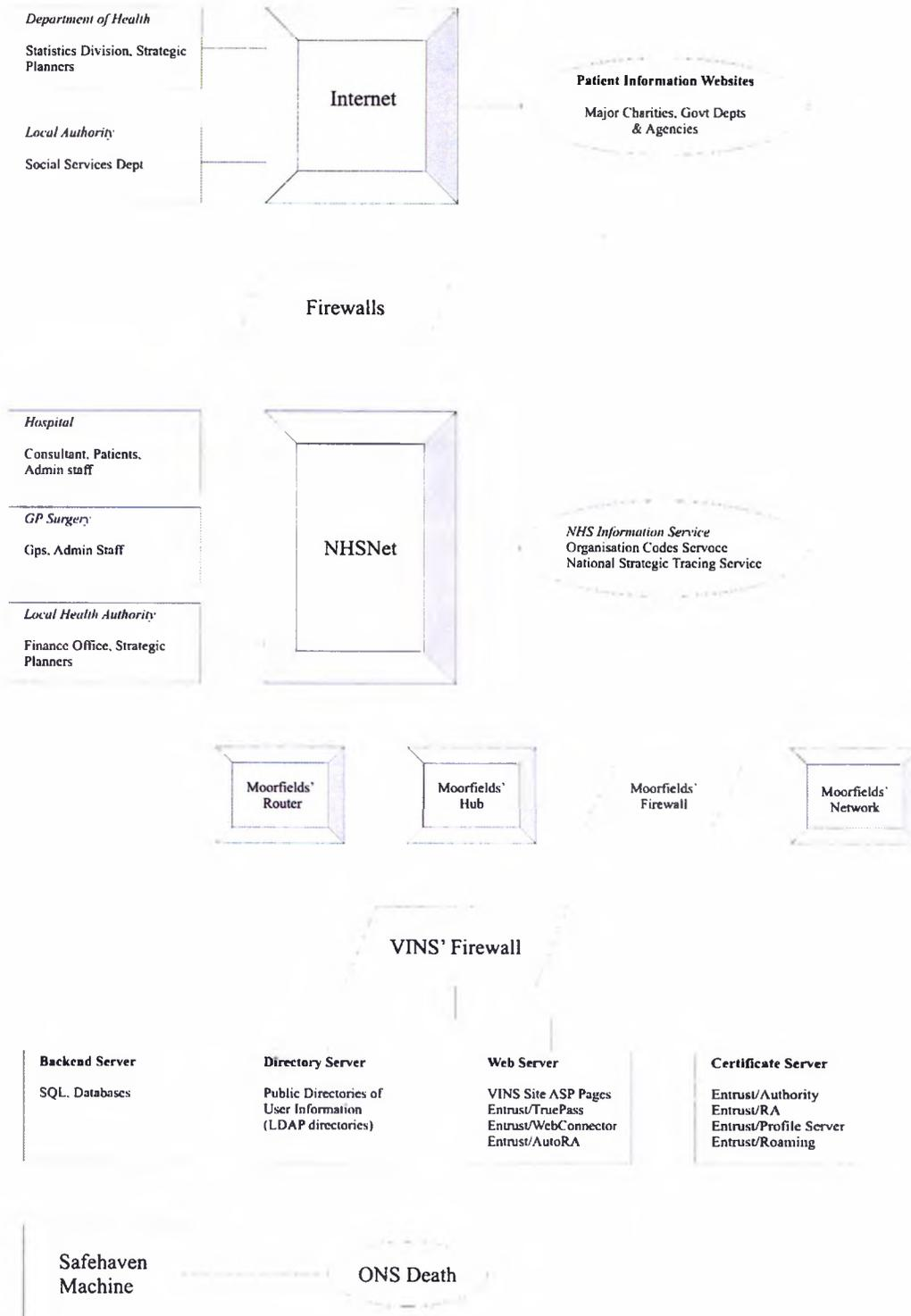
**Figure 6.4..Top level network diagram of the electronic Visual Impairment Notification System (eVINS) for pilots.**
