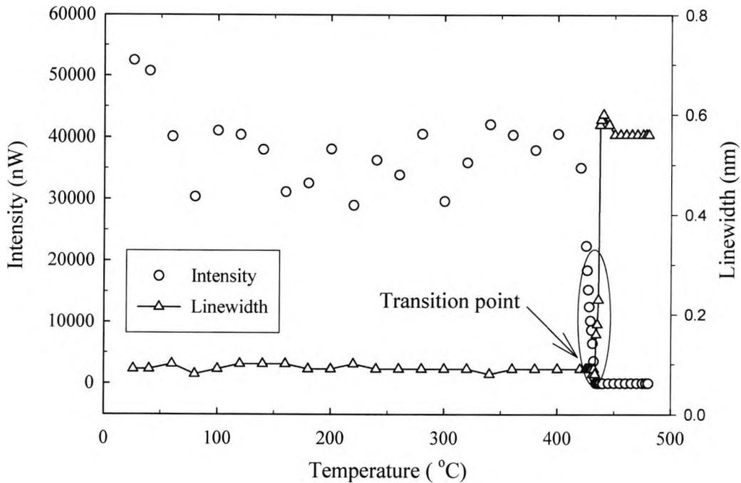
Fig. 5.10: Intensity and linewidth variation of the sensor (zero-strain on chirped grating) with different temperatures from room temperature to 480 °C, with a fixed pump power of 52 mW.
