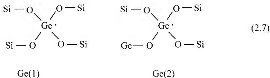
The Ge(1) or Ge(2) centre can trap an electron to convert it into a Ge(1)<sup>-</sup> or Ge(2)<sup>-</sup> centre [Secats *et al.* 1993].
