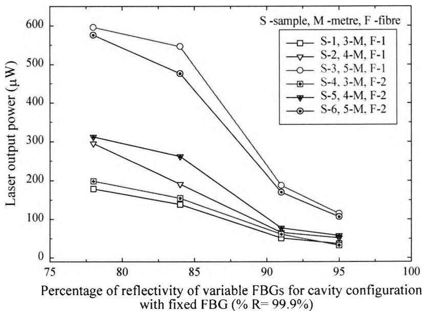
Fig. 3.24: Laser output power as a function of different cavity configurations.
