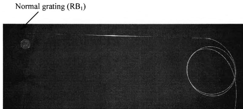
Fig. 4.9: Photograph of the probe containing the normal grating (RB<sub>1</sub>) at the left-end.
