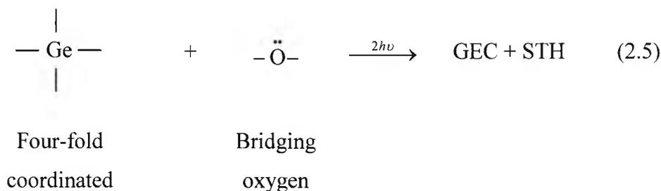
The lone pair electrons on bridging oxygens are excited to the conduction band from the valance band via a two-photon absorption process with excimer laser irradiation; and produced GEC and STH simultaneously. The conversion of the GEC to GeE' centre may be described using the following reaction:
