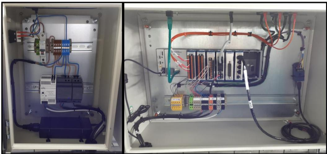
**Figure 6.2 DAQ system with Power supply unit**
