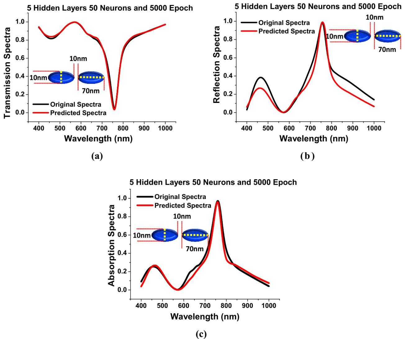
**Figure 5.** *Hidden layer = 5, Neurons = 50 and Epoch = 5000* (a) Shows the comparison between the predicted transmission spectra with respect to the original transmission spectra. (b) Shows the anticipated reflection spectra are compared to the original reflection spectra. (c) Shows the predicted absorption spectra against the original absorption spectra.
