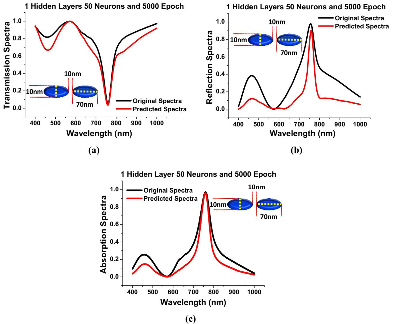
**Figure 4.** *Hidden layer = 1, Neurons = 50 and Epoch = 5000* (a) Shows the comparison between the predicted transmission spectra with respect to the original transmission spectra. (b) Shows the anticipated reflection spectra are compared to the original reflection spectra. (c) Shows the predicted absorption spectra against the original absorption spectra.
