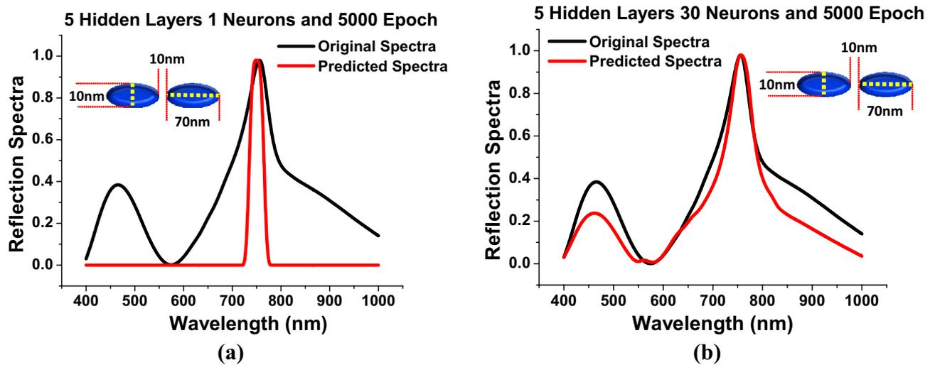
**Figure 7.** Hidden layers= 5 and Epoch = 5000 (a) Shows the comparison of predicted reflection spectra with respect to the original reflection spectra at neuron = 1 (b) Represents the resemblance of predicted reflection spectra with respect to the original reflection spectra at neuron = 30
