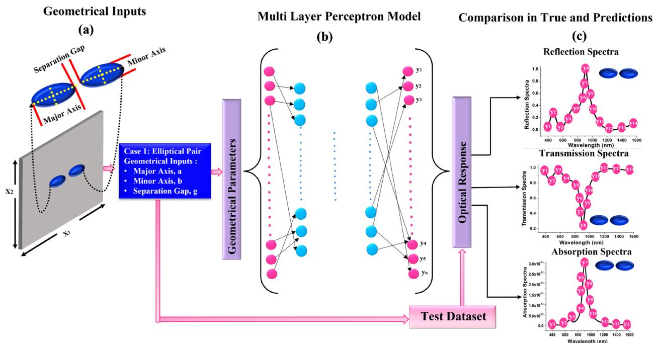
**Figure 2.** (a) Schematic of the structure of two elliptical nanostructures on SiO<sub>2</sub> substrate (The top and front views of a single unit cell with the geometrical parameters are represented in the insets). (b) A DNN model that predicts the optical response over a wavelength range for the given geometrical parameters and (c) Shows the predicted optical Reflection, Transmission and Absorption responses for a given geometrical structure.
