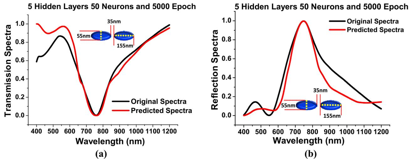
**Figure 10.** *Hidden layer = 5, Neurons = 50 and Epoch = 5000* (a) Shows the comparison between the predicted transmission spectra against the original transmission spectra. (b) Shows the anticipated reflection spectra are compared to the original reflection spectra when  $a = 155$  nm,  $b = 55$  nm,  $g = 35$  nm and  $h = 40$  nm.
