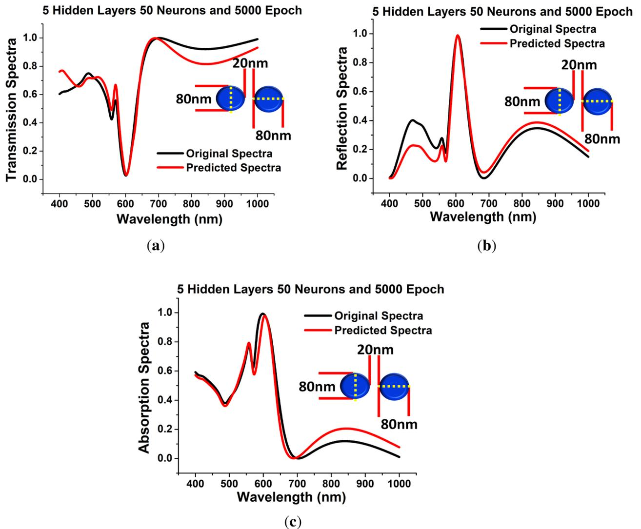
**Figure 9.** *Hidden layer = 5, Neurons = 50 and Epoch = 5000* (a) Shows the comparison between the predicted transmission spectra with respect to the original transmission spectra of circular dimer with  $d = 80\text{ nm}$ ,  $g = 20\text{ nm}$  and  $h = 40\text{ nm}$ . (b) Shows the anticipated reflection spectra are compared to the original reflection spectra. (c) Shows the predicted absorption spectra against the original absorption spectra of the same.
