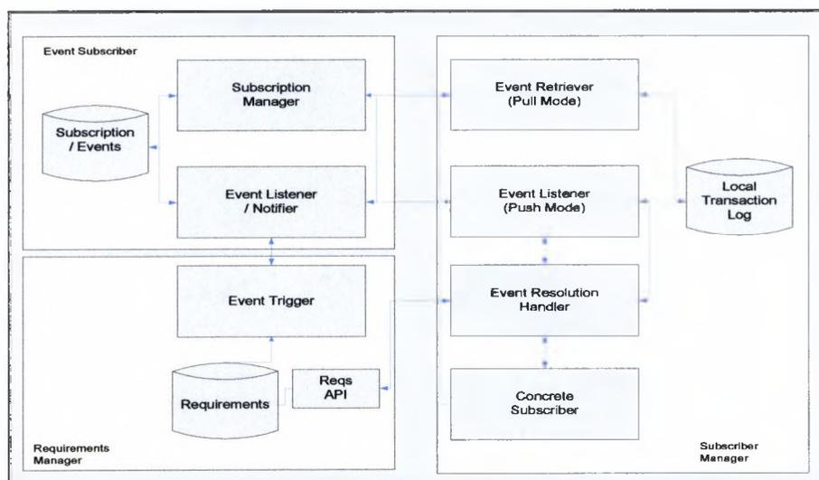
**Figure 2.7 System level model of Event-Based Traceability**
