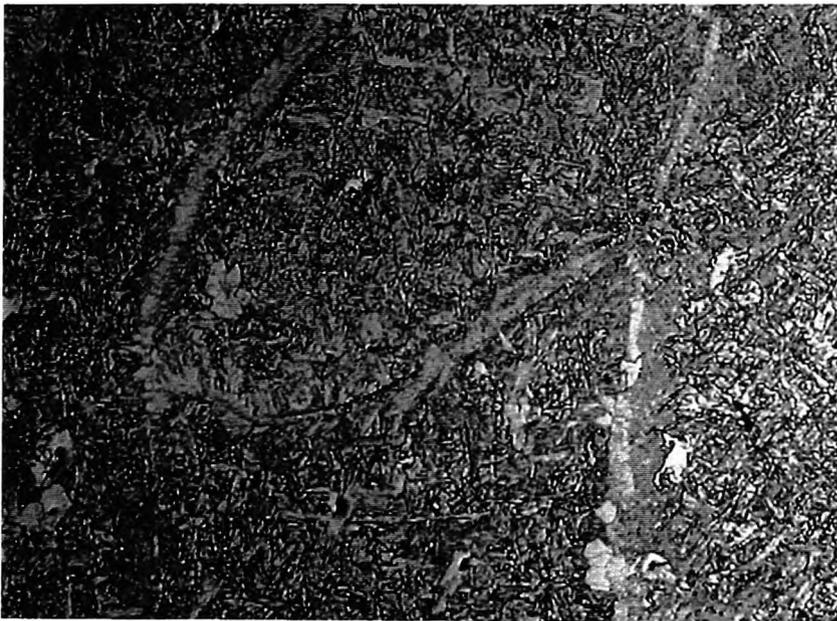
*Figure 5-4* Crack in a thin film of ferrite surrounding coarse austenite grain(90X)
