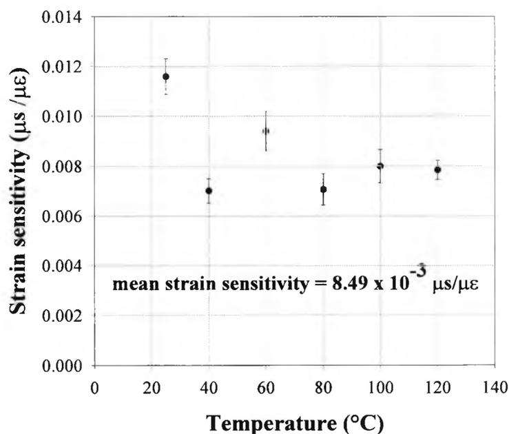
Fig.4.6 Strain sensitivity of the  $\text{Er}^{3+}$ -doped fibre lifetime versus temperature.
