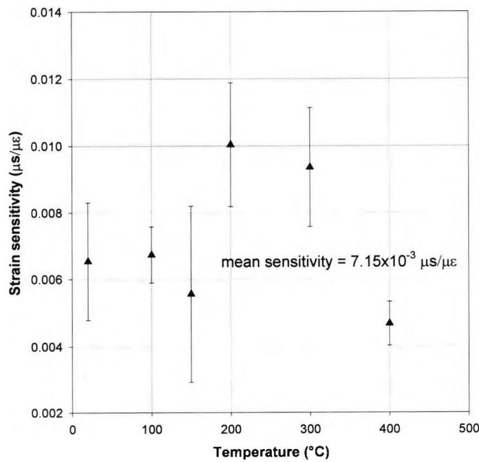
Fig.3.10  $\text{Er}^{3+}$  1050 ppm strain sensitivity of the fluorescent lifetime as a function of temperature.
