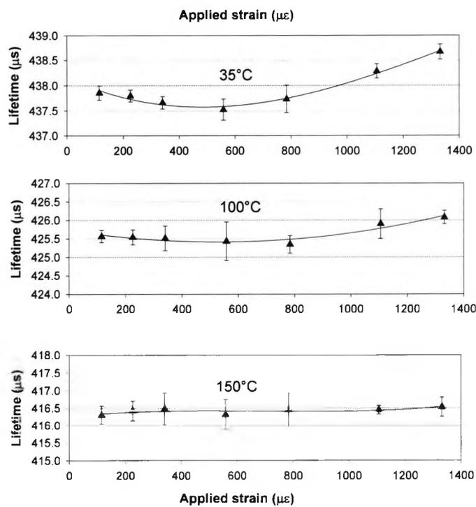
Fig.3.28  $\text{Nd}^{3+}$  sensor 2: lifetime versus strain for the minimum, middle and maximum temperatures.
