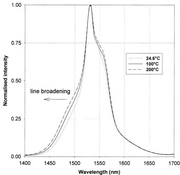
Fig.3.12 Er<sup>3+</sup> 4370 ppm fluorescence spectra recorded from OSA.
