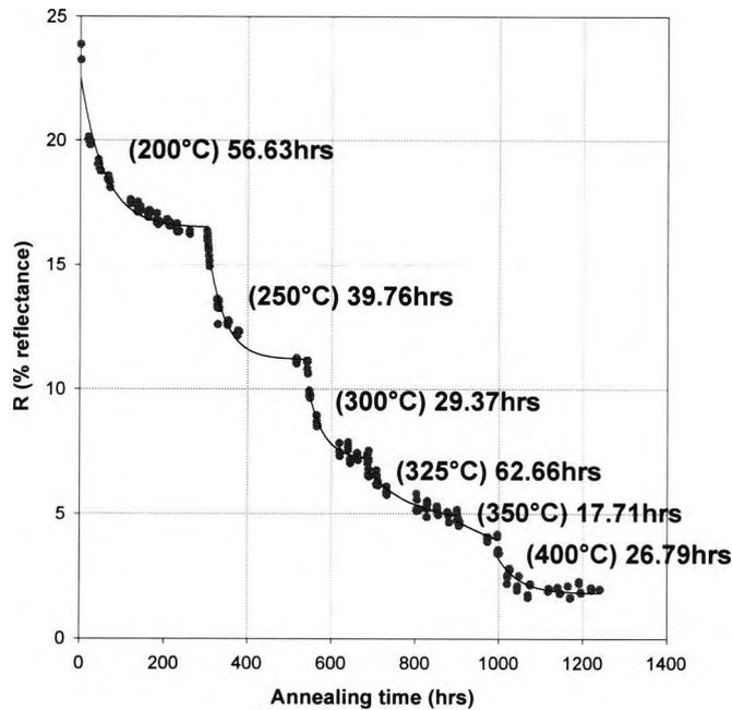
Fig.4.25 Long term thermally induced decay effects on FBG performance.
