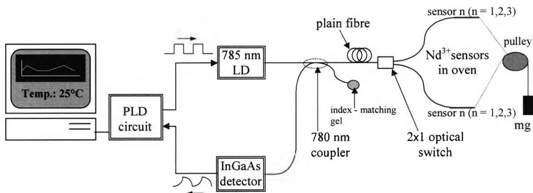
Fig.3.23 Experimental set-up for Nd<sup>3+</sup> fibre temperature/strain calibration.
