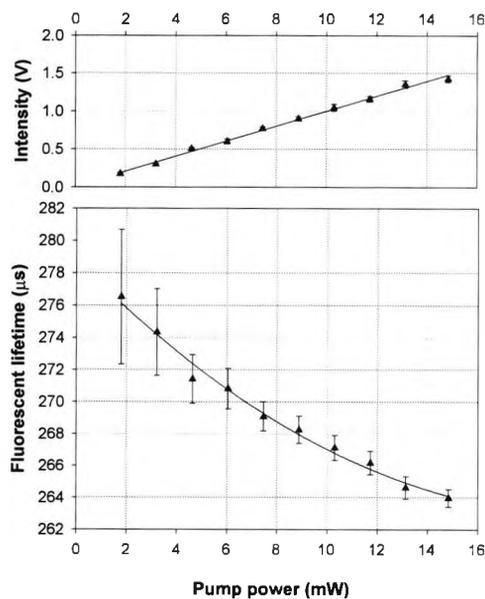
Fig.3.68 Tm<sup>3+</sup>/Ho<sup>3+</sup> co-doped fibre sensor (~10 cm) experimental results on pump power at 26.2°C.
