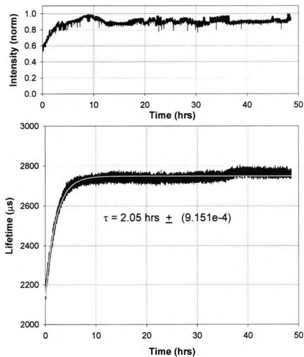
Fig.4.28  $\text{Er}^{3+}:\text{Yb}^{3+}$  co-doped photosensitive fibre annealing at 800°C for 48 hrs.
