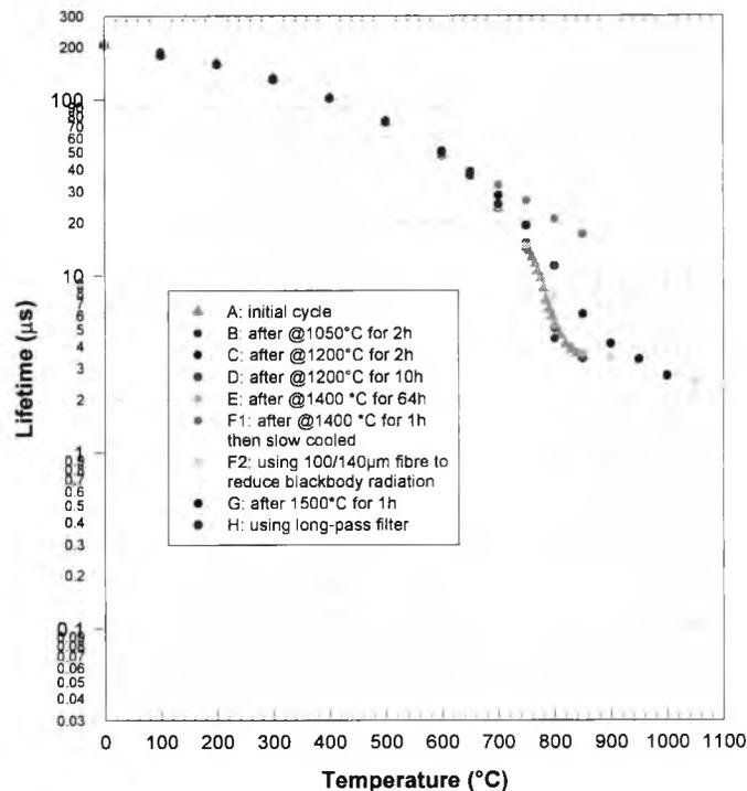
Fig.3.53 Fluorescence @800 nm band - all results.
