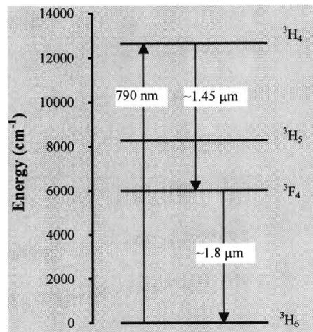
Fig.3.32 Energy level diagram of the  $Tm^{3+}$  ion, showing transitions of interest [11].
