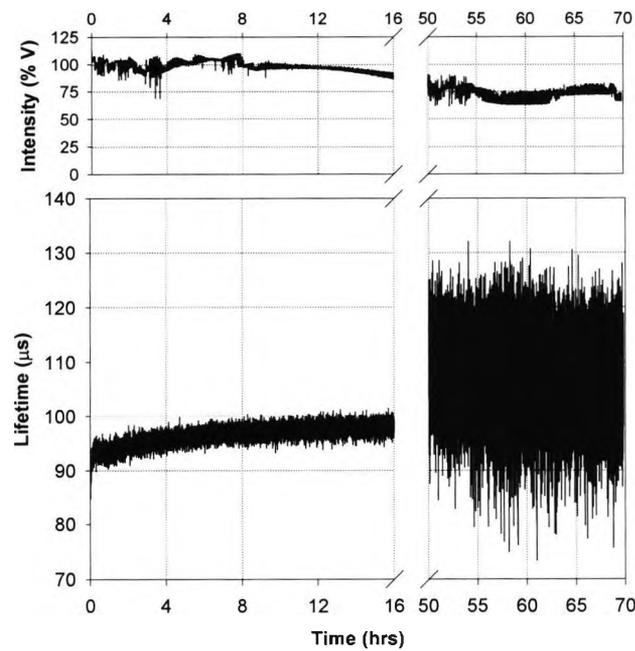
Fig.3.49 Sample (b) annealing at 900°C for 70 hours.
