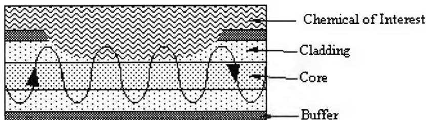
Fig.1.2 Fibre optic evanescent wave absorption technique [7].
