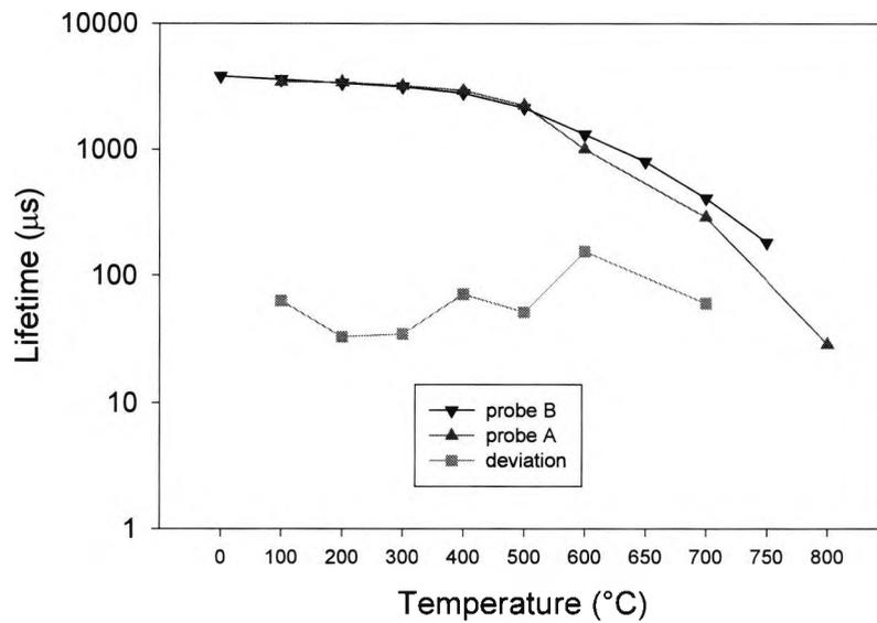
Fig.3.60 Probe A and probe B comparisons and exchangeability for fluorescence at the 1  $\mu\text{m}+$  band.
