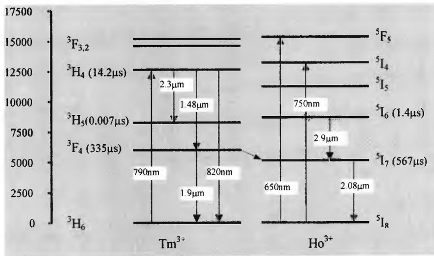
Fig.3.31 Energy level diagram of the  $Tm^{3+}$  and  $Ho^{3+}$  rare earth ions, showing the transitions previously used and lifetimes obtained in brackets from the relevant energy levels [10].
