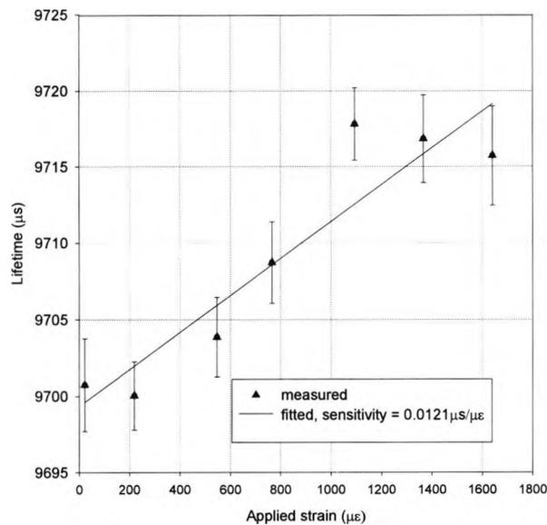
Fig.3.16  $\text{Er}^{3+}$  4370 ppm fluorescent lifetime strain effect at 100°C.
