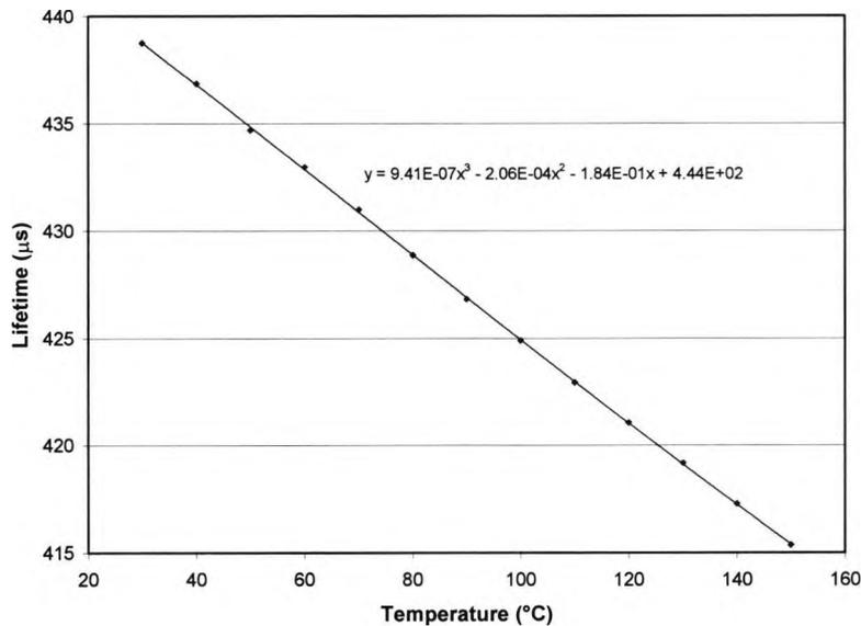
Fig.3.24 Nd<sup>3+</sup> temperature calibration data for sensor 1.
