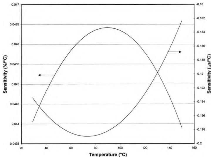
Fig.3.25 Nd<sup>3+</sup> temperature sensitivities of sensor 1.
