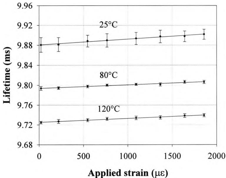
Fig.4.5 Strain effect on the lifetime of  $\text{Er}^{3+}$ -doped fibre element of the combined  $\text{Er}^{3+}$ -doped fibre/FBG sensor at 25°C, 60°C and 120°C.
