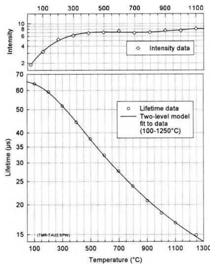
Fig.3.40 Thermal characteristics of the fluorescence of 280 ppm  $Tm^{3+}$ -doped fibre [21].
