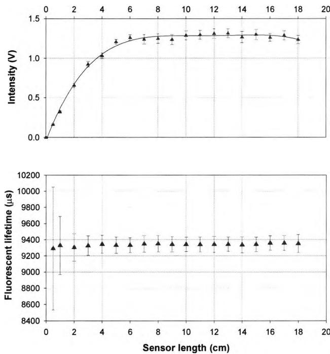
Fig.3.65 Er<sup>3+</sup> Yb<sup>3+</sup> co-doped fibre sensor length effects at 26.2°C.
