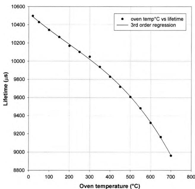
Fig.3.8  $\text{Er}^{3+}$  1050 ppm temperature calibration (without strain).
