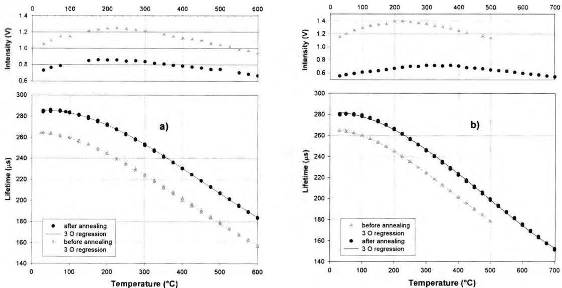
Fig.3.47  $Tm^{3+}/Ho^{3+}$  co-doped fibre samples before and after annealing process (a) sample A and (b) sample B.
