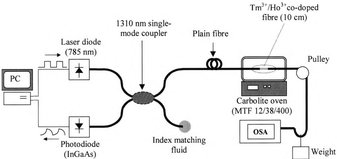
Fig.3.35 Experimental arrangement (B) used to measure the temperature and strain dependence of  $Tm^{3+}/Ho^{3+}$  co-doped fibre.
