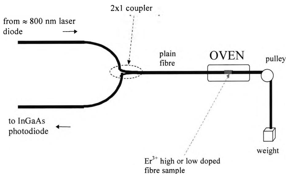
Fig.3.1 Simplified schematic of experimental arrangement used in Er<sup>3+</sup> doped fibre strain and temperature tests.
