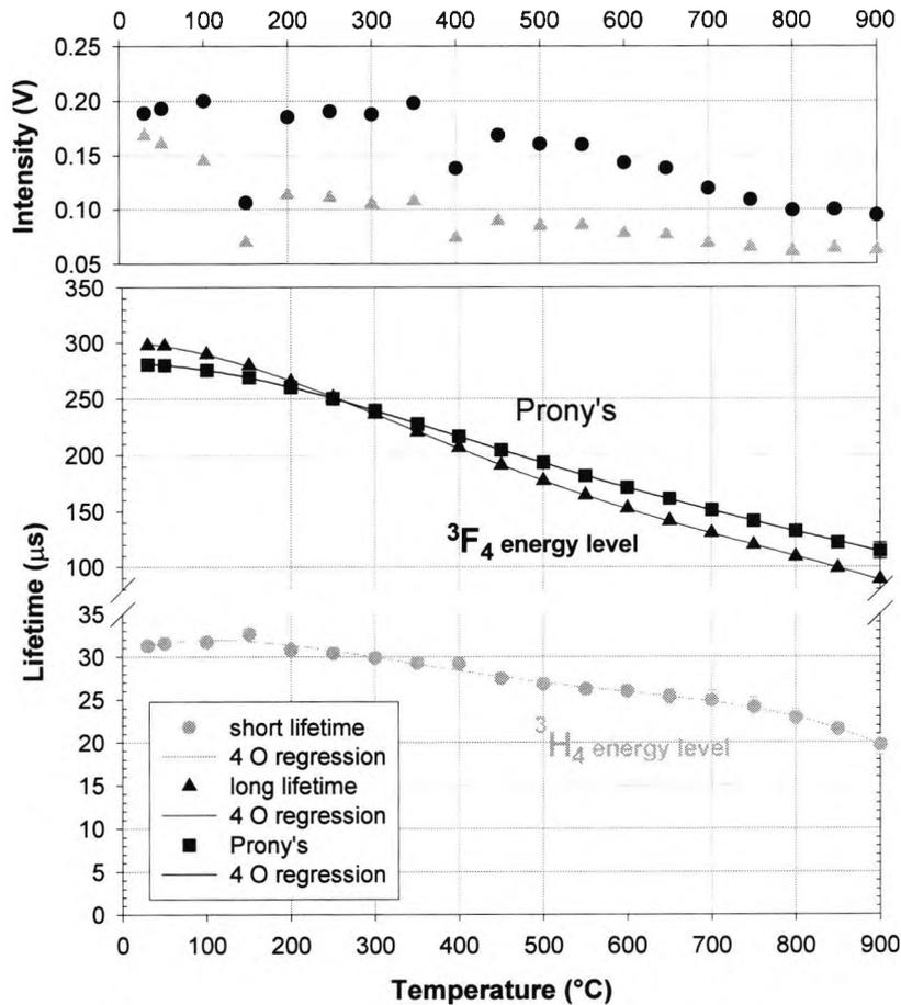
Fig.3.46  $Tm^{3+}/Ho^{3+}$  co-doped fibre high temperature characteristics (up to  $900^{\circ}C$ ) of the energy levels involved (without any thermal annealing).
