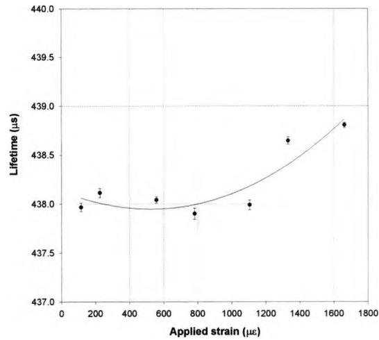
Fig.3.27  $\text{Nd}^{3+}$  sensor 1: strain effect on lifetime at 35°C.
