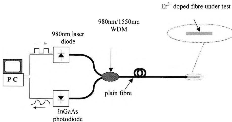
Fig.3.61  $\text{Er}^{3+}$  doped fibre experimental set-up for sensor length testing.
