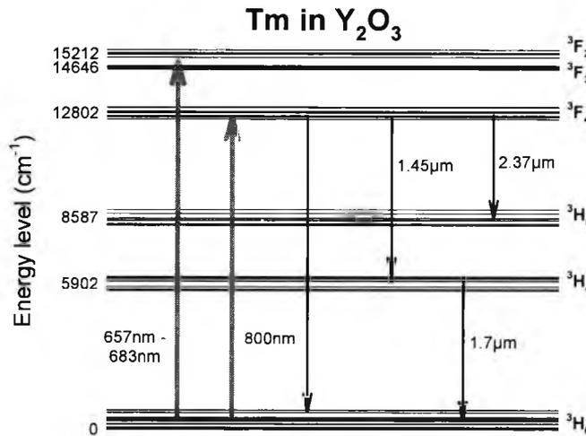
Fig.3.51  $\text{Tm}^{3+}$  in  $\text{Y}_2\text{O}_3$  energy level diagram showing the relevant electronic energy levels of  $\text{Tm}^{3+}$  in  $\text{Y}_2\text{O}_3$  (data from RSTB's database of laser materials, MS474, NASA-LaRC, Hampton, VA23681-2199, USA).
