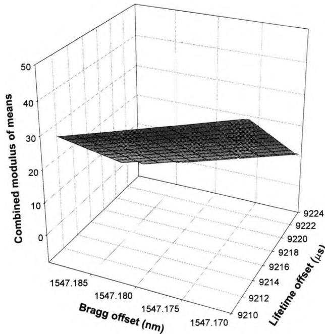
Fig.4.22 Sensor 3 – means modelling of baseline values to achieve a combined minima for optimisation of use (over the range 30 –150°C).
