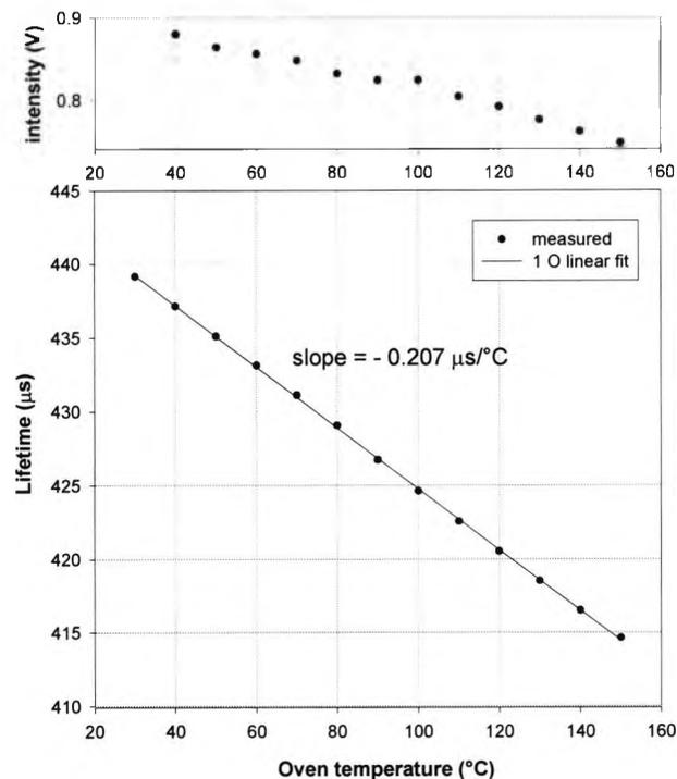
Fig.3.29 Nd<sup>3+</sup> sensor 3: lifetime versus temperature calibration.
