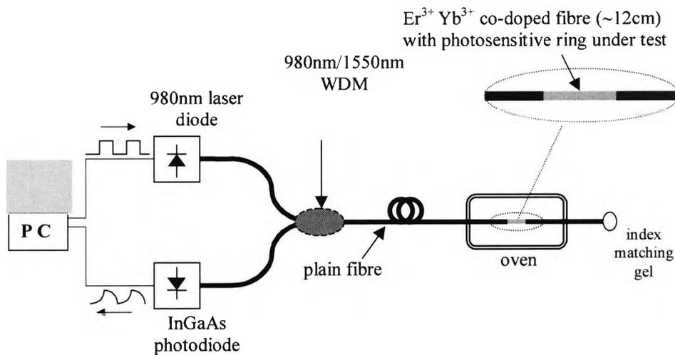
Fig.3.18  $\text{Er}^{3+}$   $\text{Yb}^{3+}$  co-doped fibre experimental set-up for temperature measurement.
