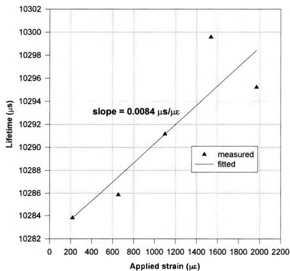
Fig.3.4 Lifetime as a function of strain at 50°C for 200 ppm Er<sup>3+</sup> doped fibre.
