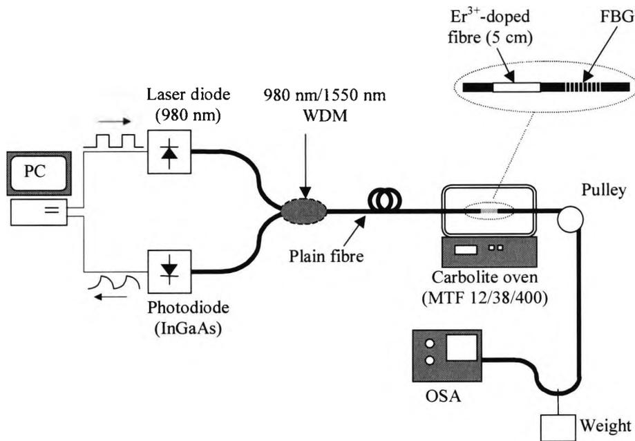
Fig.4.2 Simplified schematic of the experimental arrangement used for the temperature and strain test of the combined Er<sup>3+</sup>-doped fibre/FBG sensor.
