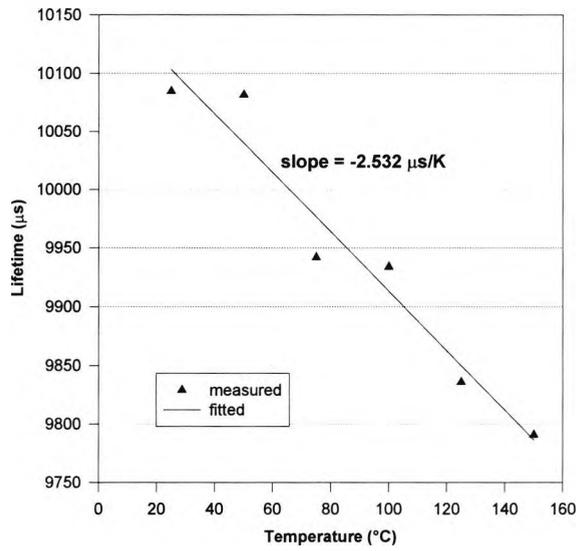
Fig.3.3 Lifetime vs. temperature (without strain) for 960 ppm Er<sup>3+</sup> doped fibre.
