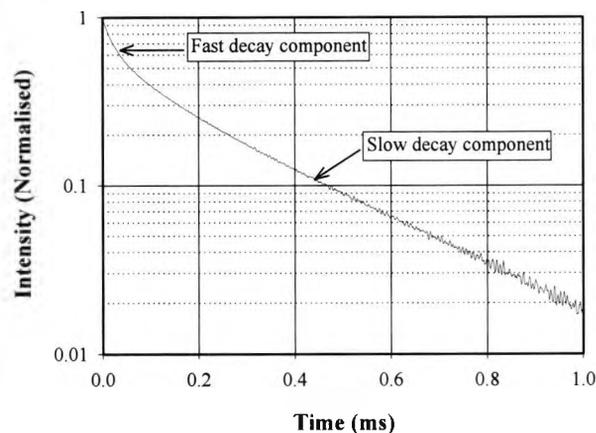
Fig.3.37 Multi-exponential form of  $Tm^{3+}/Ho^{3+}$  co-doped fibre fluorescence, measured at  $22^\circ C$ .
