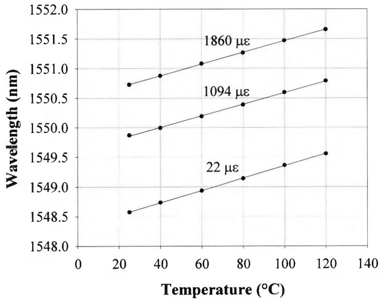
Fig.4.7 Wavelength change as a function of temperature for the FBG at three different applied strains.
