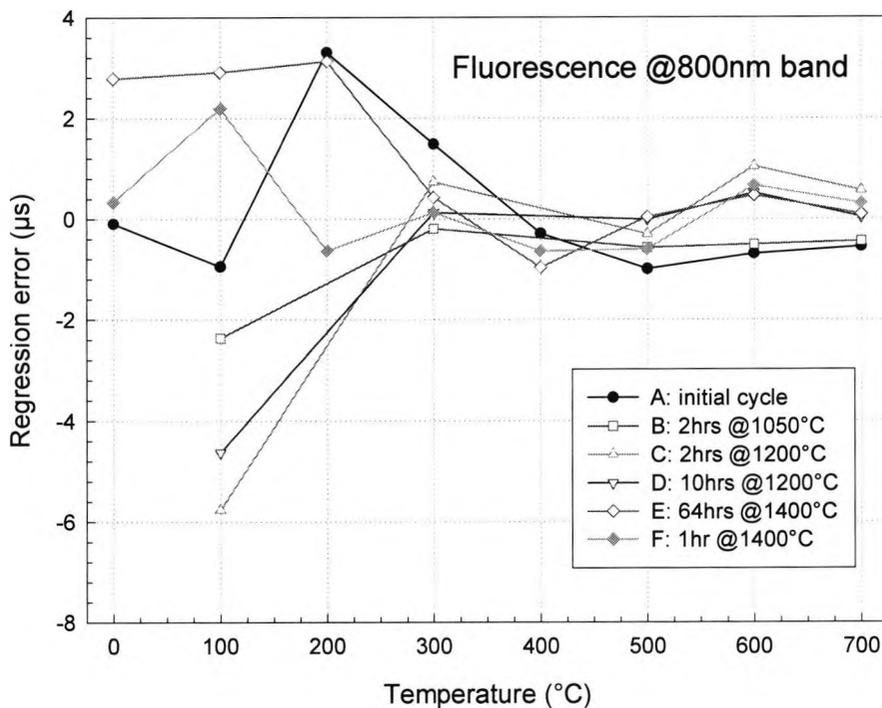
Fig.3.55 Regression errors of lifetime data of  $Tm^{3+}:Y_2O_3$  fluorescence at 800 nm.
