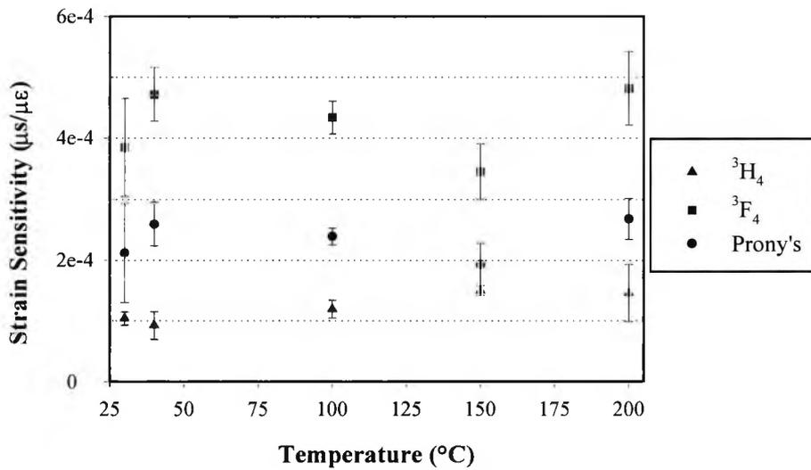
Fig.3.45 Strain sensitivity of the  $^3F_4$  and  $^3H_4$  energy level lifetimes of  $Tm^{3+}/Ho^{3+}$  co-doped fibre together with the single exponential Prony fit to the fluorescence decay at various temperatures.
