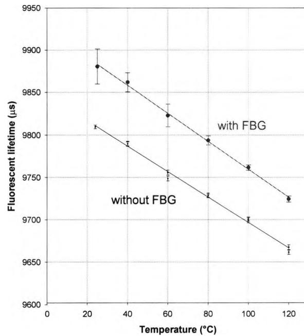
Fig.4.4 Temperature calibration of the  $\text{Er}^{3+}$ -doped fibre element of the combined  $\text{Er}^{3+}$ -doped fibre/FBG sensor (i.e. with zero strain ) compared with previous results from the same fibre without grating, both shown over the same temperature range.
