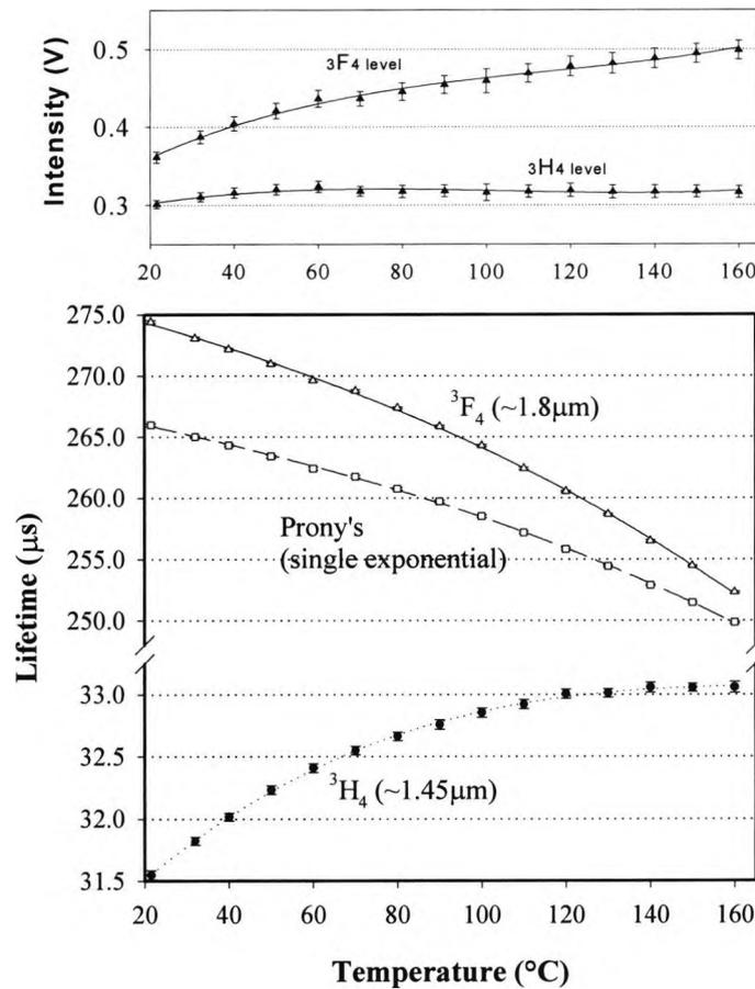
Fig.3.41 Temperature dependence of the intensities and fluorescent lifetimes of the  ${}^3F_4$  and  ${}^3H_4$  energy levels of  $Tm^{3+}/Ho^{3+}$  co-doped fibre together with the single exponential Prony fit to the fluorescence decay. Solid lines are 3<sup>rd</sup> order polynomial fits.
