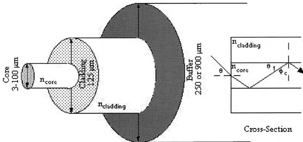
Fig.1.1 Cross-sectional view of a typical optical fibre [7].
