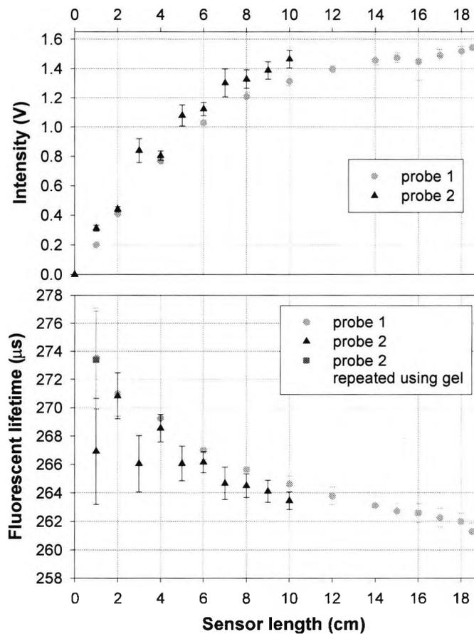
Fig.3.67  $Tm^{3+}/Ho^{3+}$  co-doped fibre experimental results on sensor lengths at 26.8°C.
