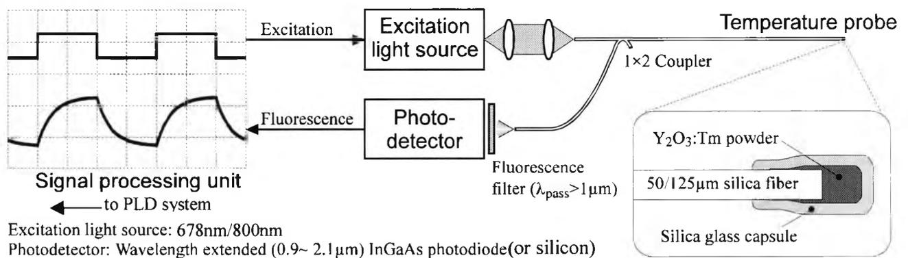
Fig.3.52 Experimental set-up used for  $Tm^{3+}$  in  $Y_2O_3$  [27].
