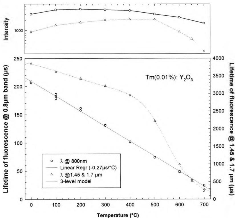
Fig.3.57 Thermal characteristics of  $Tm^{3+}$  fluorescence in  $Y_2O_3$ .
