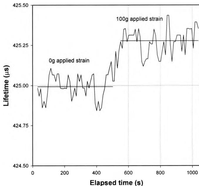
Fig.3.26 Nd<sup>3+</sup> sensor 1 – effect of strain at 100°C.
