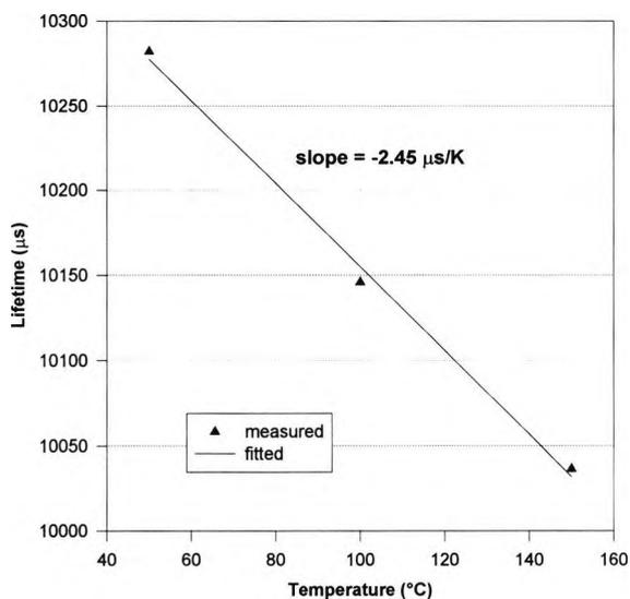
Fig.3.5 Lifetime vs. temperature (without strain) plot for 200 ppm Er<sup>3+</sup> doped fibre.
