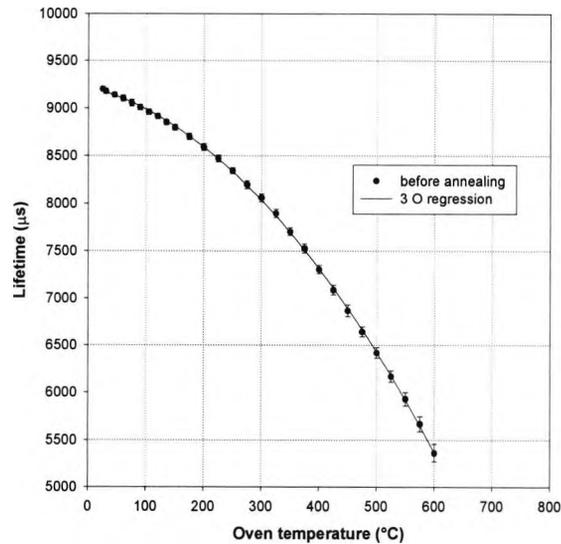
Fig.3.19 Er<sup>3+</sup> Yb<sup>3+</sup> co-doped fibre initial temperature calibration.
