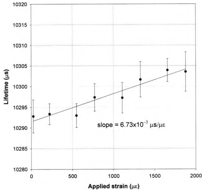
Fig.3.9  $\text{Er}^{3+}$  1050 ppm strain sensitivity of the fluorescent lifetime at 100°C.
