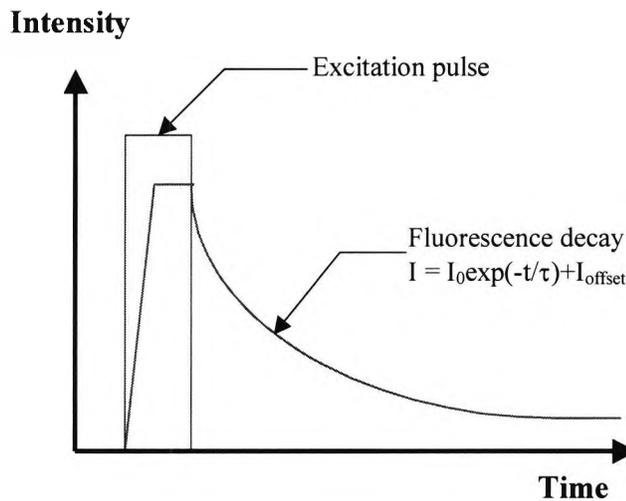
Fig.1.4 Schematic of the decay-time approach.
