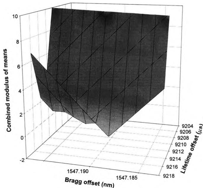
Fig.4.21 Sensor 3 – means modelling of baseline values to achieve a combined minima for optimisation of use (over the range 30 –120°C).
