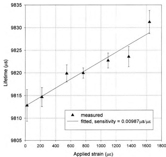
Fig.3.15 Er<sup>3+</sup> 4370 ppm fluorescent lifetime strain effect at 40°C.
