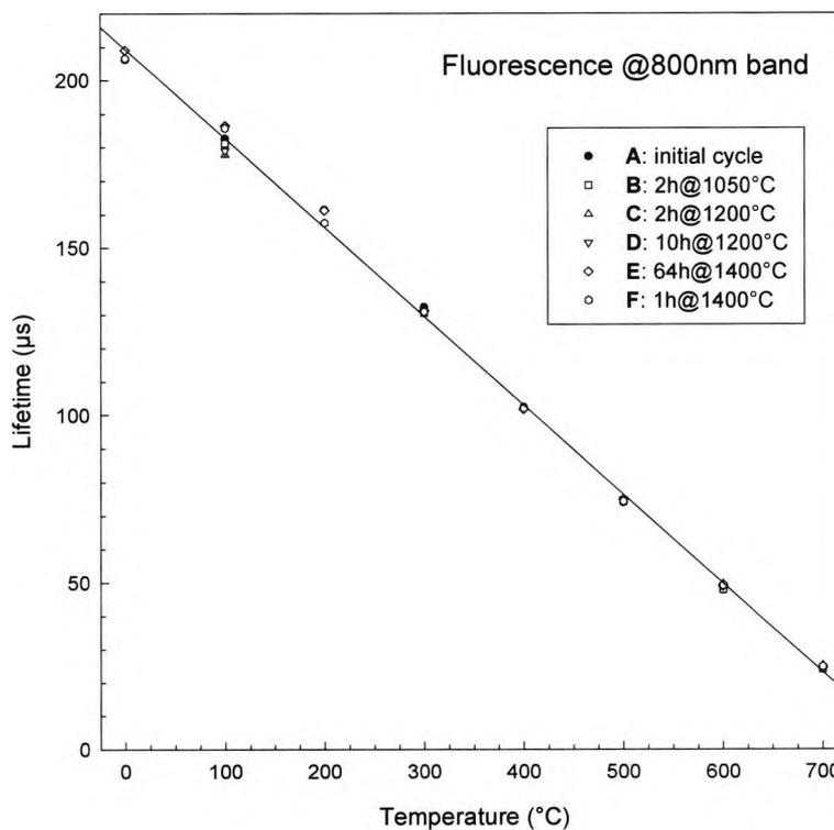
Fig.3.54 Lifetime of  $Tm^{3+}:Y_2O_3$  fluorescence at 800 nm.
