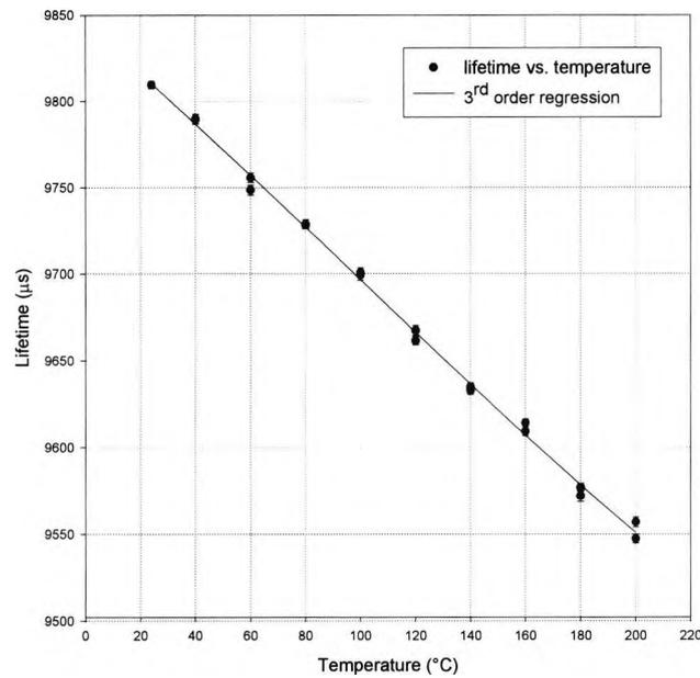
Fig.3.14 Er<sup>3+</sup> 4370 ppm fluorescent lifetime versus temperature.
