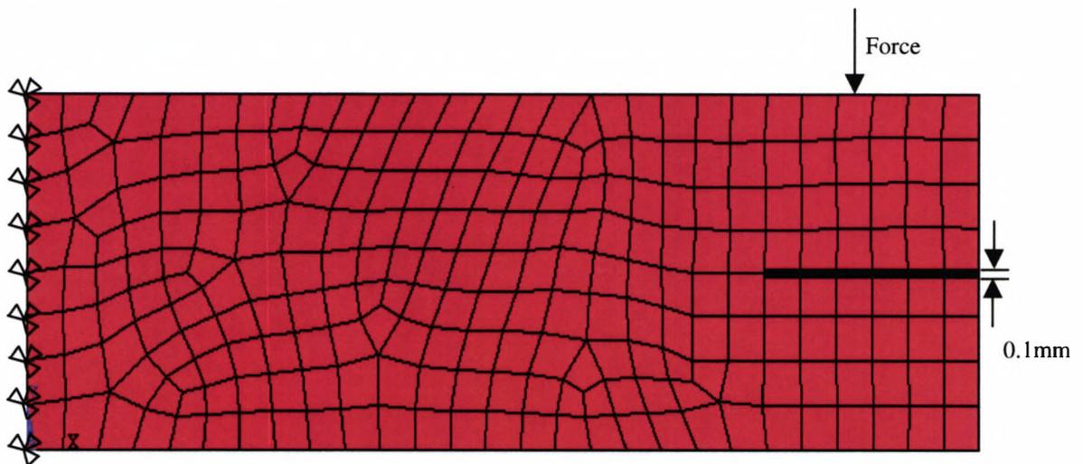
Figure 10.9: Mesh of the model with contact element
