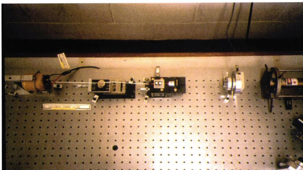
Figure B2: Laboratory Set-up, Polarised Light into the fibre
