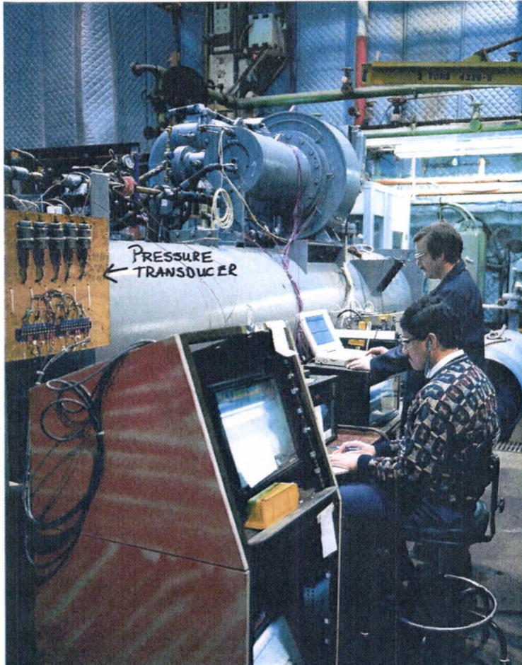
**Figure 7: Data collection system – Pressure Transducers, temperature chart recorders and Vibration acquisition**
