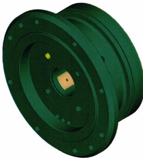
**Figure 4.7a: Solid model of front of hydrostatic bearing**
