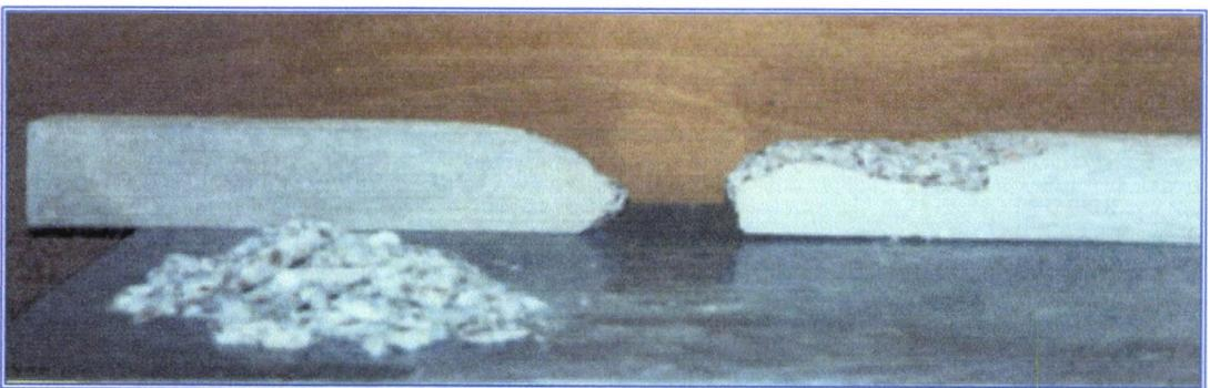
**Figure 8.1.2.b Beam after an explosive spalling.**
