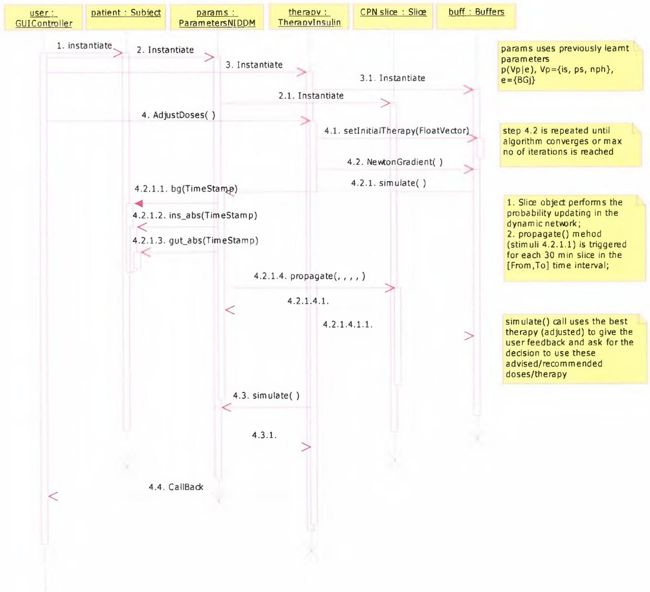
**Figure 8.10** Sequence diagram associated with Figure 8.9. It shows the sequence of messages/stimuli passed between objects to realise 'Advice' use case
