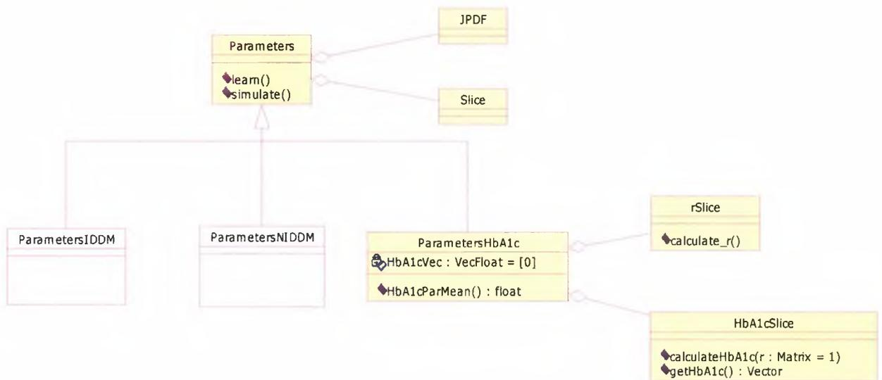
**Figure 8.11** Class diagram showing the additional classes to implement the  $HbA_{1c}$  prediction use case
