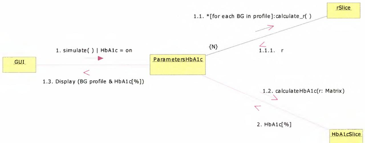
**Figure 8.12** Collaboration diagram to realise the predict steady state  $HbA_{1c}$  use case
