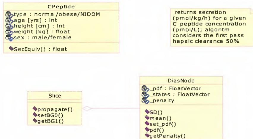
**Figure 8.7** Class diagrams showing attributes and operations of some of the utility classes. Slice has an aggregation relationship with DiasNode instances storing model stochastic variables  $BG_0$ , intermediary glucose balance and active insulin.
