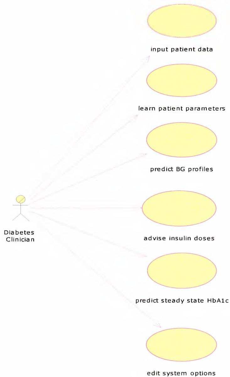
**Figure 8.5** Use case diagram showing possible ways the user can interact with the system
