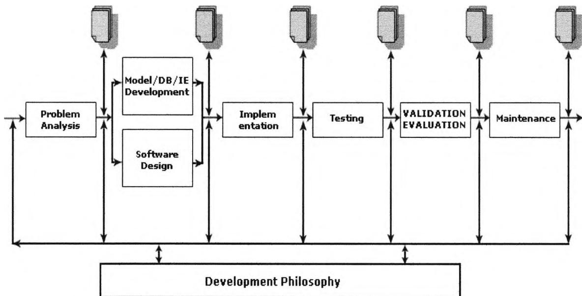
**Figure 7.3** Waterfall development life cycle including model/database(DB)/ inference engine (IE) and validation/evaluation stages. Development philosophy sets the values and beliefs that are driving the waterfall life-cycle, and in particular controls problem analysis, model/DB/IE and validation/evaluation stages
