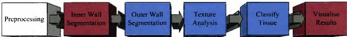
Figure 1.1: An overview of the IBD detection system. White blocks indicate significant existing research, red blocks indicate some existing research, and blue blocks indicate little existing research within our problem domain.
