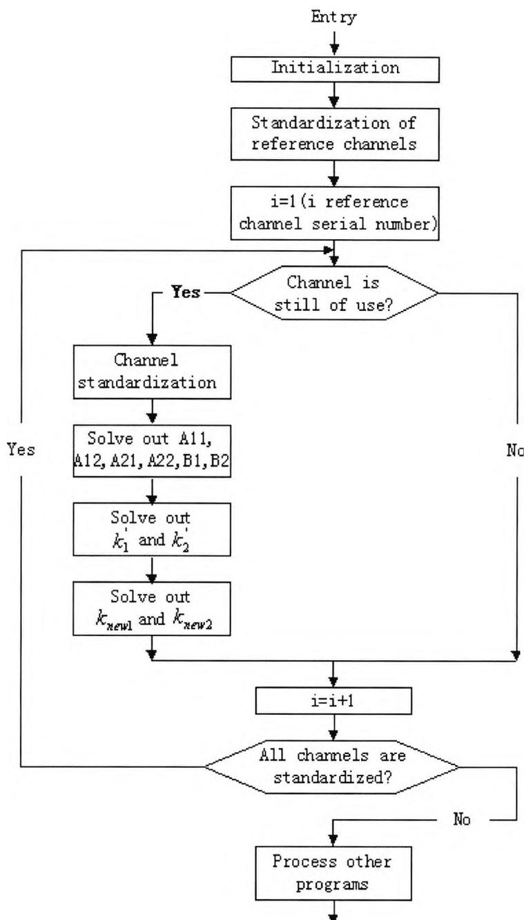
Fig. 10.1 Flow chart of automatic adjustment of channel parameters
