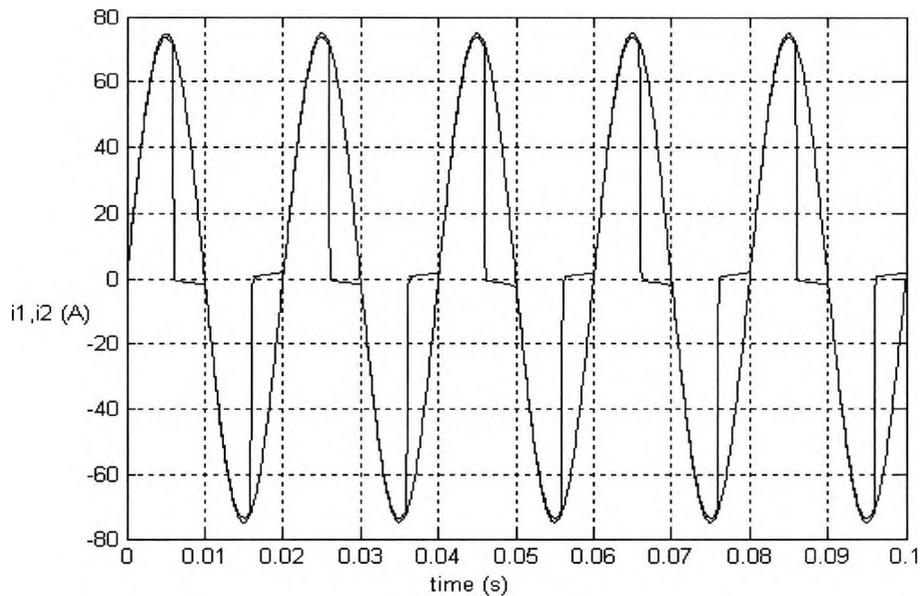
Fig. 6.2(b) CT steady-state saturation under resistance current excitation condition
