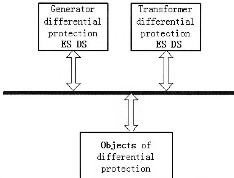
Fig. 9.6 Object oriented application of generator and transformer differential protections
