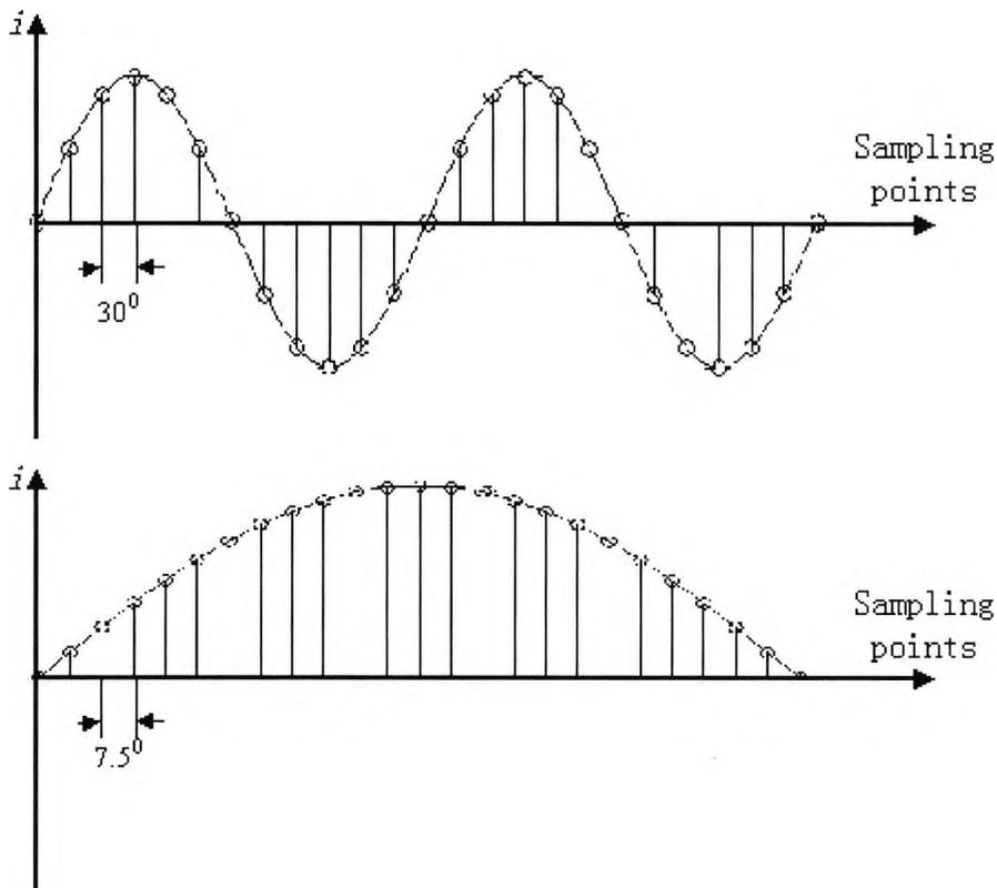
Fig. 11.1 Comparison of waveforms with two sampling frequencies
