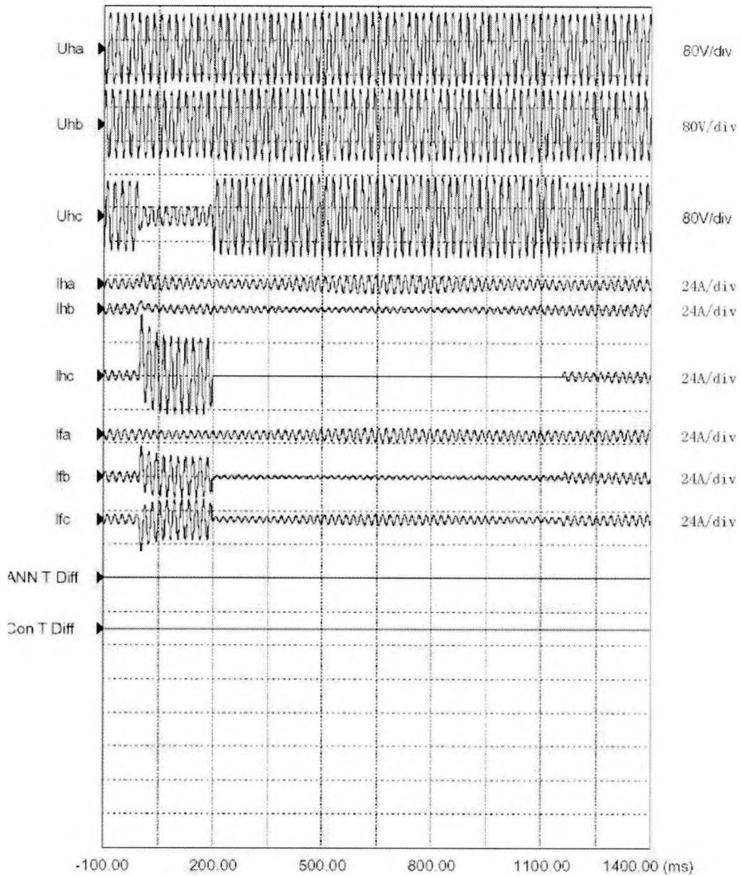
Fig 8.11 Successful reclosed after phase C to ground fault occurred in transmission line.
