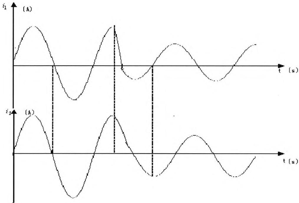
$i_1$  -- The primary current,  $i_2$  -- The secondary current
