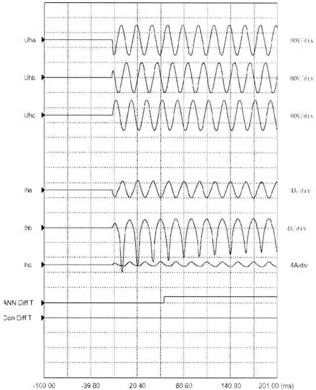
Fig 4.7 Transformer interturn fault (1.7%) in low-voltage side when switching on
