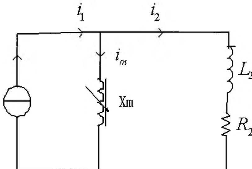
Fig. 6.1(a) CT equivalent circuit
