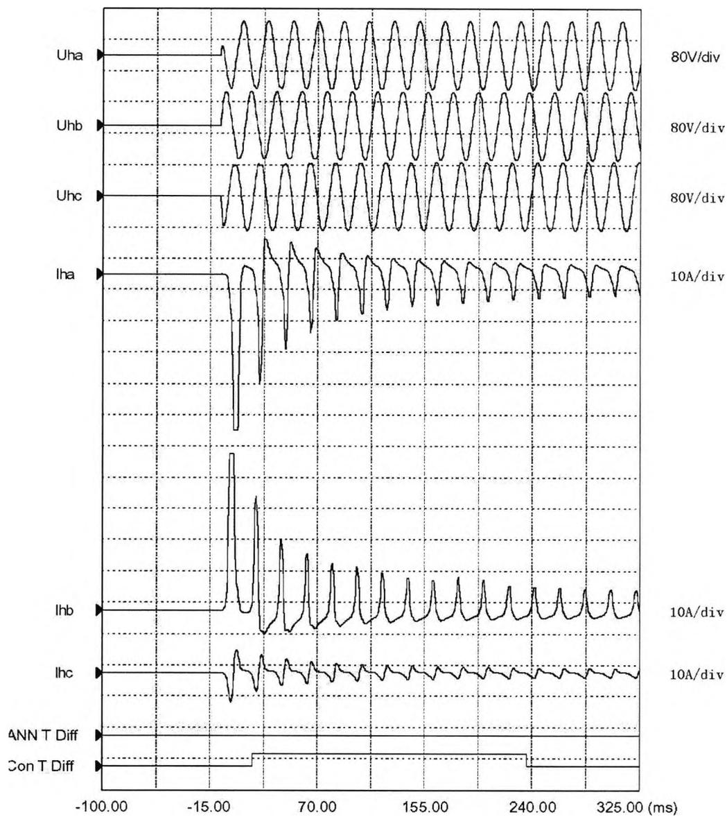
Fig 4.5 Transformer inrush current when switching on
