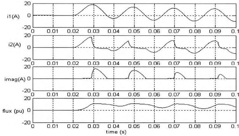
Fig. 6.2(a) CT transient saturation under fault current excitation condition
