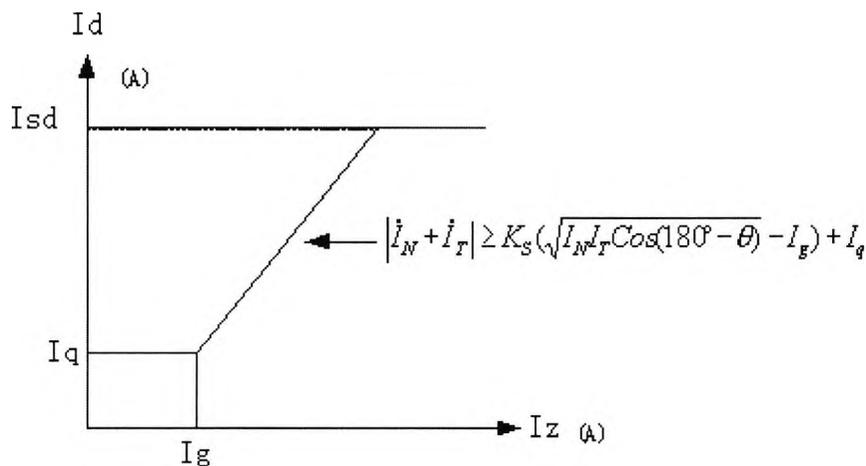
Fig. 2.2 Generator differential protection based on scalar product restraint
