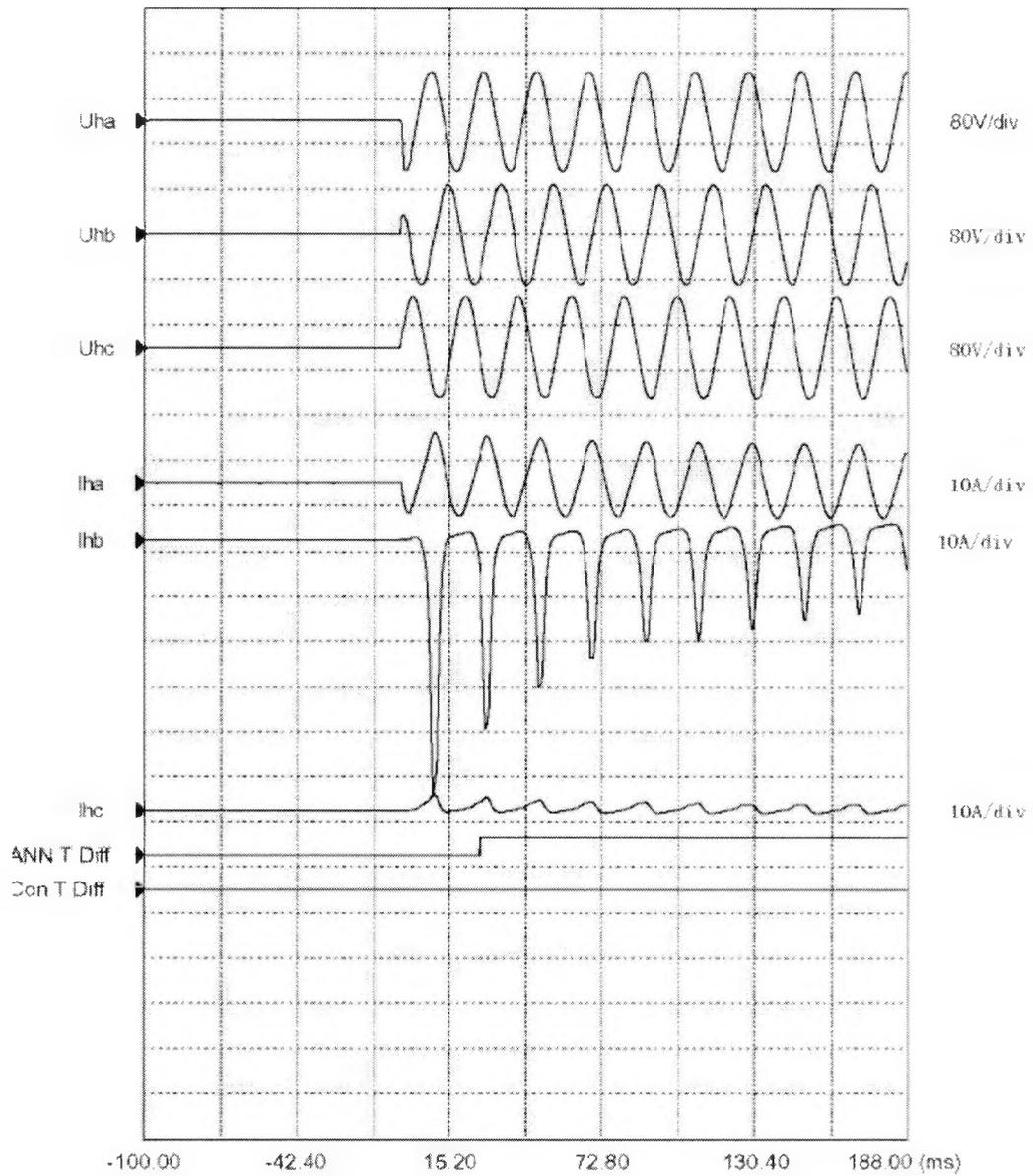
Fig 4.6 Transformer inter-turn fault (2.4%) at high-voltage side when switching on
