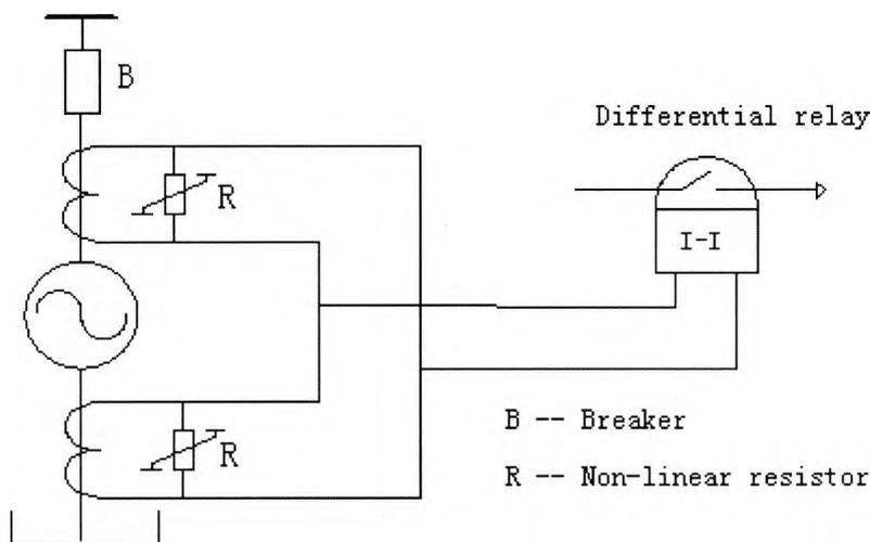
Fig. 5.1 Relays against CT secondary open-circuit
