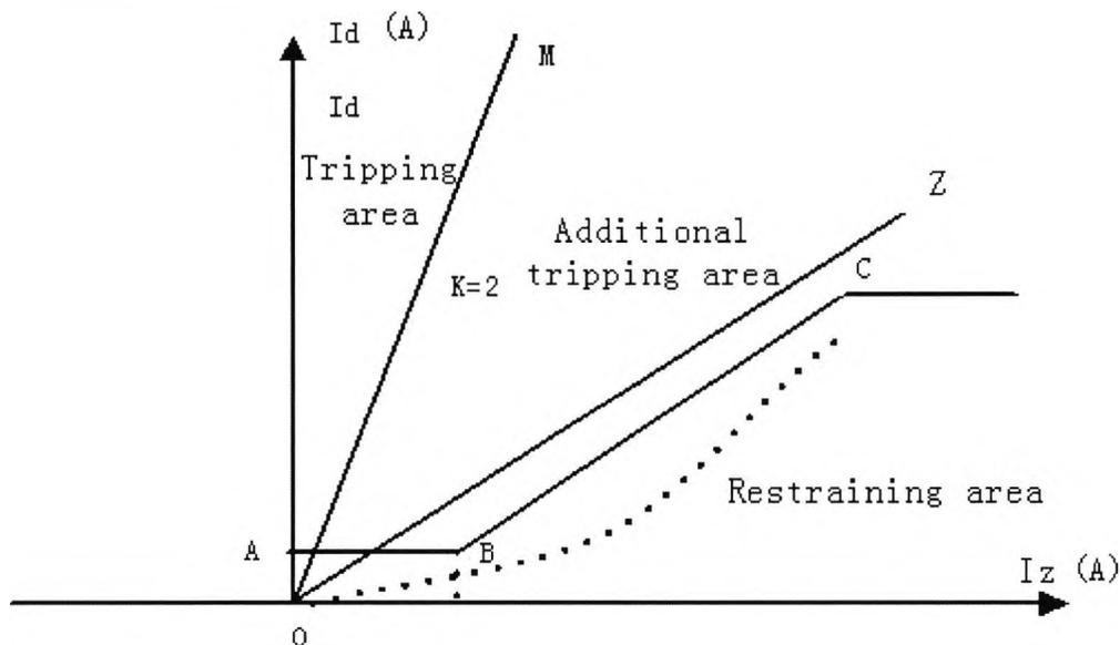
Fig. 8.5 The corresponding relation between the scalar product restraint principle and
