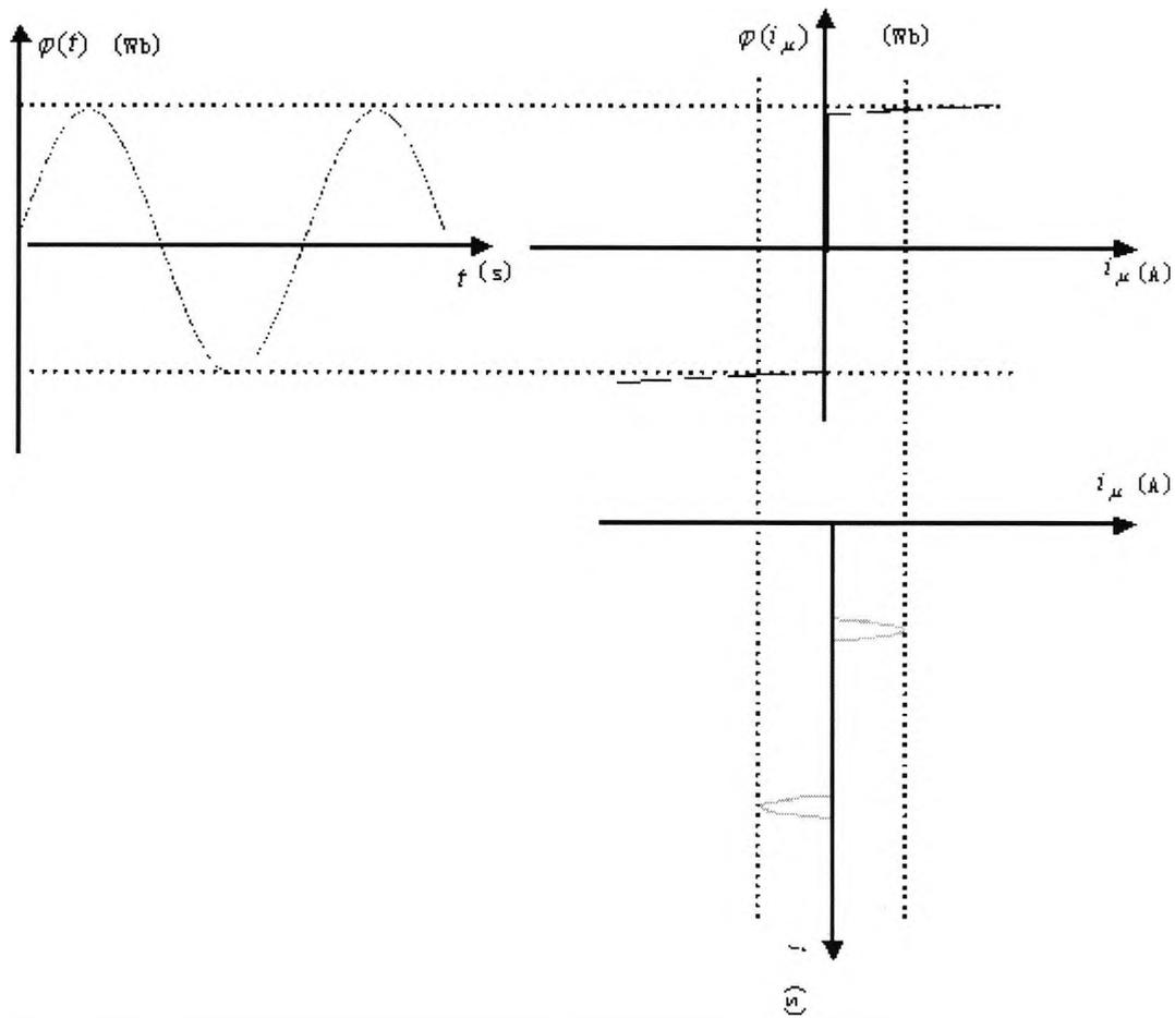
Fig. 4.1 Biased current during slightly over-excitation of transformer
