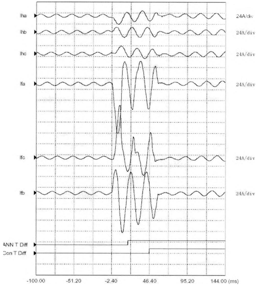
Fig. 6.5 A three-phase internal short-circuit occurred in low side of transformer
