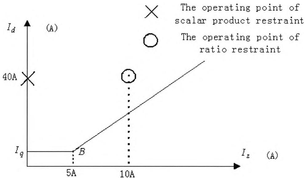
Suppose  $I_N=10$  (A),  $I_T=30$  (A), internal angle  $180^\circ - 0 = 180^\circ$
