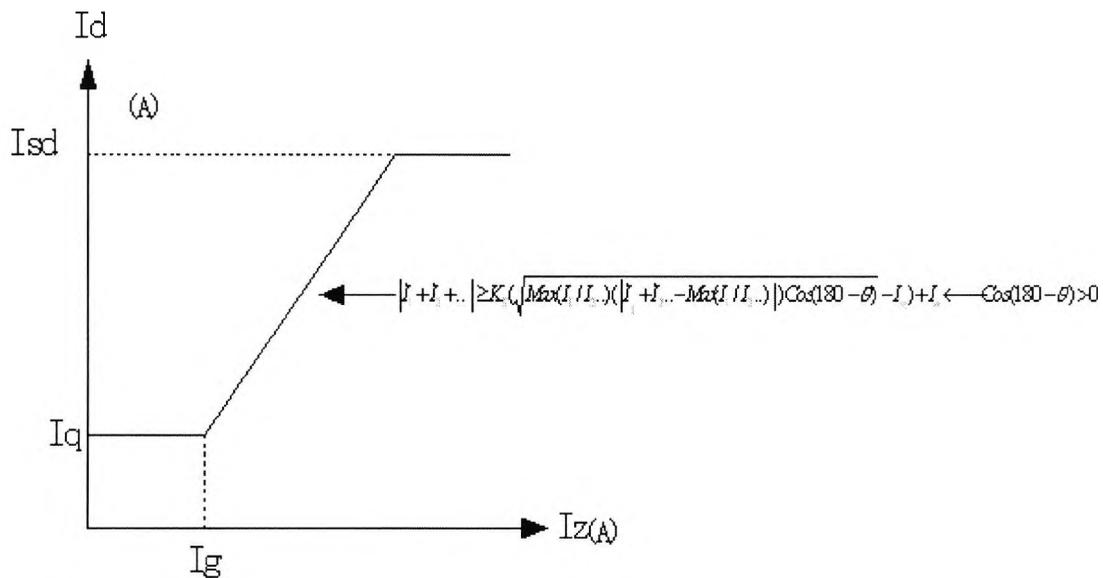
Fig. 2.3 Scalar product restraint characteristic curve
