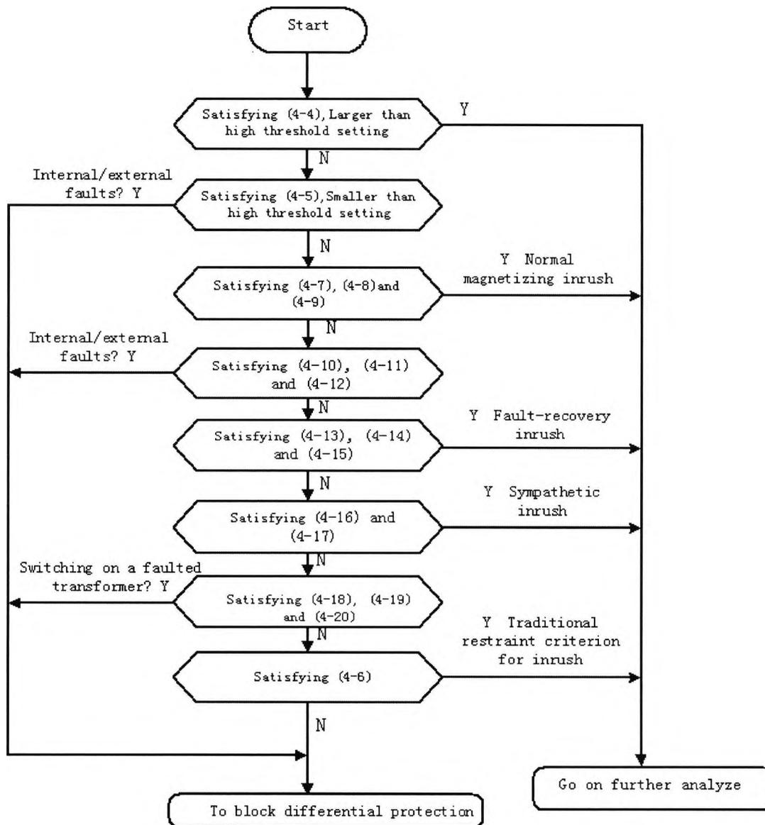
Fig 4.3 Flow chart of multi-condition inrush current restraint mechanism
