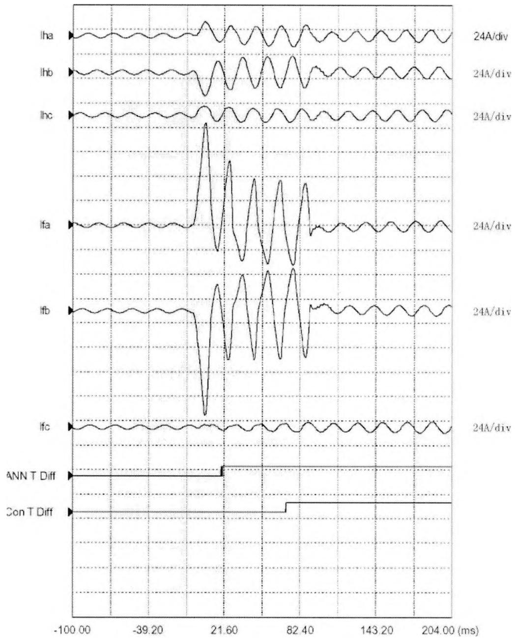
Fig 8.7 Transformer internal phase A to phase B short-circuit in low-voltage side
