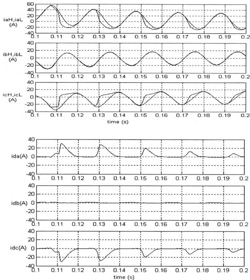
Fig. 6.3 Dynamic simulation test data of AB phase-to-phase fault on the high-voltage side
