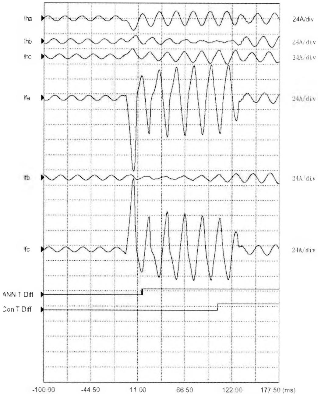
Fig 6.6 A phase A to phase C internal short-circuit occurred in low voltage side of transformer
