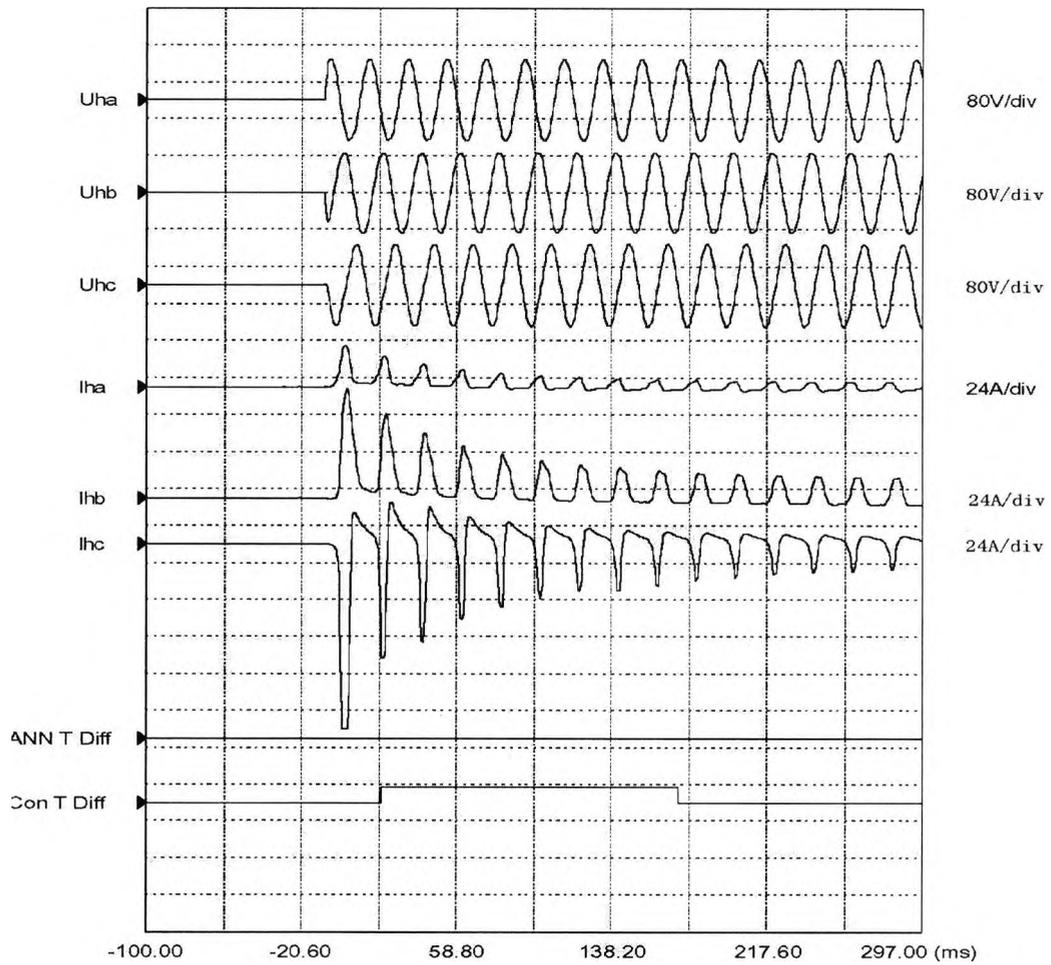
Fig 4.4 Transformer inrush current when switching on
