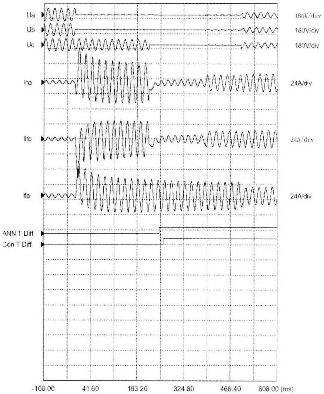
Fig 8.10 A phase A to phase B to ground transferred to transformer internal three-phase fault
