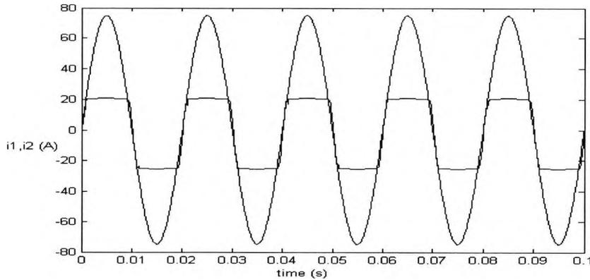
Fig. 6.1(c) CT steady-state saturation under inductance current excitation condition
