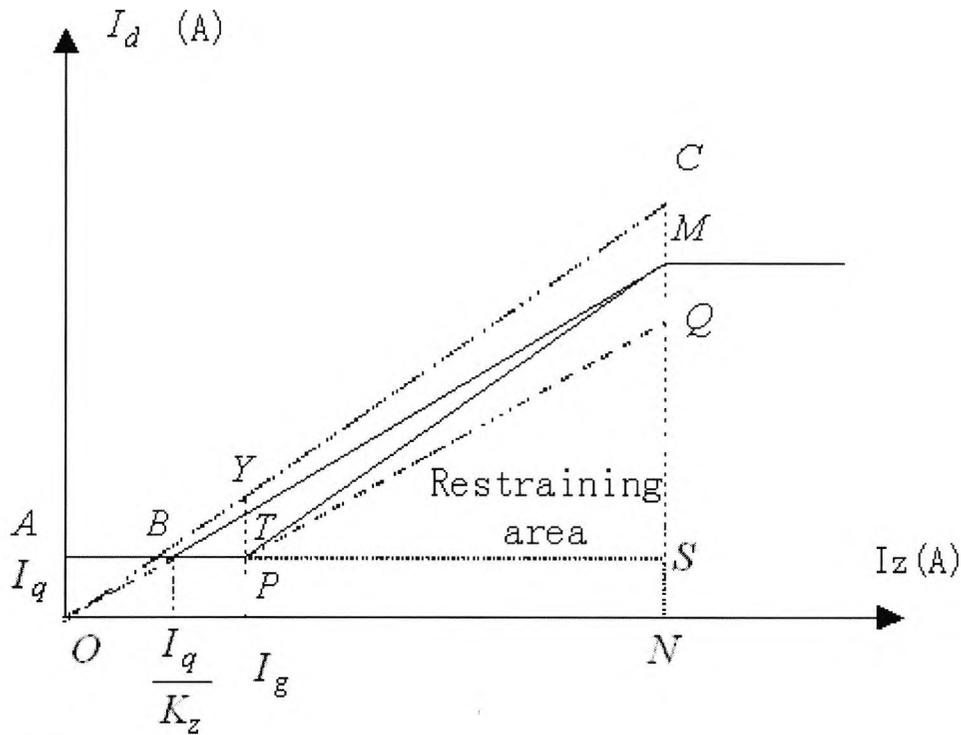
Fig. 8.2 The corresponding relation of the restraint coefficient and the slope
