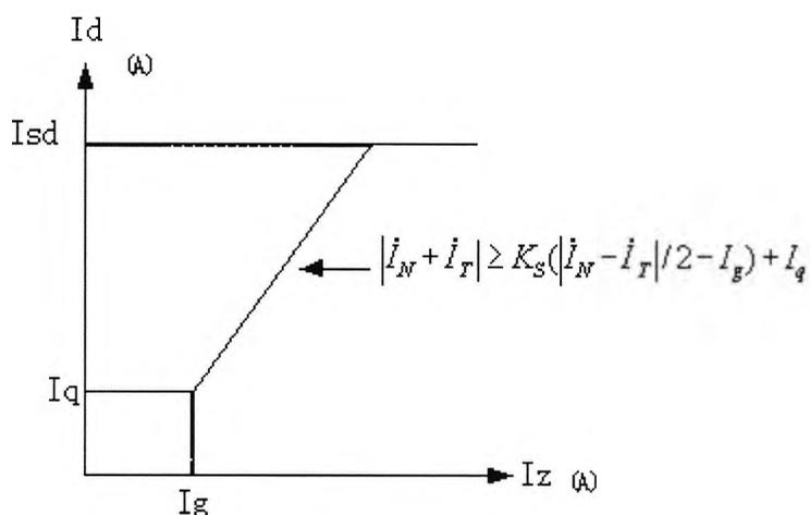
Fig. 2.1 The ratio restraint characteristic curve (not passing through the origin)
