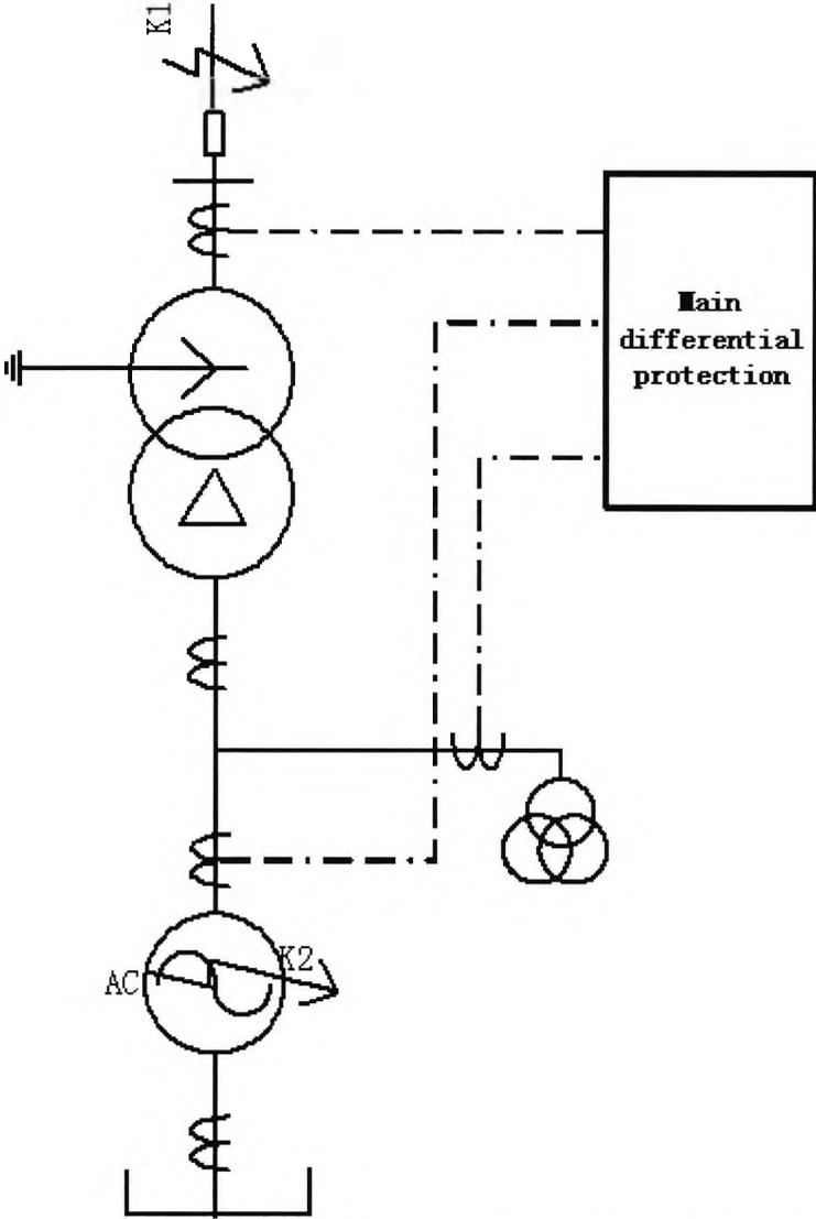
K1: System side fault point; K2: Generator side fault point
