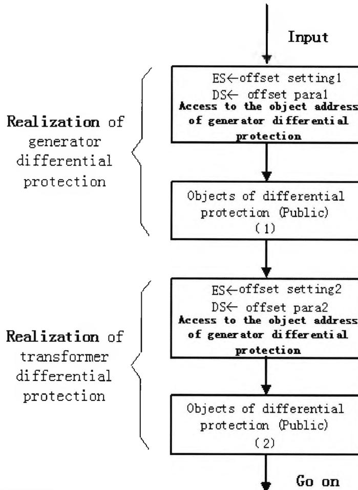
Fig. 9.7 Simplified realization framework of object oriented differential protection software
