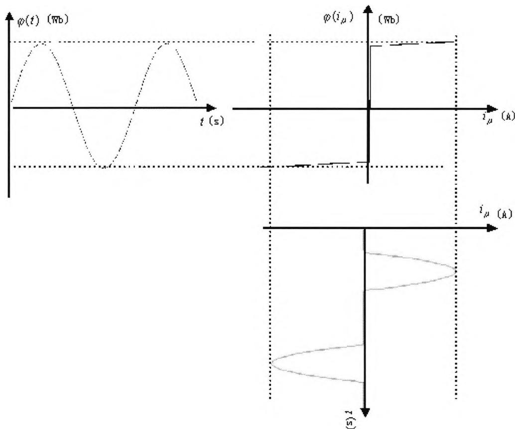
Fig. 4.2 Biased current during severe over-excitation of transformers
