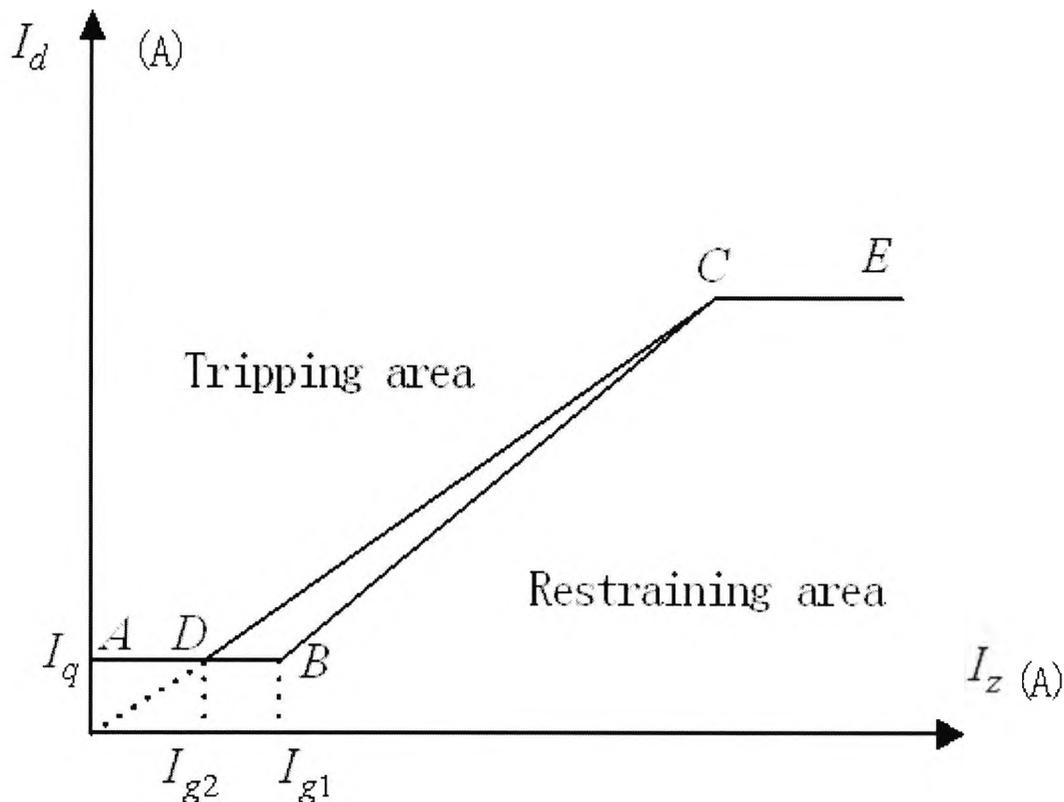
Fig. 8.1 The restraint curves passing the origin and not passing the origin
