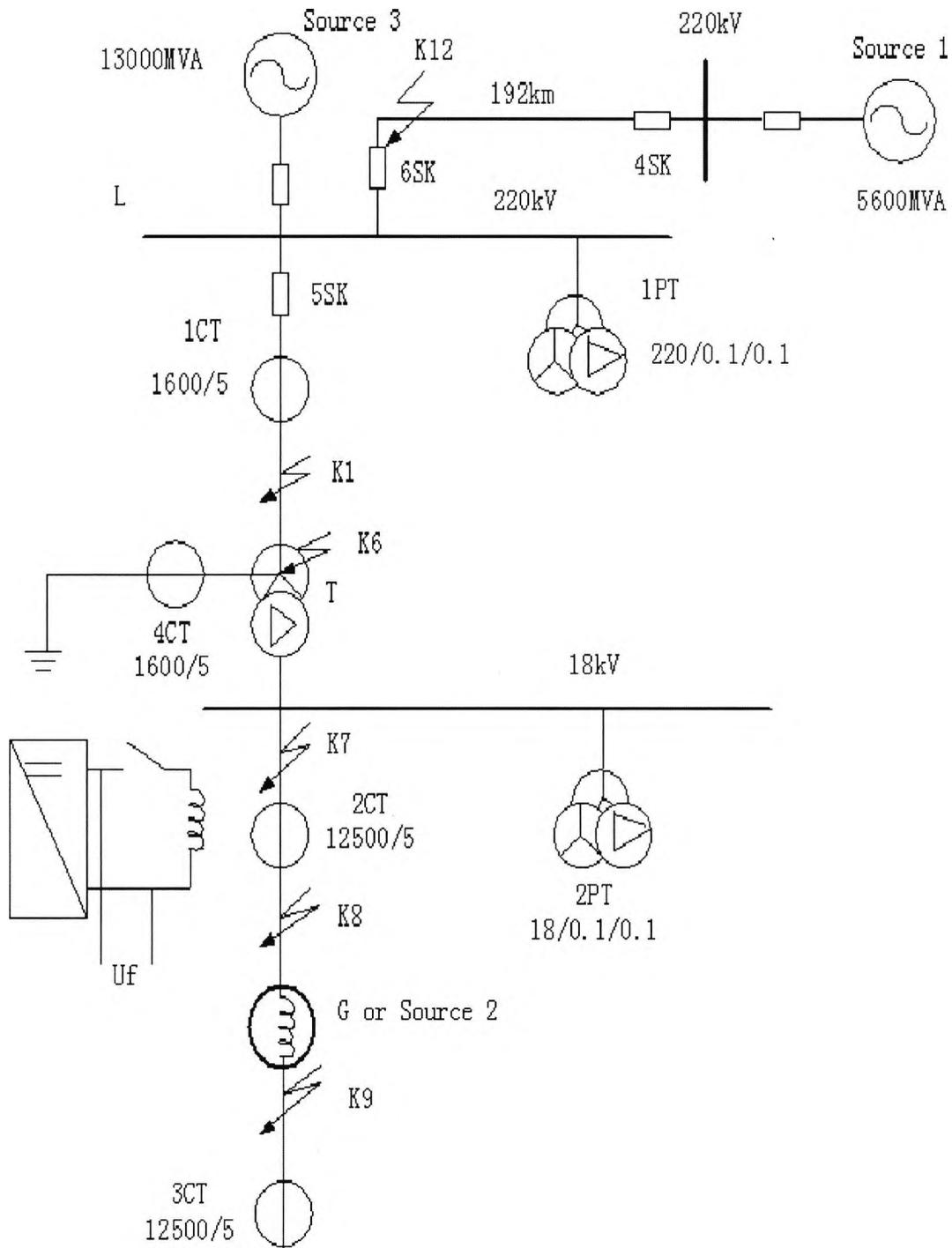
Fig.3.2 Simulation system module for generator and transformer protection test developed by EPRI
