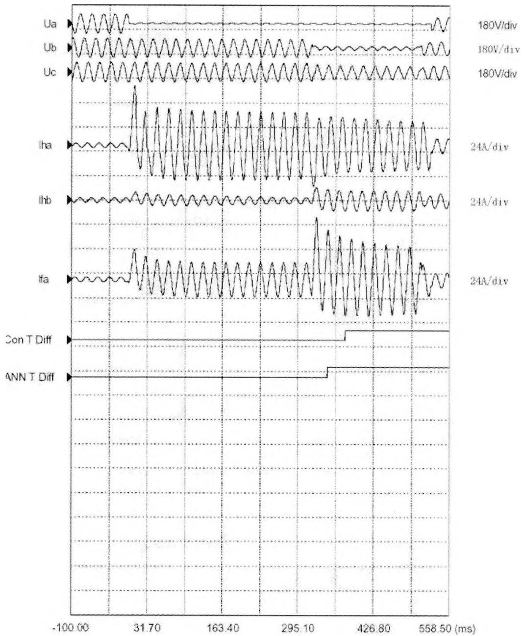
Fig 8.9 A phase A to ground line fault transferred to internal phase A to phase B short-circuit in low-voltage side
