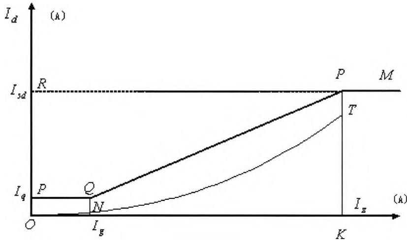
Fig. 6.1(b) Characteristic of differential protection based on ratio restraint
