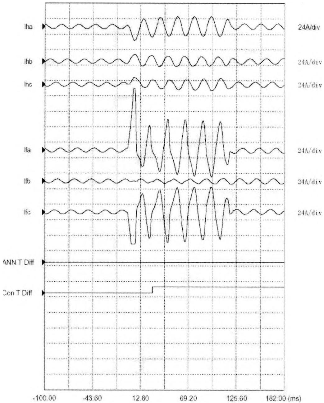
Fig 8.8 Transformer external phase A to phase C short-circuit in low-voltage side
