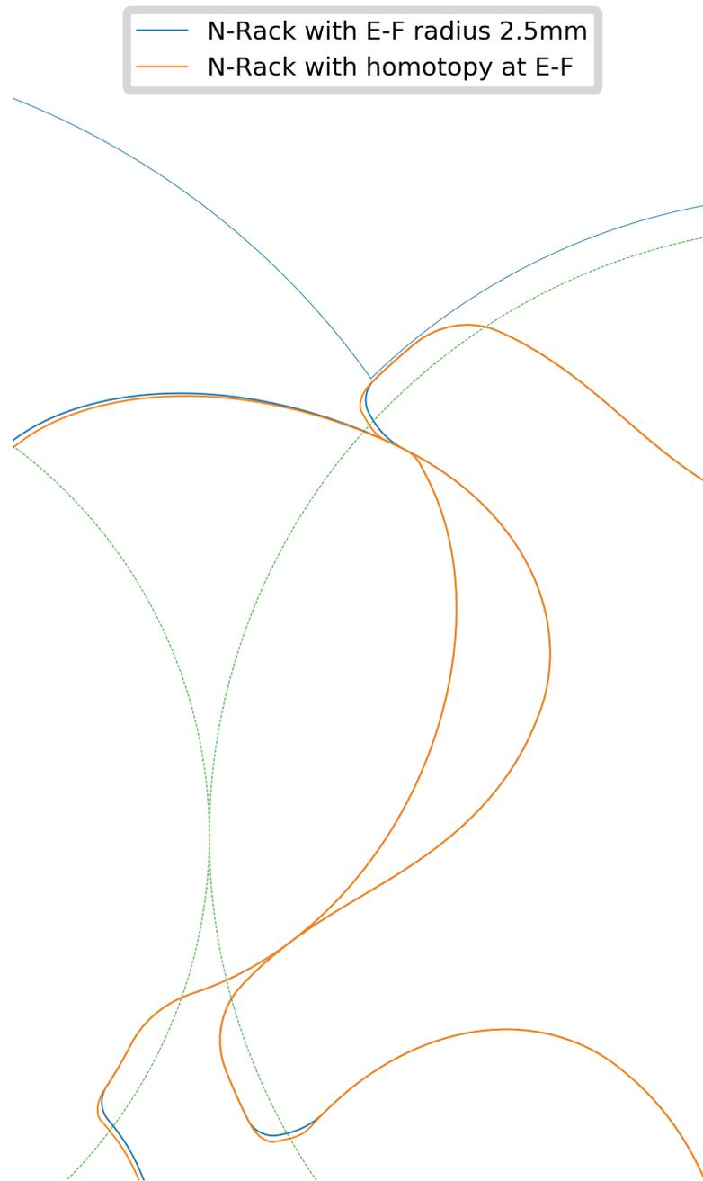
**Figure 4.10:** Profile generated with  $\mathcal{H}(\text{Ellipse}, \text{Line})$  at  $E - F$  retrofitted with the benchmark N-profile which has a circle of radius 2.5 mm at  $E - F$
