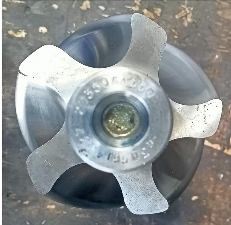
**Figure 5.14:** The K-BETA3 gate rotor manufactured at KPCL for testing
