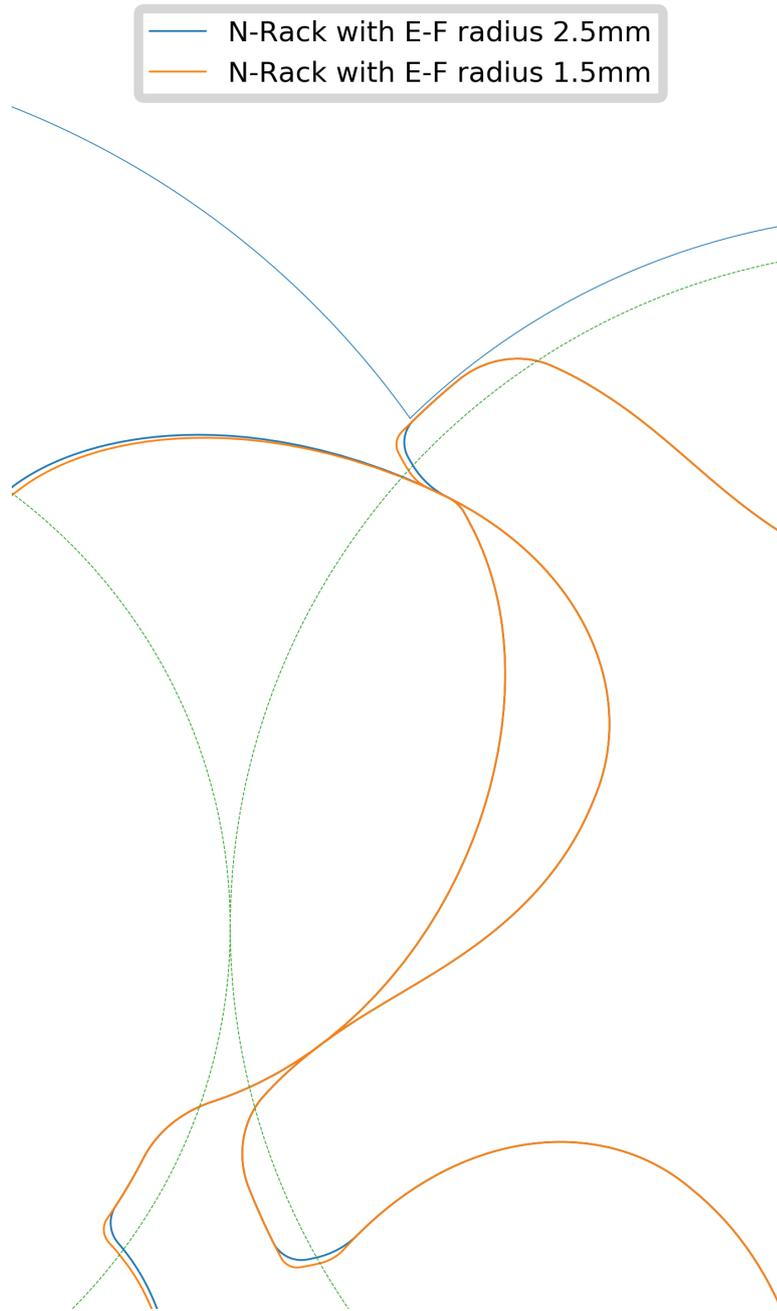
**Figure 4.7:** N-Profiles generated by N-Racks with tip radii for  $E - F$  as 2.5 mm and 1.5 mm
