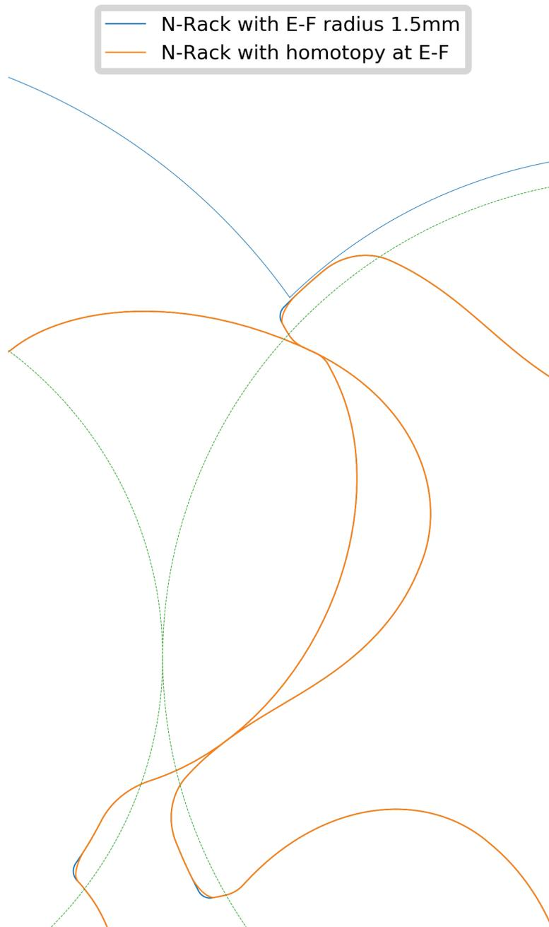
**Figure 4.11:** Profile generated with  $\mathcal{H}(\text{Ellipse}, \text{Line})$  at  $E - F$  retrofitted with benchmark N-profile if it had 1 mm smaller radius at  $E - F$
