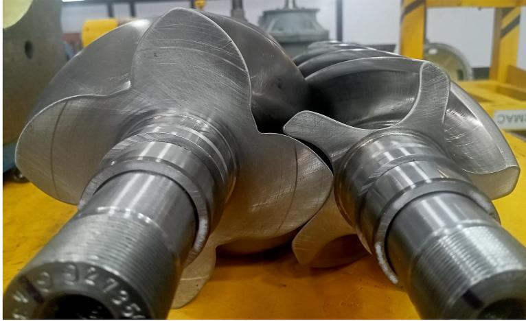
**Figure 5.7:** The 141 mm K-BETA1 rotors manufactured at KPCL for testing
