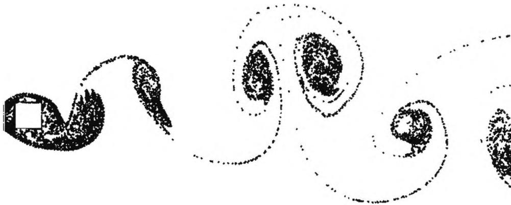
*Figure 5.45: Streaklines around a square cylinder at  $Re=4.2 \times 10^4$ .*
