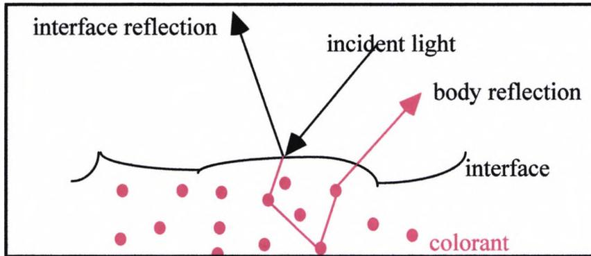
Figure 2.5 Reflected light from a dielectric material
