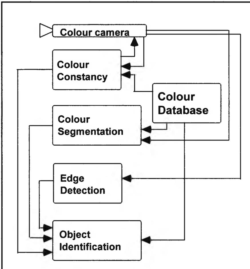
**Figure 1.0 Example of a colour machine vision system for object identification.**
