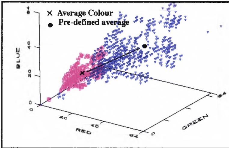
**Figure 5.6. The changes of observed colours in the colour space when the averaging colour constancy algorithm is applied.**
