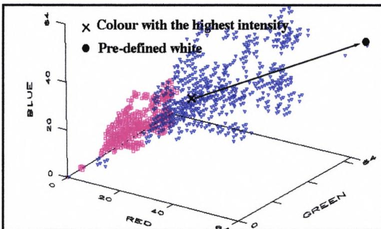
**Figure 5.7 The changes of observed colours in the colour space when the colour constancy algorithm with a predefined white is applied ( Under a transformation, the colour at location X will become the colour at location ●).**
