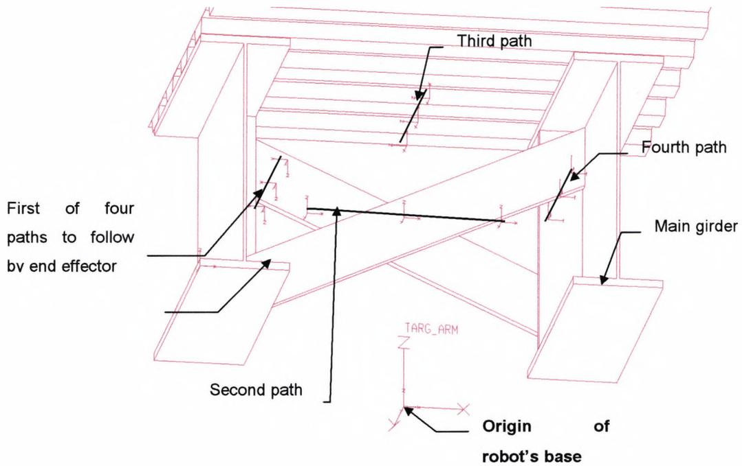
**Figure 4.3 Bridge Detail [A3] according to Table 4.3**
