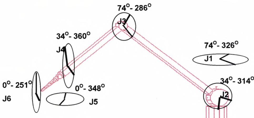
**Figure 10.8 Optimal Robot Selected for Extended Task (five paths)**
