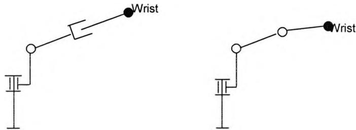
**Figure 7.3 Schematic Representations of RRP and RRR Configurations**
