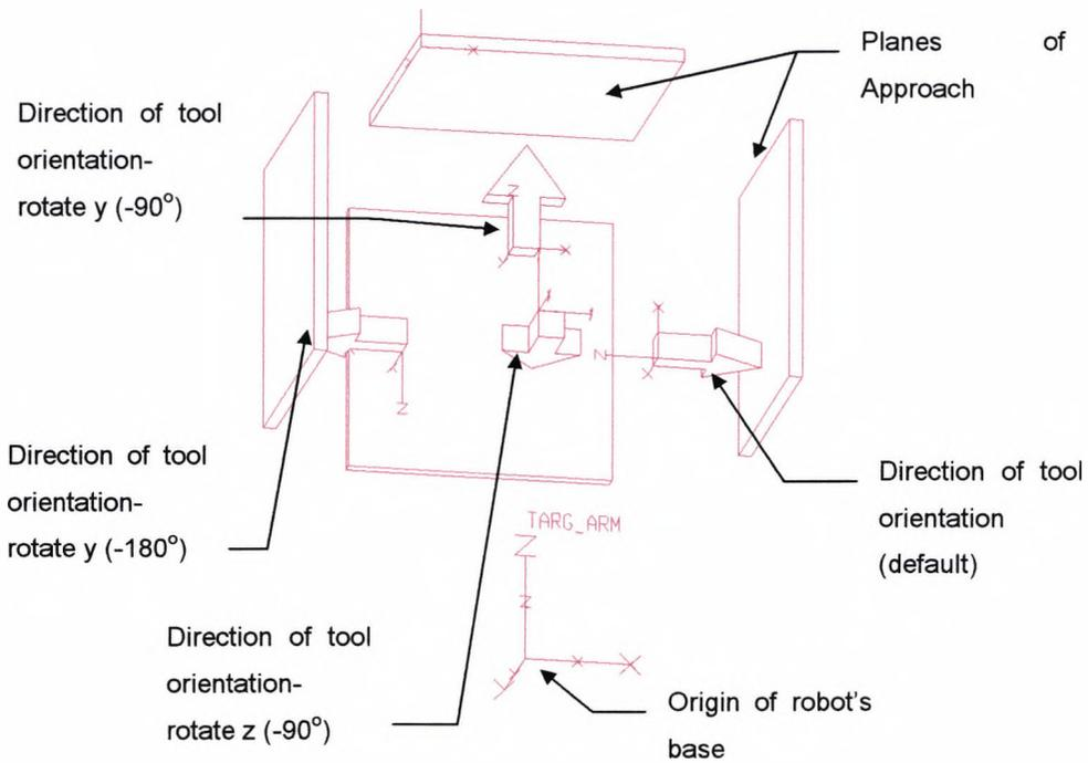
**Figure 4.16 Schematic Idealisation of Tool Orientation**
