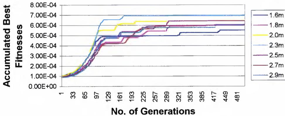
Figure 9.9 Accumulated Performance of MPIR for Variety of Reach in Different Size Workspaces
