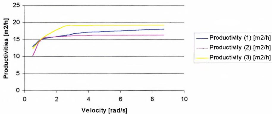
**Figure 9.10 Productivity of MPIR with 2.3m Reach for Varying Velocity Profiles**
