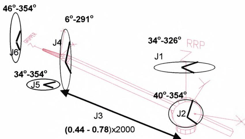
Figure 10.5 Optimal Robot Selected for Specified Initial Task (four paths)
