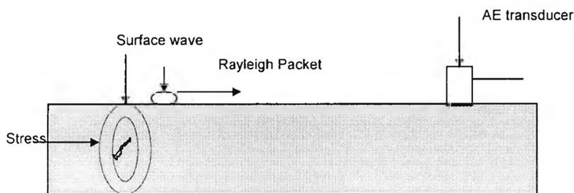
**Figure 5.4 Acoustic Emission Testing (AE)**
