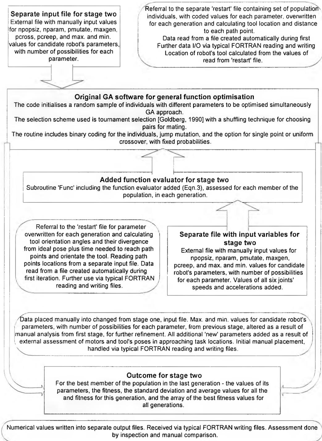
**Figure 8.5a and Figure 8.5b. Modules and their Roles, Function and Interaction for Stages One and Two**
