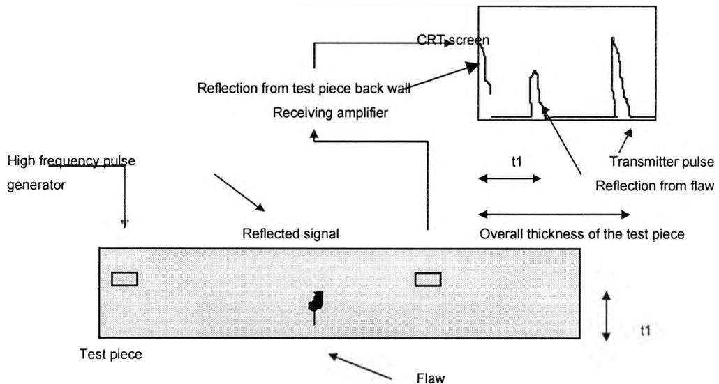
**Figure 5.2 Ultrasonic Testing (UT)**
