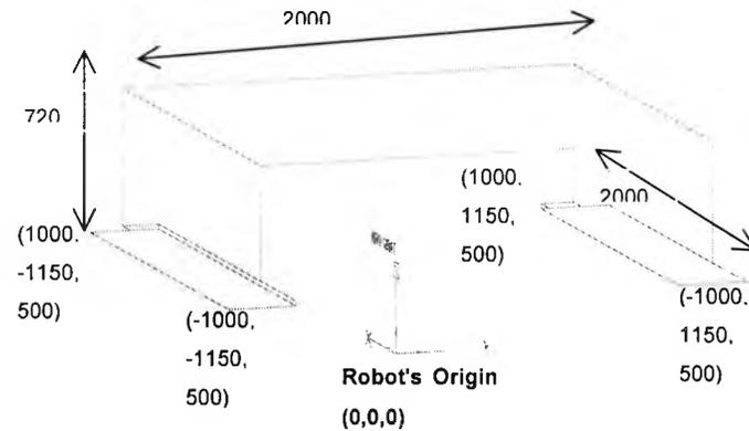
**Figure 8.1. Collision Envelope Isolated from the Unit Workpiece**
