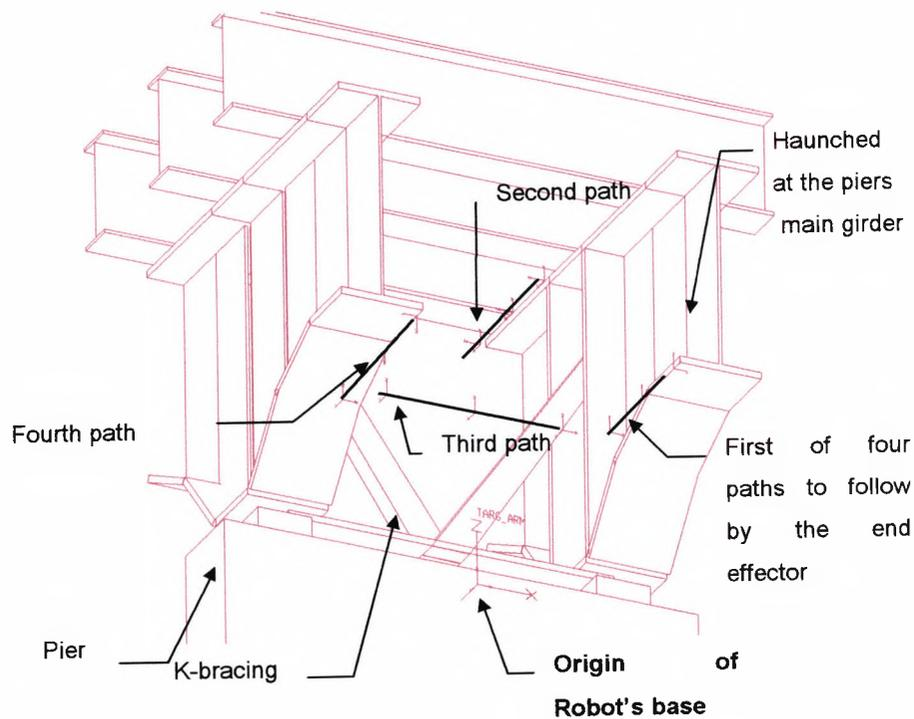
**Figure 4.8 Bridge Detail [C2] according to Table 4.3**
