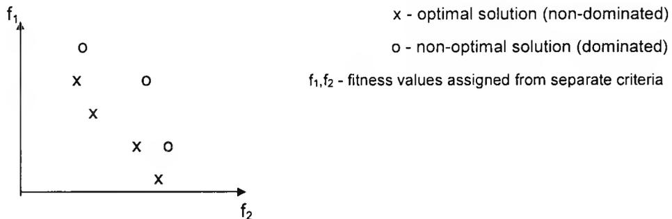
**Figure 8.4 Two-objective Function Showing Pareto Optimal Set**
