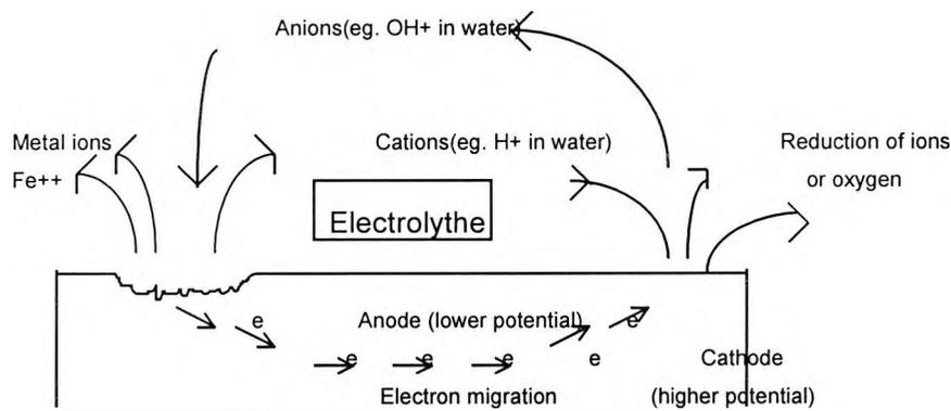
**Figure A.2 Simple Corrosion Cell**
