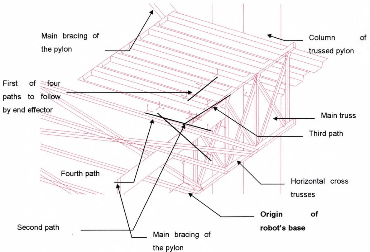
**Figure 4.4 Bridge detail [B1] according to Table 4.3**
