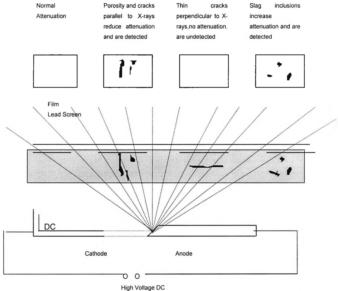
**Figure 5.1 X-Radiography Testing (RT)**
