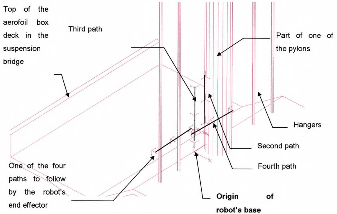
**Figure 4.15 Bridge Detail [E3] according to Table 4.3**
