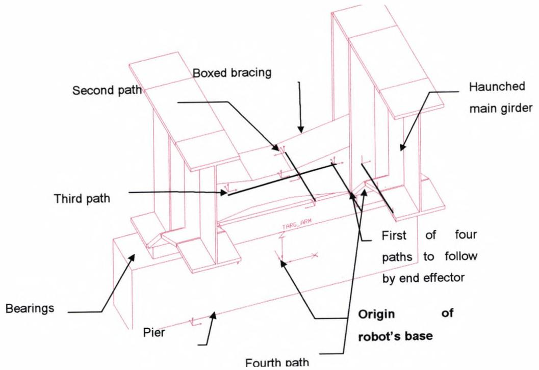
**Figure 4.9 Bridge Detail [C3] according to Table 4.3**
