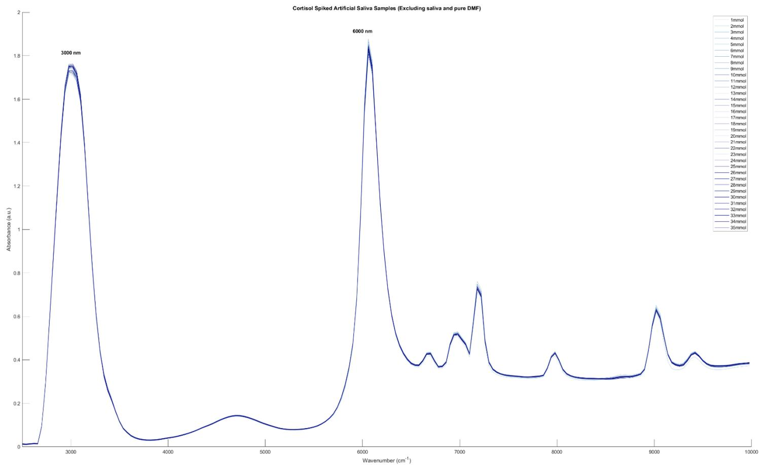
Figure 16 - Spectrogram of Cortisol-spiked saliva samples. Window size - 2500 -10,000nm. Including peak labels.
