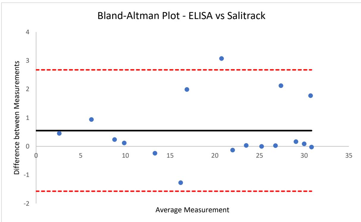
Figure 31b - Bland-Altman Plot for ELISA vs Salitrack Sensor. Showcasing average difference of 0.551ng/mL between concentration results obtained using the two methods.
