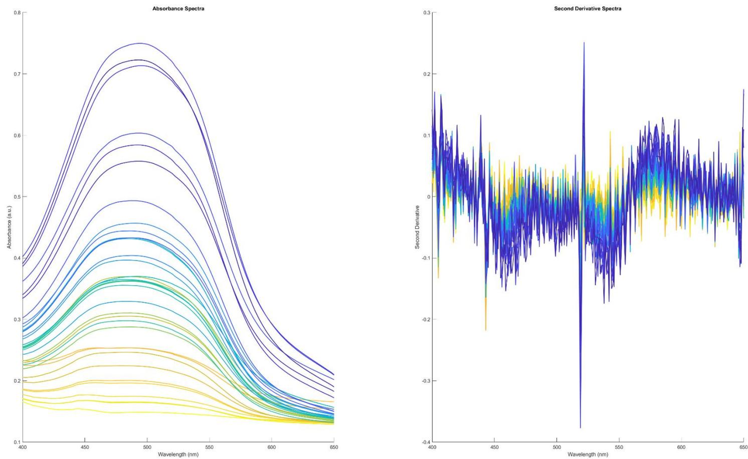
Figure 20 – Absorbance spectra of cortisol spiked saliva samples (left) with increasing colour intensity from yellow to blue showcasing increasing cortisol concentrations (left), 2nd order derivative transformation of cortisol-spiked artificial saliva samples(right) in the spectral range 400-650nm.
