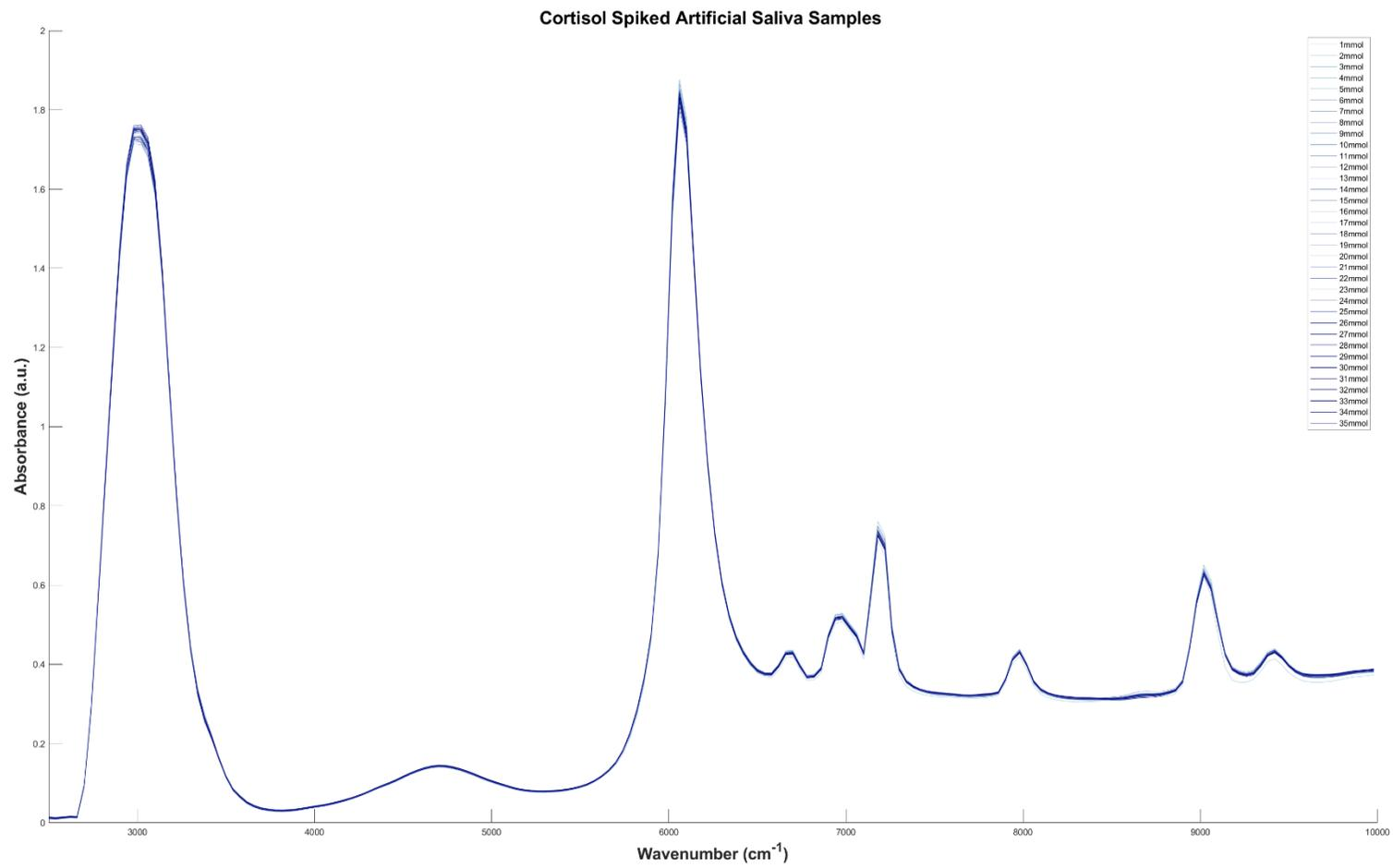
Figure 15 - Spectrogram of Cortisol-spiked saliva samples with increasing shades of blue representing increasing cortisol concentrations in artificial saliva samples. Window size - 2500-10,000nm.
