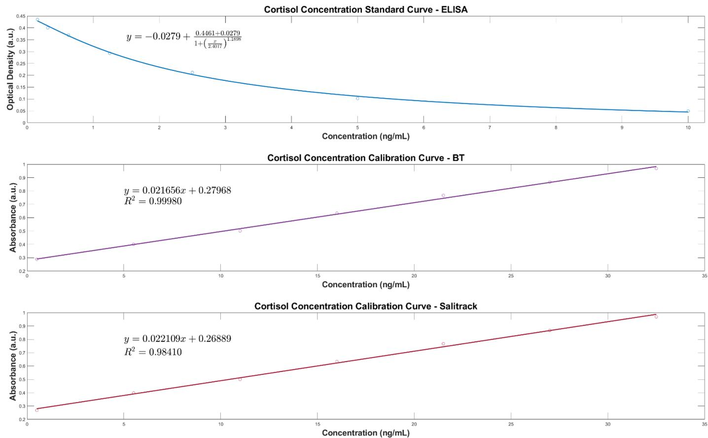
Figure 27 - Regression models for the analytical evaluation of artificial salivary cortisol in the clinical range (ng/mL) showing comparison between the gold standard ELISA protocol (Top), the Blue Tetrazolium (BT) method (Middle) and the prototype Salitrack colorimetric sensor (Bottom). The proposed BT method and prototype sensor show distinctive ability to determine cortisol in spiked artificial saliva samples.
