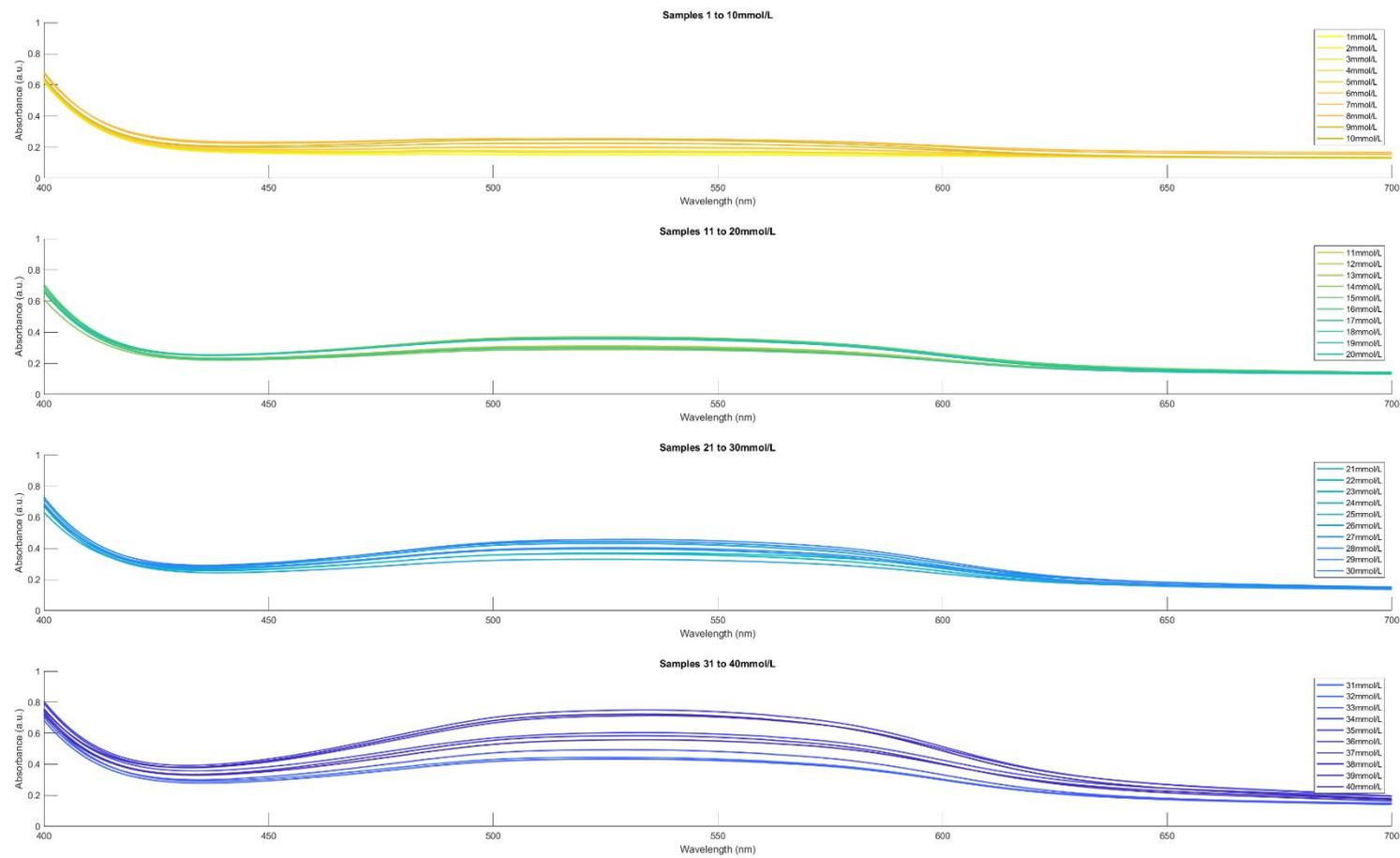
Figure 19 - Spectral visualisation of cortisol-spiked artificial saliva samples ranging from 1-40mmol/L in the spectral range 400-650nm.
