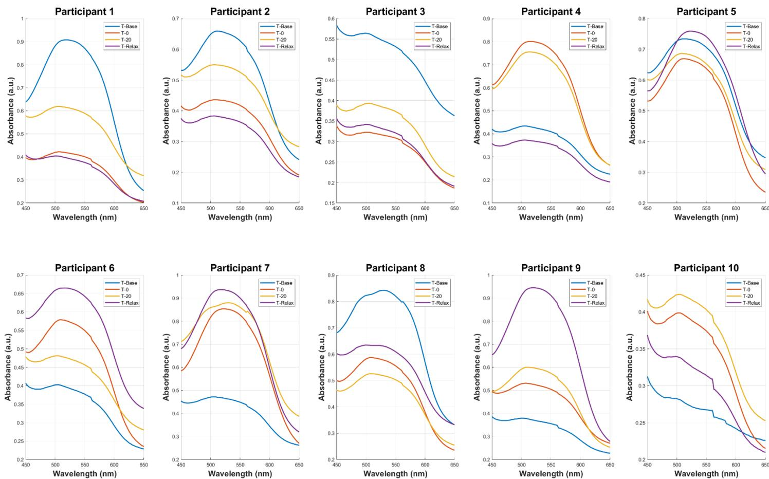
Figure 33– Absorbance spectra of cortisol in blue tetrazolium and tetramethylammonium hydroxide reagents with characteristic peak at 510nm, dataset 1 (Participants 1-10), including post-processing (averaging, baseline subtractions and Savitsky-Golay smoothing). Peak separation between varying concentrations shows clear distinction between detected cortisol concentrations.
