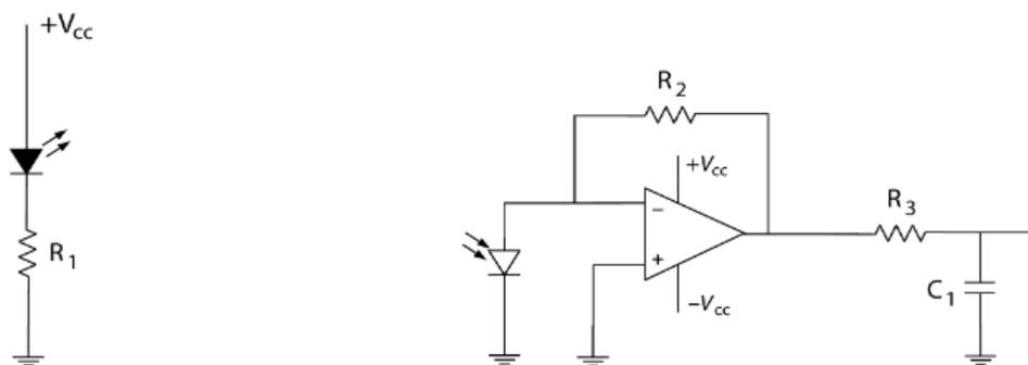
Figure 25 - Sensor circuit including LED and photodiode components for use as colorimeter.
