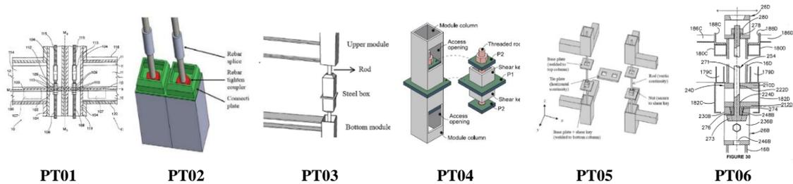
Figure 2. Post-tensioned IMCs
