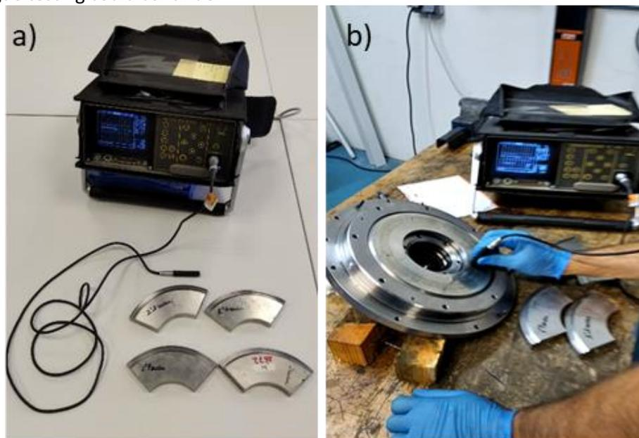
*Figure 5.13: (a): Eddy current equipment and antifriction material samples with different thickness to calibrate the equipment. (b): Inspection of the sensorised antifriction material specimen by eddy current technique.*
