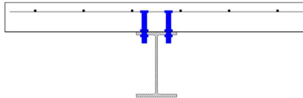
Figure 1. Demountable bolted
