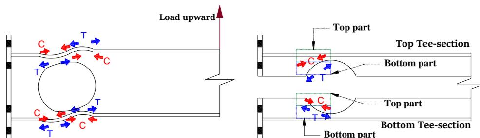
Figure 5. Illustration of the behaviour of Tee-sections.
