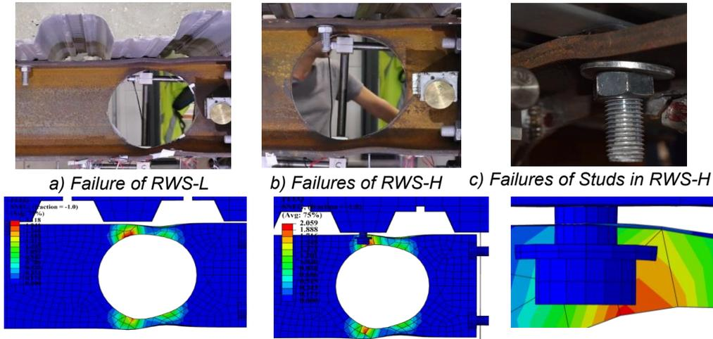
Fig. 3: Comparison between tests and FE models.
