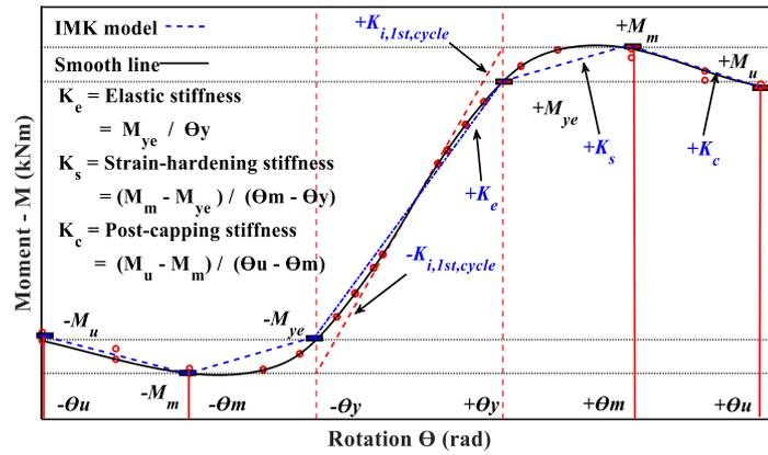
Fig. 4: Backbone curve for hysteretic models using IMK
