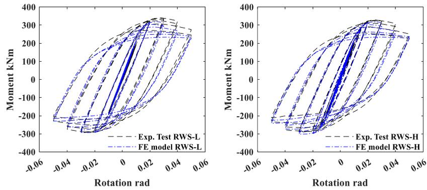
Fig. 2: Comparing between FE and experimental results.
