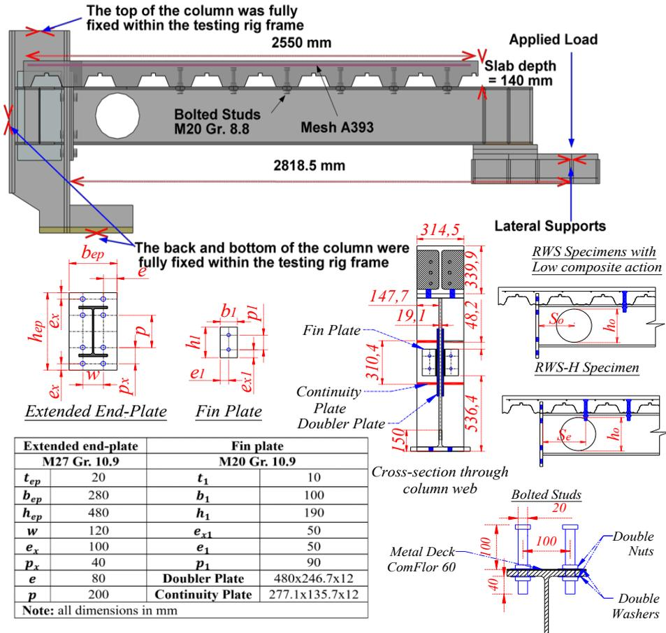
Fig. 1: Dimensions of test specimens (mm) [6].
