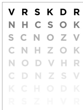
Figure 2.23: Pelli-Robson contrast sensitivity chart
