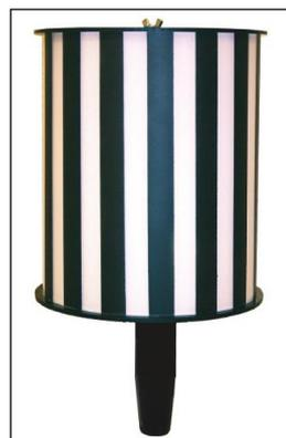
Figure 2.1: Optokinetic drum
