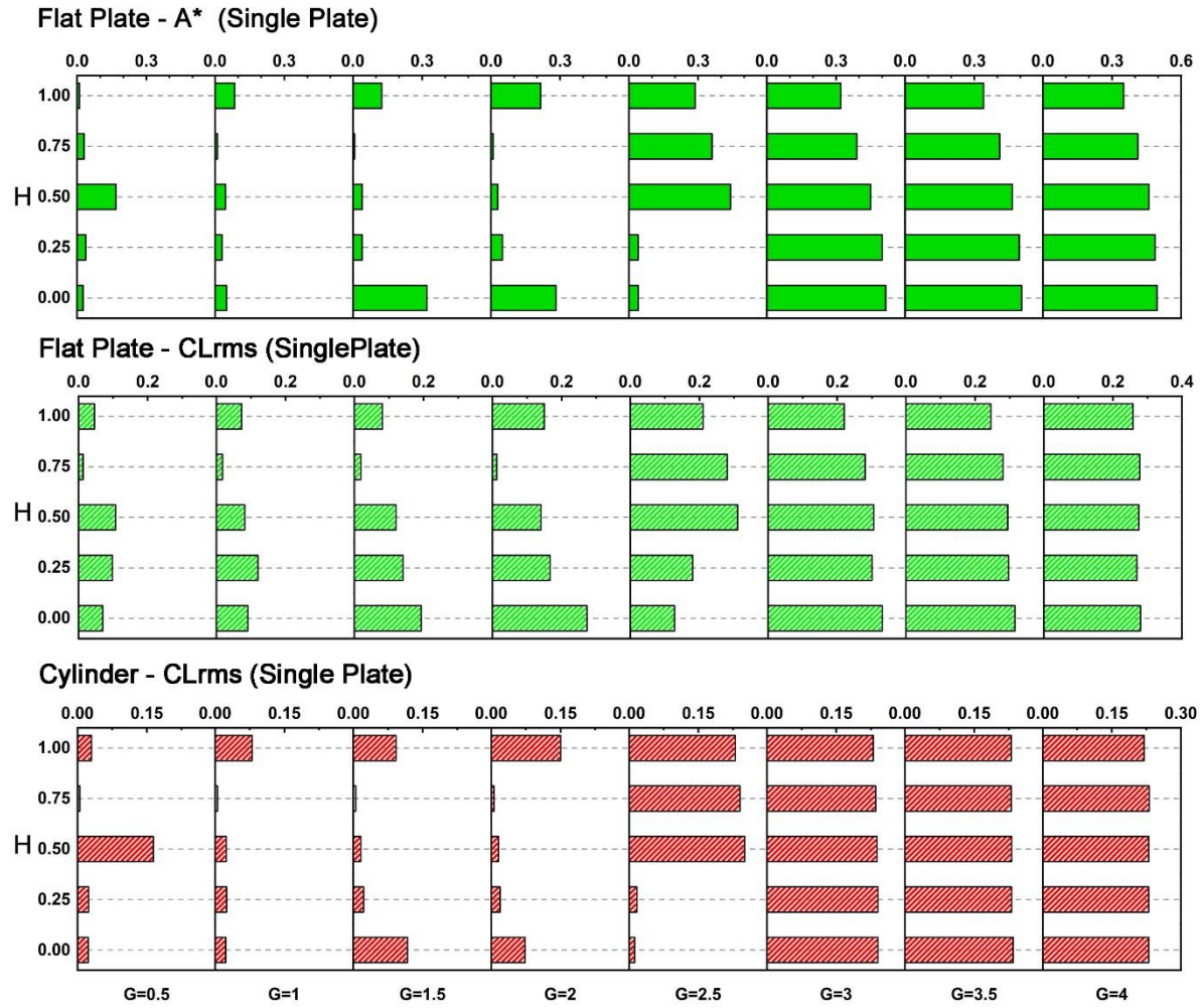
FIG. 5) Vibration amplitude and CL_{rms} of the single flat plate and the cylinder in different configurations at Ur=6
