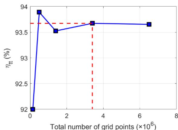
**Figure 4.** Mesh study of the first stage out of the 14-stage design. The blue line shows the efficiency variation with the number of grid points while the red dashed line highlights the selected mesh point for the study.
