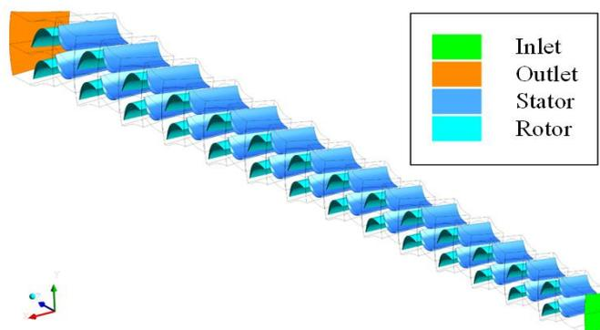
**Figure 3.** Numerical domain of the 14-stage design.
