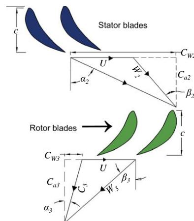
**Figure 1.** Geometry of a blade cross-section where  $C$  is the absolute velocity,  $W$  is the relative velocity,  $U$  is the blade linear speed,  $C_a$  is the absolute axial velocity,  $C_w$  is the absolute tangential velocity,  $\alpha$  is the absolute velocity angle and  $\beta$  is the relative velocity angle.
