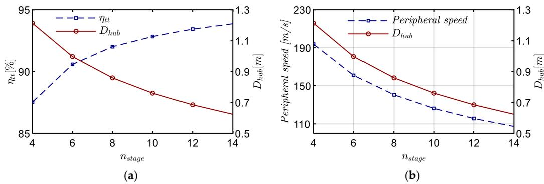
**Figure 7.** Effect of the number of stages ( $n_{st}$ ) on (a) the total-to-total efficiency ( $\eta_{tt}$ ) and hub diameter ( $D_{hub}$ ), and (b) peripheral speed for the CO<sub>2</sub>-SO<sub>2</sub> mixture as evaluated by the mean line loss model.
