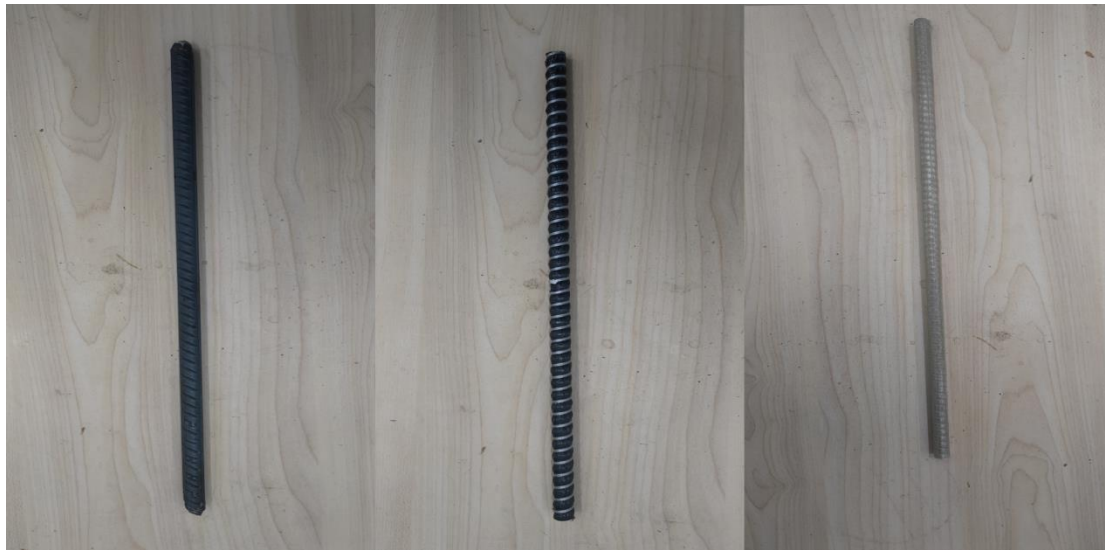
Figure 1. Reinforcement types Type. (a) Ordinary steel reinforcement (b)Carbon Fiber Reinforcement(c)Glass fiber reinforcement
