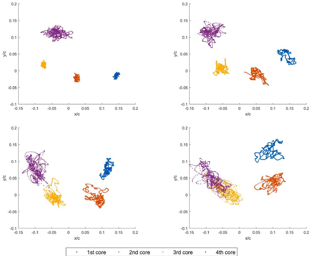
Fig. 8. Scatter plots of the instantaneous vortex core locations of the four strongest vortices in C-type configuration at  $Re = 90,000$ ,  $5^\circ$  AoA and 0, 0.5, 1 and 1.5 chords downstream respectively. (For interpretation of the references to colour in this figure legend, the reader is referred to the web version of this article.)
