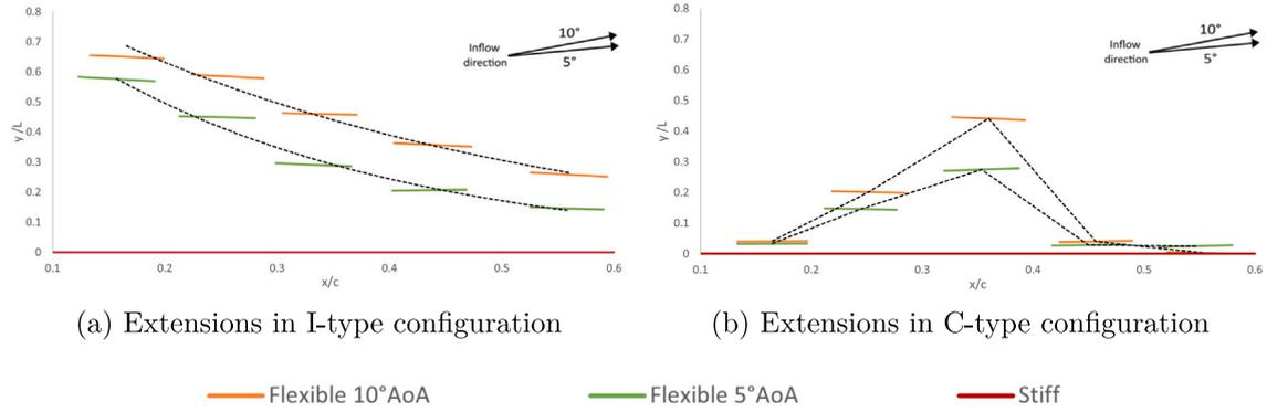
Fig. 6. Contours of the tips as seen from the lateral side relative to the pitched aerofoil, showing the upwards bending extensions and twist at  $Re = 70,000$ . (For interpretation of the references to colour in this figure legend, the reader is referred to the web version of this article.)
