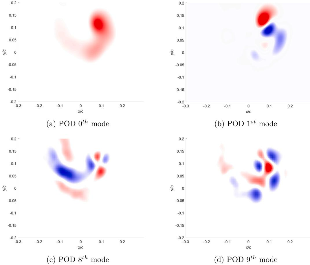
**Fig. 13.** Proper orthogonal decomposition modes at  $z/c = 1.0$  in the  $Re_c = 70,000$  and  $10^\circ$  AoA test. (For interpretation of the references to colour in this figure legend, the reader is referred to the web version of this article.)
