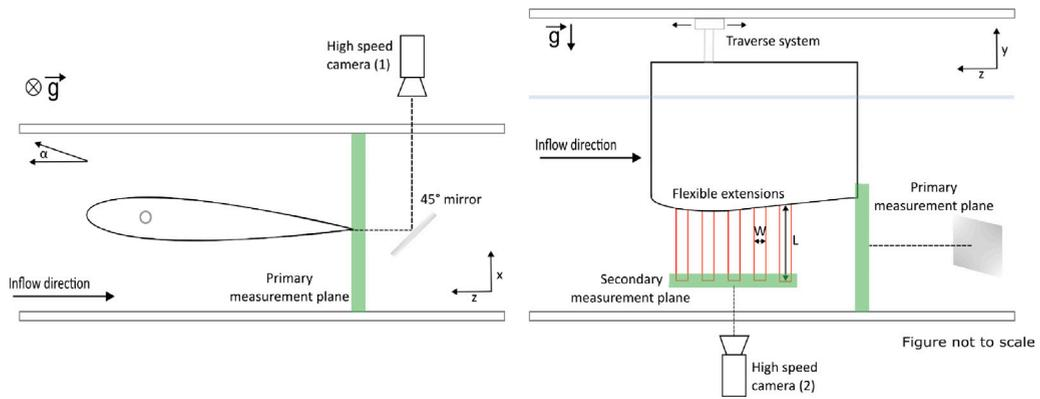
Fig. 4. Experimental setup (left: top-view, right: frontal view).
