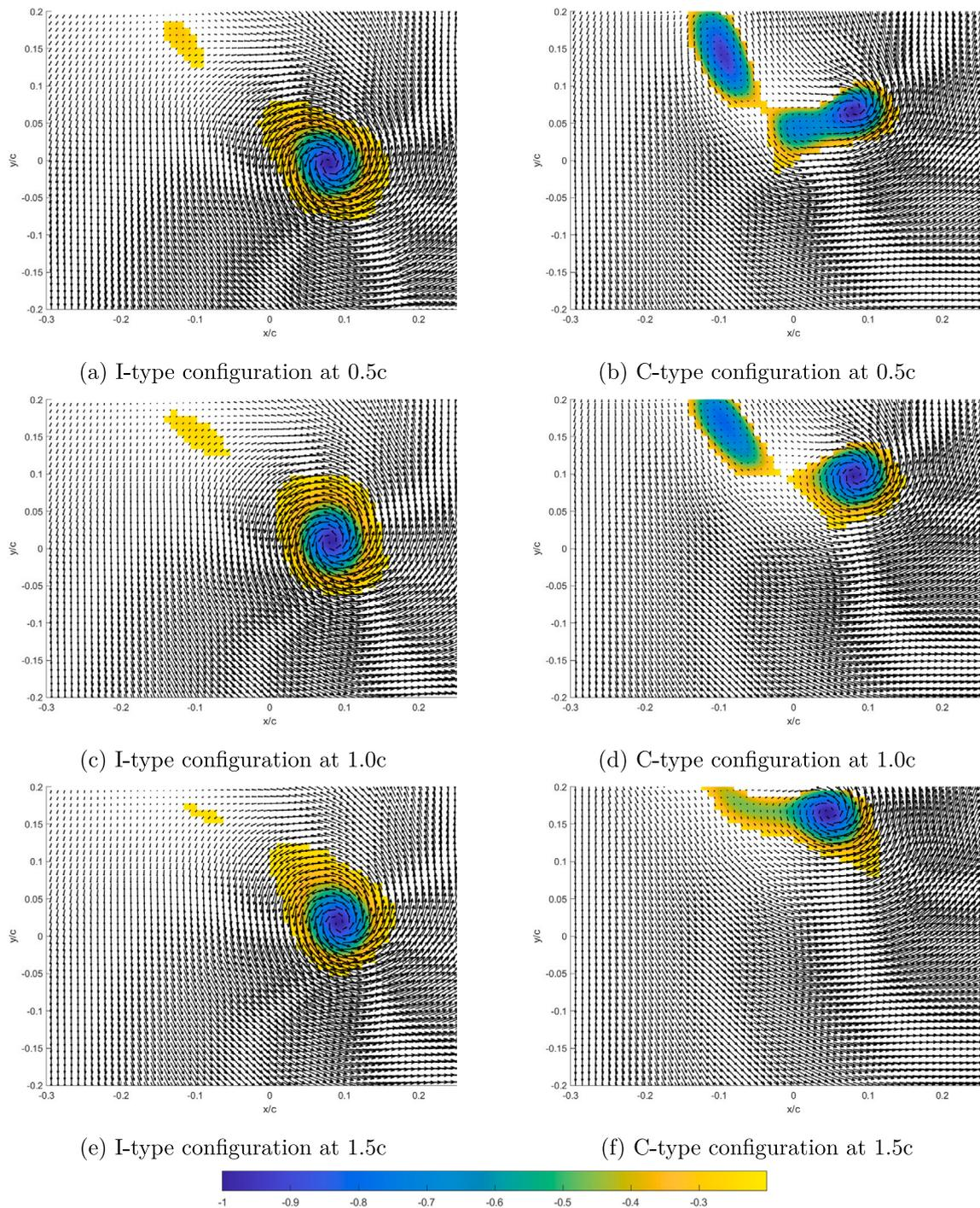
**Fig. 12.** Contours of lambda-2 criterion, in the fully deployed and bird-like configurations at  $Re = 70,000$  and  $10^\circ$  AoA. (For interpretation of the references to colour in this figure legend, the reader is referred to the web version of this article.)
