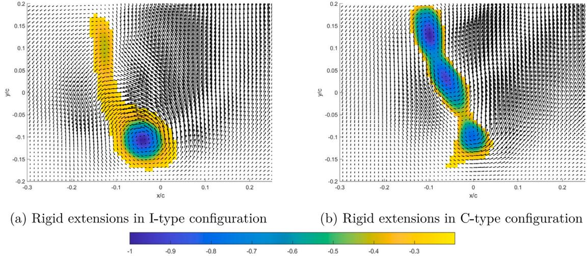
**Fig. 14.** Contours of lambda-2 criterion, 0 chords downstream at  $Re = 70,000$  and  $10^\circ$  AoA of the rigid extensions. (For interpretation of the references to colour in this figure legend, the reader is referred to the web version of this article.)
