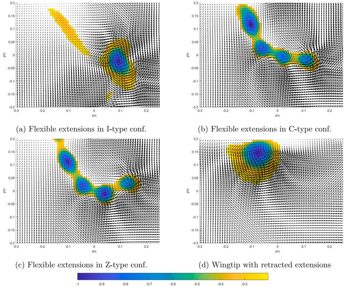
**Fig. 11.** Contours of lambda-2 criterion, 0 chords downstream at  $Re = 70,000$  and  $10^\circ$  AoA. (For interpretation of the references to colour in this figure legend, the reader is referred to the web version of this article.)
