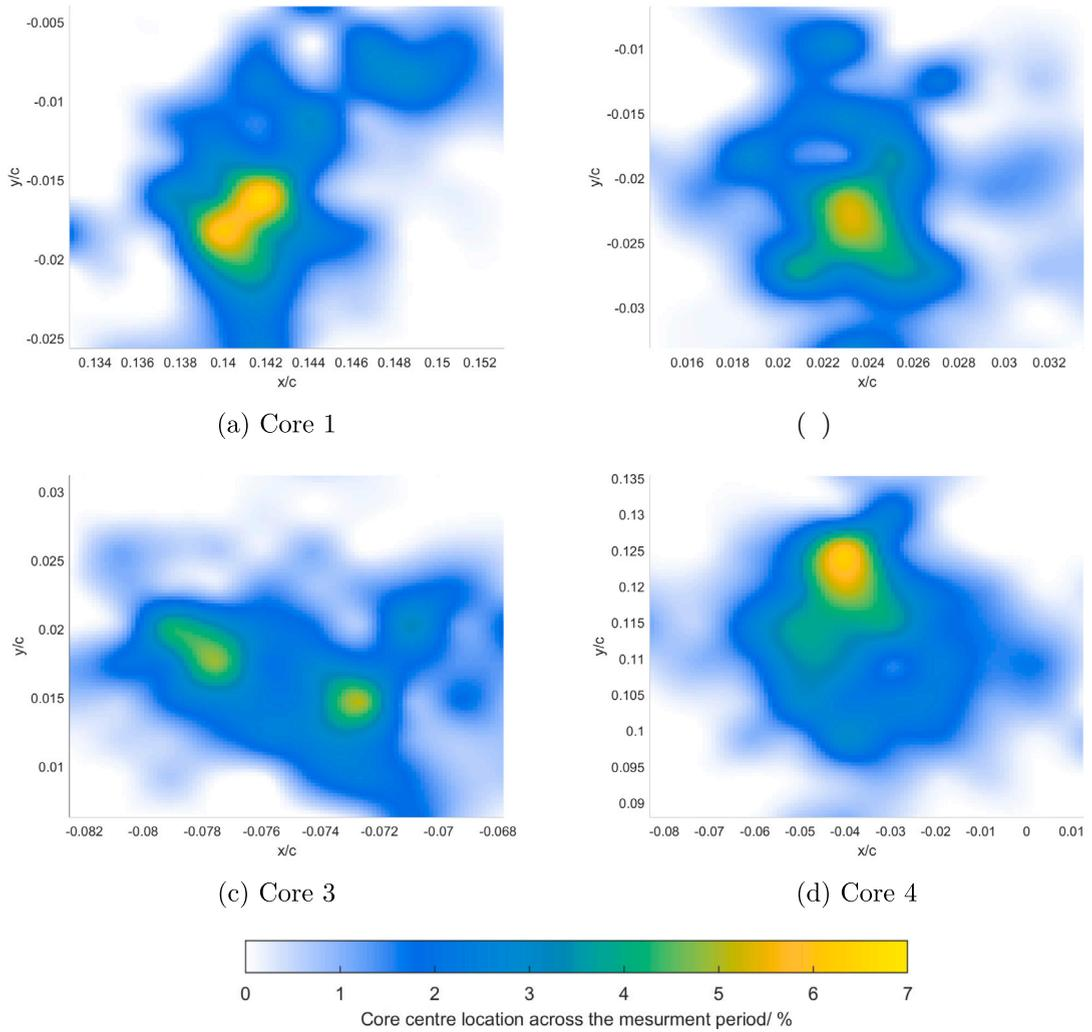
Fig. 15. Zoomed-in view, 2D probability density function of the x,y locations of the 4 strongest cores at  $Re_c = 90,000$  in the cross-sectional plane at a z-position of 0 chords downstream of the trailing edge. Note the physical area of each plot is not equivalent and is instead scaled to fit the range of core centre movement. (For interpretation of the references to colour in this figure legend, the reader is referred to the web version of this article.)
