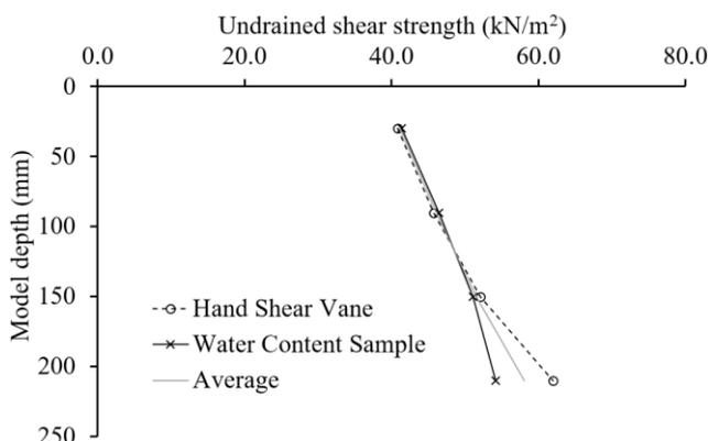
Figure 7: Model undrained shear strength profile with depth
