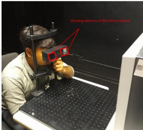
Figure 3.5: Figure shows the experimental set up for stereoacuity assessment. The subject is seated 50 cms from the screen, fixated at the random-dot pattern at the centre of the screen. The purpose of the stereo viewer (subject is holding at the spectacle plane) is to fuse the random-dot images perceived separately with each eye, with the help of prisms located inside the mirror.
